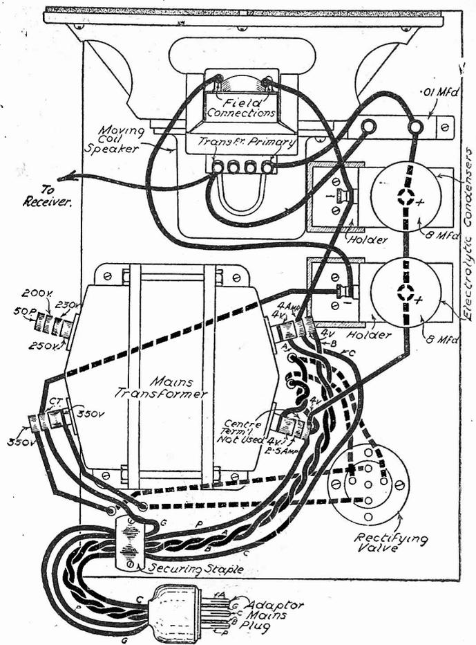
Fig. 3.—Wiring diagram of the mains unit used for the Luxor A.C. Superhet.
