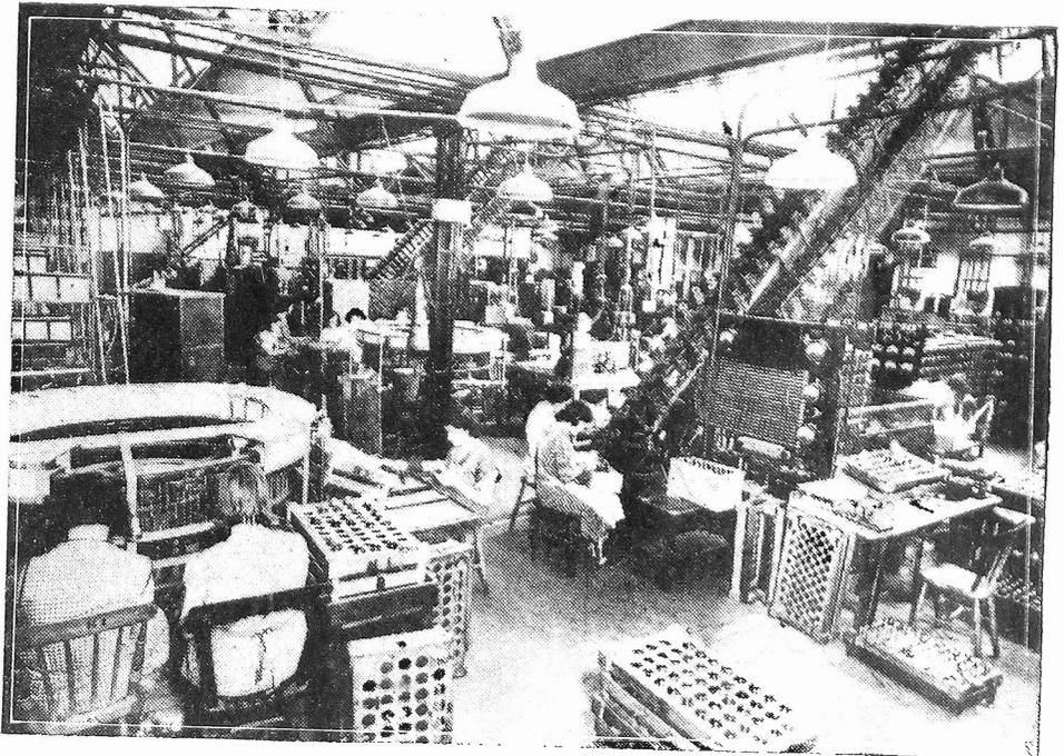
A corner of the battery-valve room in Messrs. A. C. Cossor's well-equipped factory, showing the conveyor.
