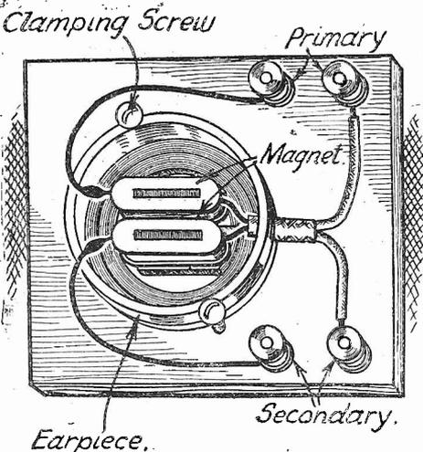
A small transformer made from an ear-phon.
