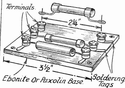
Fig. 4.—An easily made resistance-condenser unit by means of which the components can quickly be replaced.
