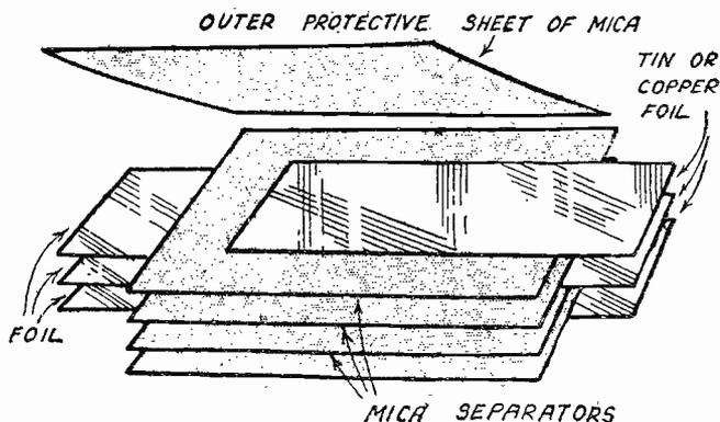
Fig. 4.—Showing how a fixed condenser is built up.
