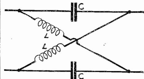
Fig. 6.—A circuit suitable for phase correction.
