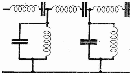
Fig. 4.—A modified circuit designed to give a band pass.
