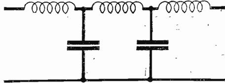
Fig. 3.—A low-pass inverse filter.
