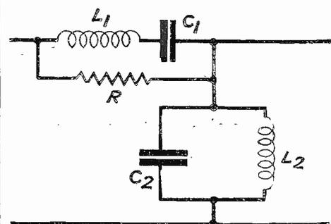
Fig. 5.—An inverted L-type circuit designed for equalization.
