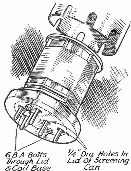
Fig. 2.—Showing how 3in. diameter screens can be fitted to standard 6-pin plug-in coil formers.
