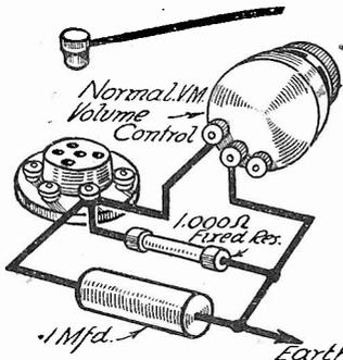
Fig. 4.—Volume control with a V.M. valve can often be improved, by connecting a fixed resistance in parallel with the volume-control potentiometer (used as a variable resistance). The reason is explained on this page.
