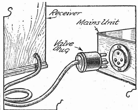
Fig. 2.—When the mains supply system is built as a separate unit, connection to it can be made by means of a valve plug and valve holder mounted as shown.
