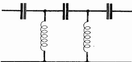
Fig. 2.—An ordinary two section T-filter.
