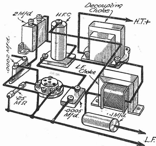
Fig. 1.—The circuit of a power-grid detector using choke capacity L.F. coupling and a choke for decoupling, as mentioned in the accompanying text.
