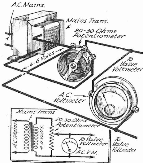
Fig. 5.—An alternative scheme, when an A.C. voltmeter is available.
