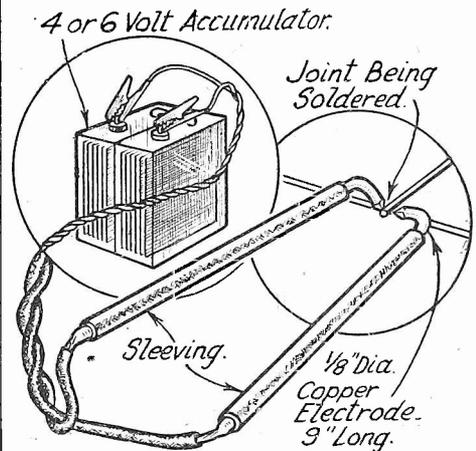
A novel method of soldering small work.
