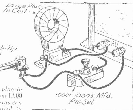
Fig. 6.—A plug-in coil of from 1,000 to 2,000 turns can often be used in series with a pre-set condenser as a pick-up scratch filter.
