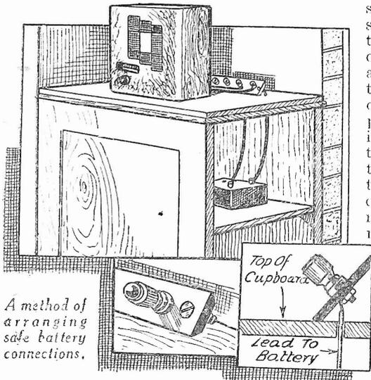
A method of arranging safe battery connections.
