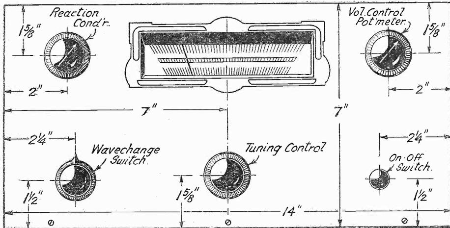
Fig. 2.—Front of panel layout.
