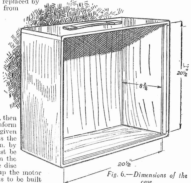
Fig. 6.—Dimensions of the case.
