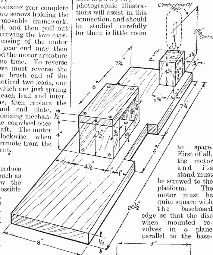
Fig. 9.—The wooden base and motor support.
