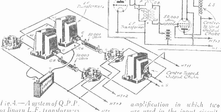
Fig. 4.—A system of Q.P.P. or ordinary L.F. transformers amplification in which two are used in the input circuit.
