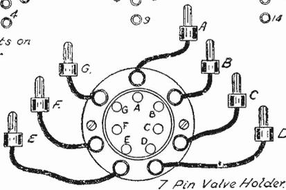
The connection for an additional valve-holder for testing Multi-pin valves on the Six-Sixty and similar test sets.
