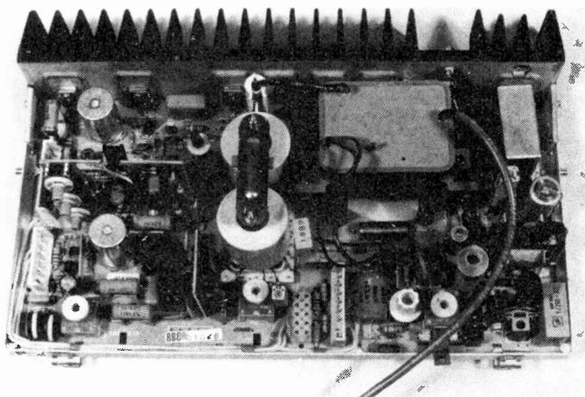
*The PC888 line and field output board. Note the massive heatsink and the test socket at the front, towards the centre.*
