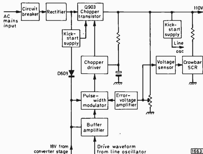
Fig. 4: Block diagram of the chopper supply circuit used in the Sony 13in. Models KV1300UB, KV1310UB and KV1330UB.
