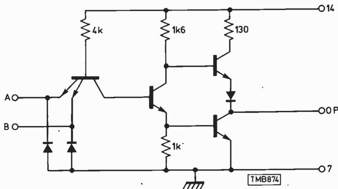
Fig. 1. Internal circuit of each of the four dual-input NAND gates of the 7400 i.c.s.
