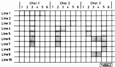
The above diagram shows a typical character format as seen on the screen. The process of character generation was explained on page 490 last month.
