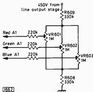
Fig. 3: C.R.T. first anode supply circuit, Sanyo Model CTP5101. The resistors at each side of the potentiometers are troublesome.
