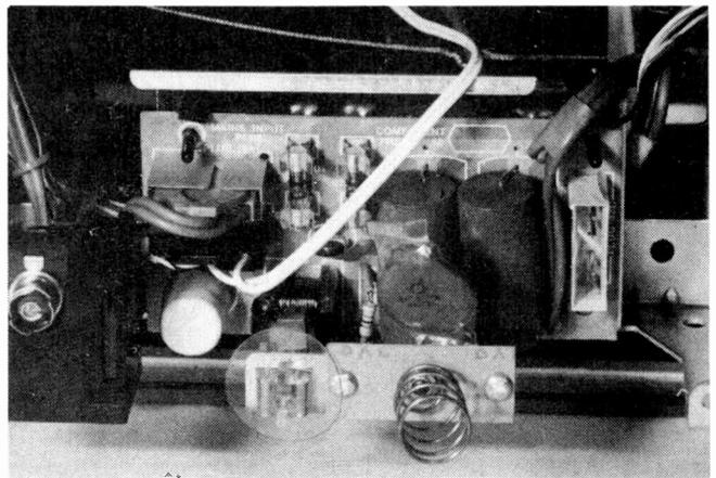
*The small mains panel is conveniently situated to enable the fuses to be quickly checked.*
