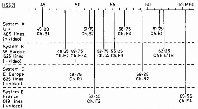
Fig. 1: Band I vision carrier frequencies used in Europe, excluding Eire and the UK B5 channel.
