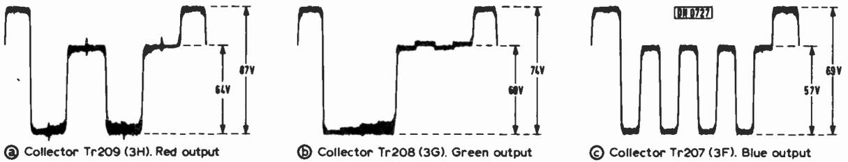
Fig. 2: RGB module waveforms.
