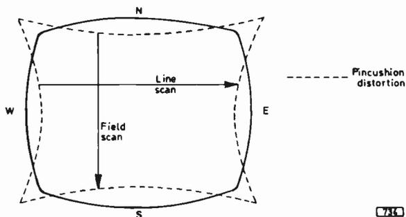
Fig. 5: Illustrating the pincushion distortion correction required.
