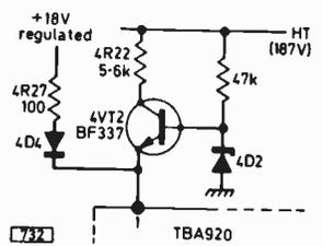
flows into it via 4VT14 base. As 4C74 charges so 4VT14 cuts off and the circuit then reverts to normal operation. On switching off 4C74 discharges via 4R108.
