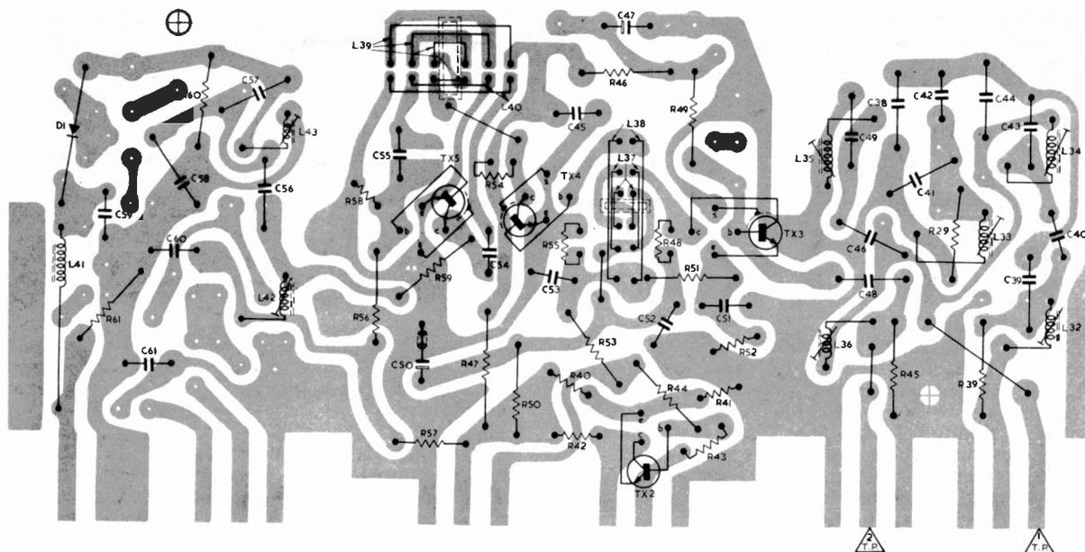
Fig. 2: Layout of the vision i.f. board—viewed from the print side.
