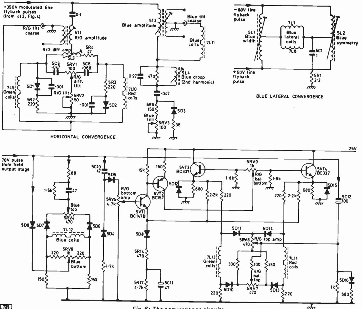
Fig. 6: The convergence circuits.
