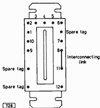
Fig. 3 (left): Tag connections to the line output transformer supplied by E. J. Papworth and Son Ltd. The  $-8V$  winding must be added—or see suggestion in column on right.
