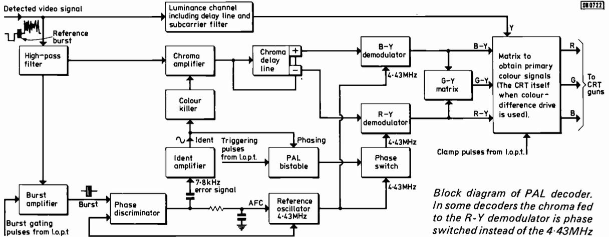
*Block diagram of PAL decoder. In some decoders the chroma fed to the R-Y demodulator is phase switched instead of the 4.43MHz reference supply.*
