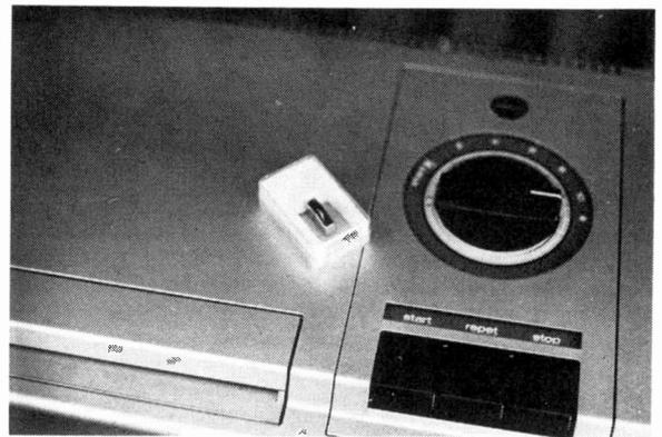
*This exclusive "Television" photograph shows a close-up view of the TED player with the pick-up cartridge in its box on top.*
