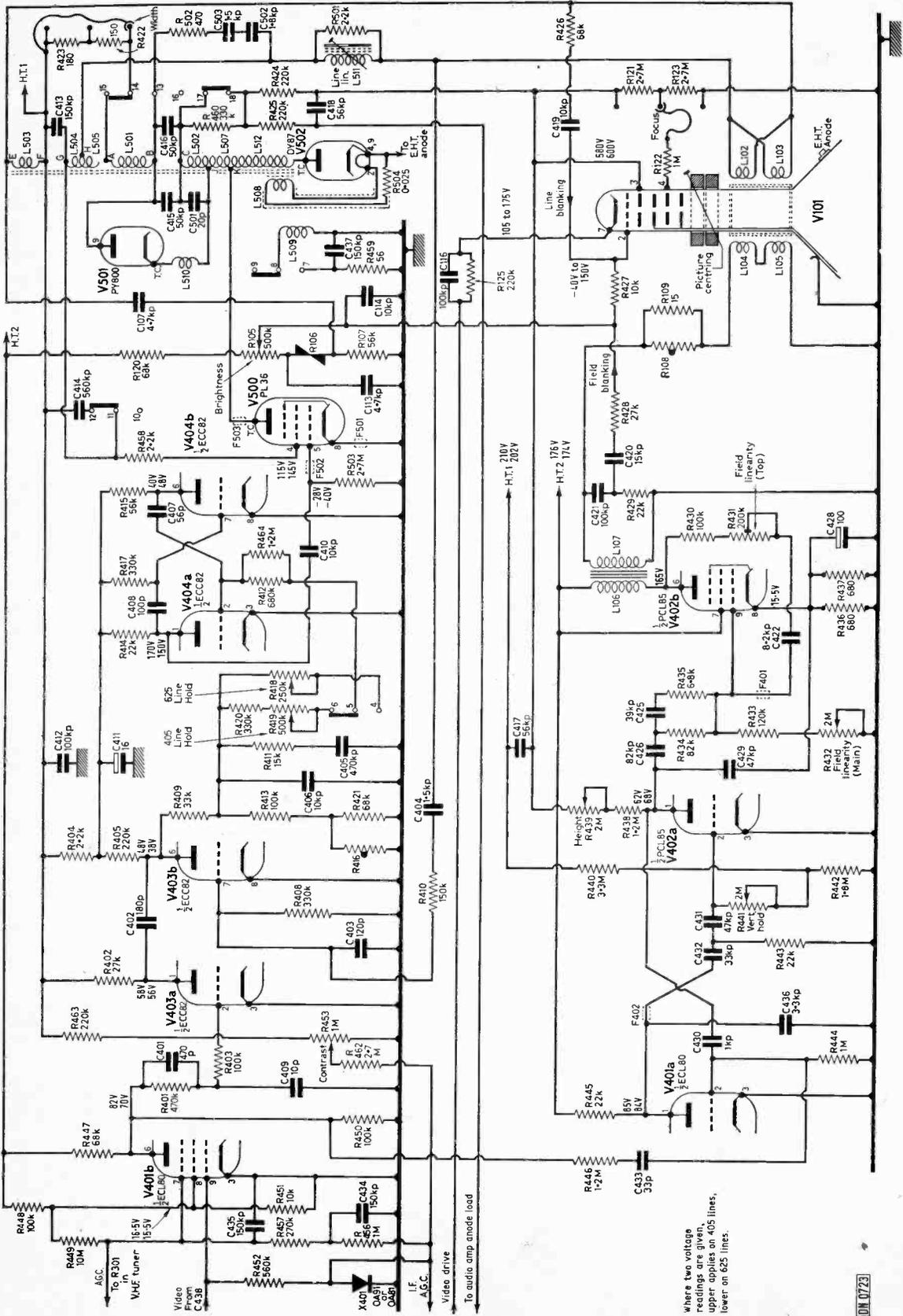
Where two voltage readings are given, upper applies on 405 lines, lower on 625 lines.
