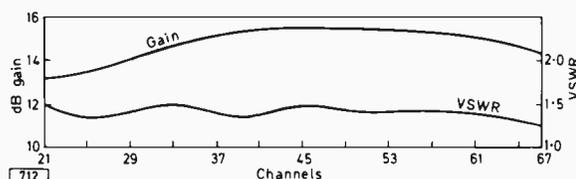
Fig. 1: Gain and VSWR characteristics of the Wolsey "Colour King" wideband u.h.f. aerial.
