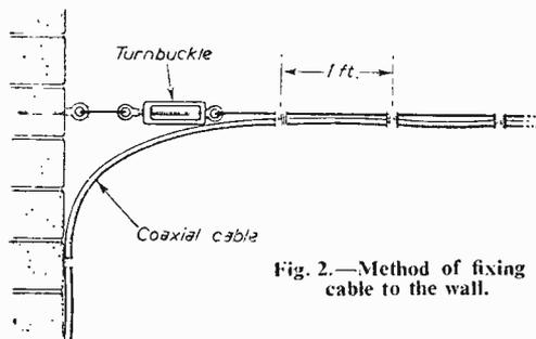
Fig. 2.—Method of fixing cable to the wall.
