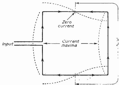
Fig. 2.—Current distribution around the loop.
