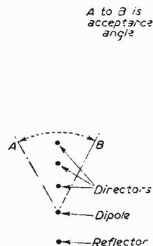
Fig. 3.—Showing the narrow acceptance angle of a five element array.
