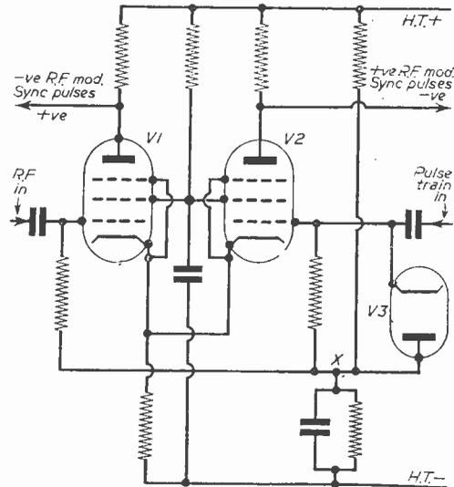
Fig. 10.—Pulse mixing stage.
