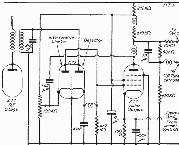
Fig. 3.—A circuit of a typical detector and video output stage modulating tube cathode.
