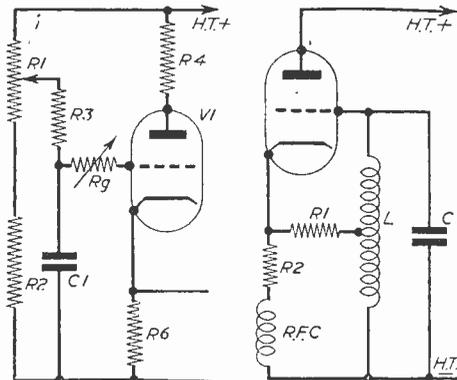
Fig. 6. (Left).—Modified Fig. 2, to give variable fly-back time. Fig. 7. (Right).—R.F. oscillator for vertical bar generation (see previous article).
