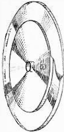
Fig. 52. — A prismatic disc, as used in an American System.
