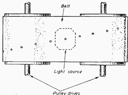
Fig. 54. — Scanning obtained by means of a perforated belt.
