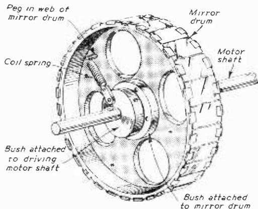
Fig. 51. — A complete mirror drum, showing the method of clipping on the mirrors.
