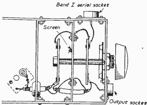
Fig. 3.—Switch installed in converter.
