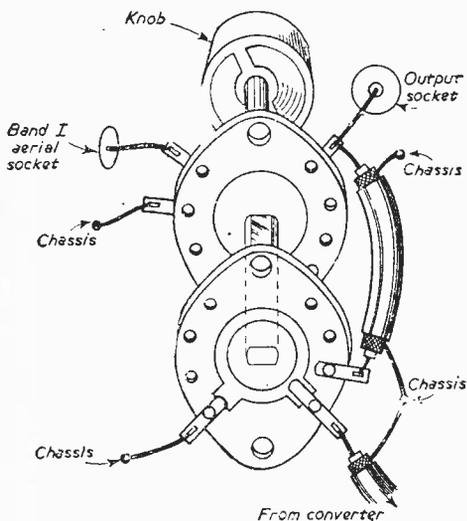
Fig. 1.—Switch in Band 1 position.
