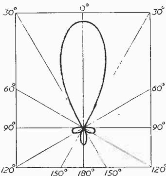
Fig. 1.—Polar diagram of Yagi array.
