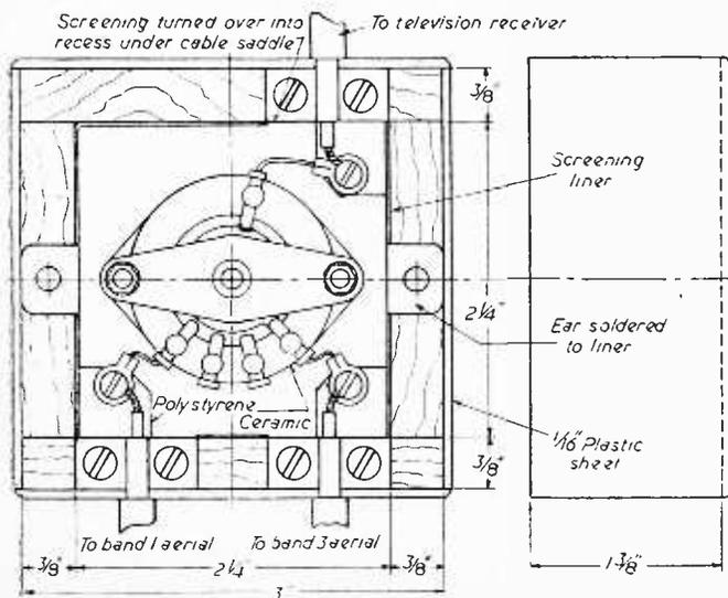
Fig. 1.—General details of the switch.
