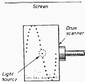
Fig. 53. — This diagram shows how the apertured drum apparatus works.
