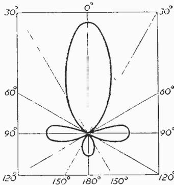
Fig. 2.—Lobes of a Yagi incorrectly matched.
