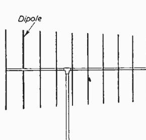
Fig. 3.—A highly directive Yagi.
