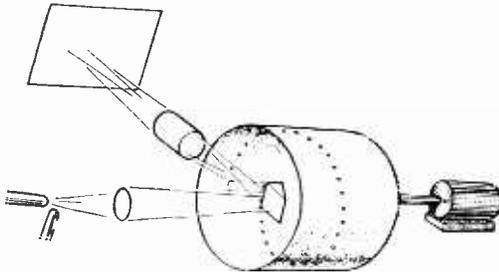
Fig. 55.—Using an external light with a drum scanning apparatus.
