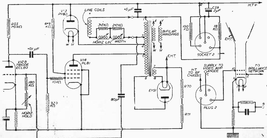
Fig. 5.—Circuit of the line timebase.
