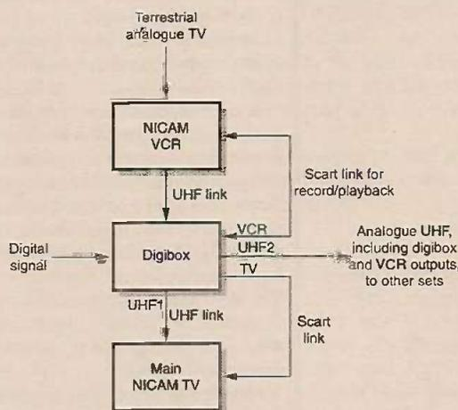
Fig. 2: Reversing the positions of the digibox and VCR, together with the use of scart connections, enables the digibox and VCR output signals to be played back via other TV sets in the system.
