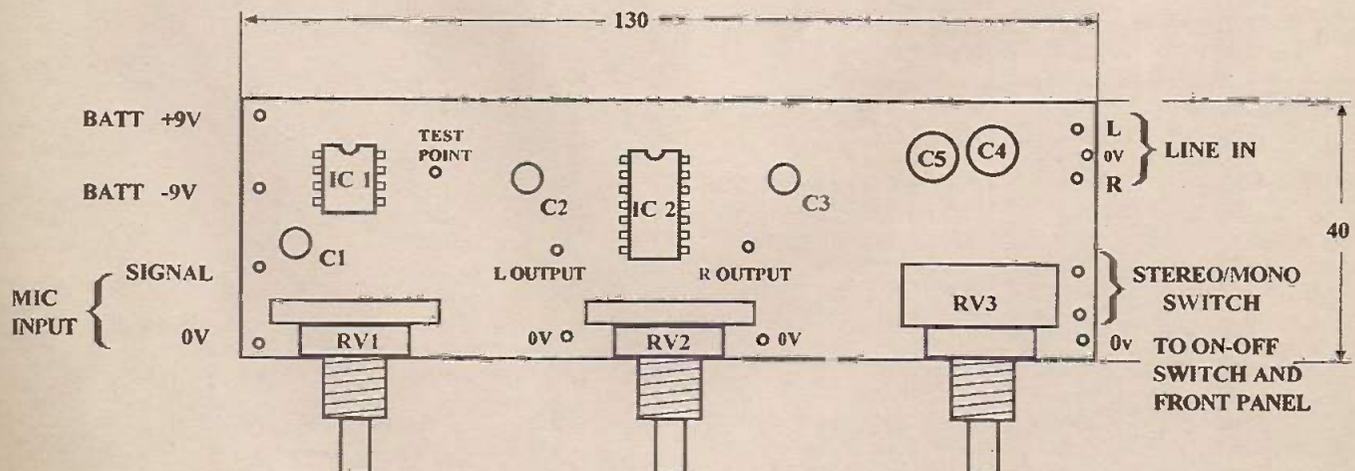
Fig. 4: Positions of the main components and connections on the stripboard. This is a suggested guide for the upper (component) side. Use the front panel as a template to position the potentiometers. Cut the potentiometer shafts to 9mm and enlarge the holes for the potentiometer legs to 1mm.
