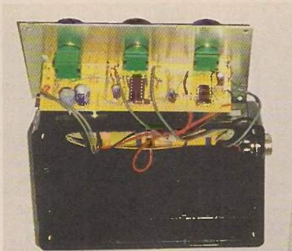
case, especially from the front panel where they can look very untidy and amateurish. My solution is simple: the control potentiometers are fitted to the panel, and the stripboard is attached to the potentiometers' connections and supported by them. As there are no heavy components on the stripboard, it can easily be held in position by the twelve potentiometer connections. The positions of the six leads from the line-level ganged potentiometer ensure that the stripboard doesn't bend or twist.
