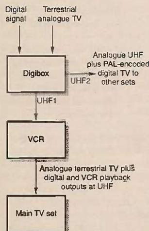
Fig. 1: The usual way of connecting a digibox, a VCR and a TV receiver.
