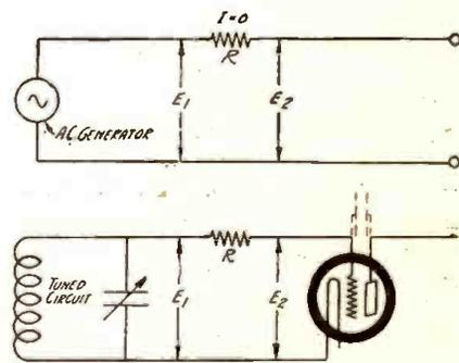
HOW THE SUPPRESSOR PREVENTS CURRENT FLOW
