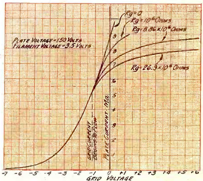
FIGURE 3: A family of grid-voltage, plate-current curves, taken with varying conditions of grid resistance values, indicating the point where grid-current begins to flow.
