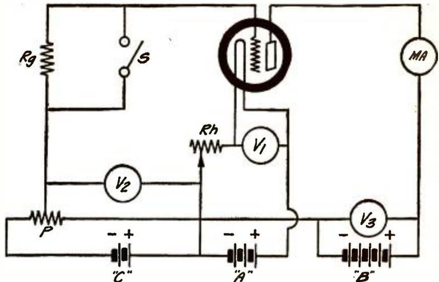
THE CIRCUIT USED IN GRID MEASUREMENT
