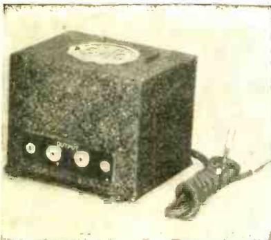
**An Output Unit for Power Valve Receivers**
