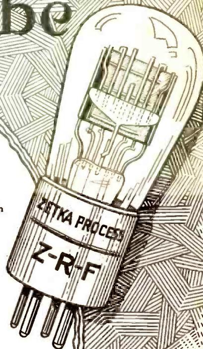
**Z-R-F—Radio Frequency Amplifier.** 5 volts, ¼ amp. High amplification constant. Low plate impedance, and low internal capacity. Uses 90 volts on plate.....Price \$4.50
