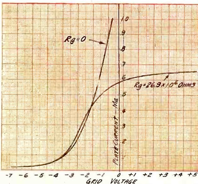
FIGURE 2: A grid-voltage, plate-current characteristic of a vacuum valve, showing how this factor varies with different conditions of grid resistance.
