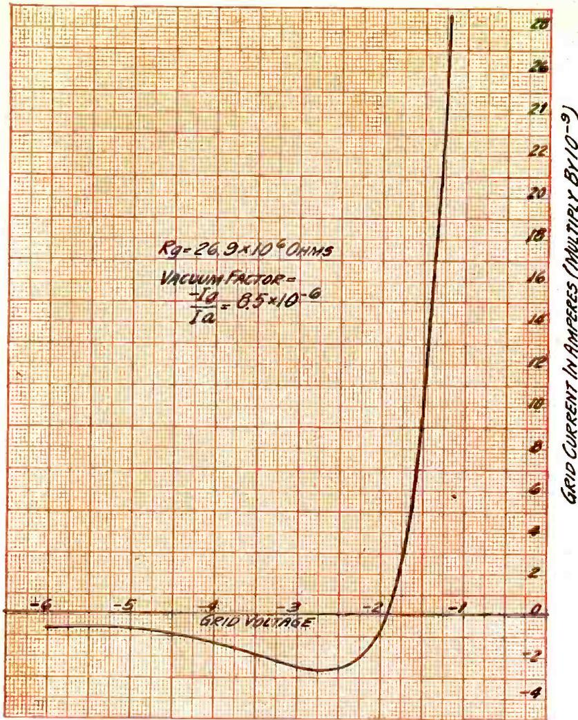
FIGURE 1: A grid-voltage, grid-current curve that shows the variation of these two factors in a vacuum valve.
