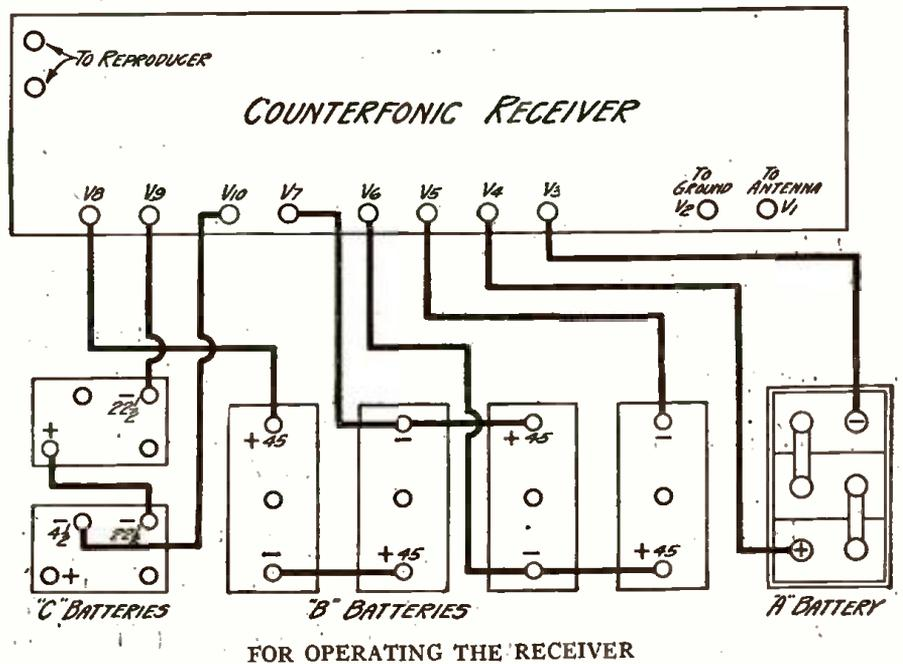
FIGURE 5: The binding posts on the back of the Counterfonic sub-panel should be connected to the batteries indicated in this diagram. The two terminals marked "To Reproducer" are those lettered V11 and V12 in Figure 3.
