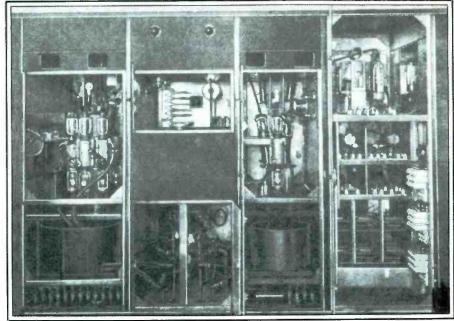
Rear view of one of the transmitters at Dixon, California. Beginning at the left we see water cooled vacuum tubes for the second stage amp, next the interstage unit with tuned circuit and water flow alarms, then the first amplifier stage, and (at the far right) the RF input apparatus.
