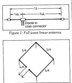
Figure 2: Full wave horizontal quad.
