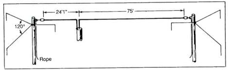
Figure 3: 31M full wave antenna.
