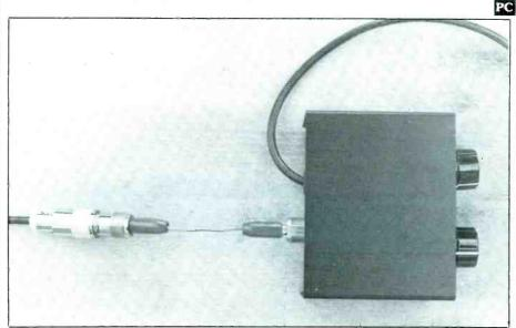
Figure 6: Changeover to single feed of Grove TUN-3 tuner.
