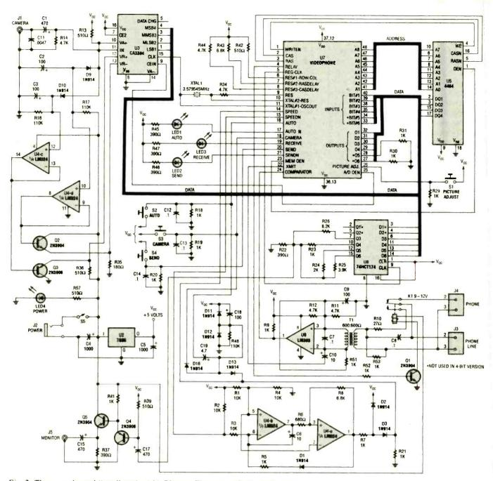
Fig. 2. These are the real "guts" of the 4-bit Phonvu. There are only five basic types of signals handled by the circuit.
