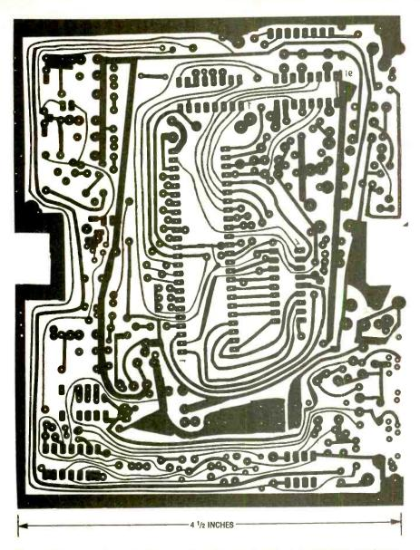
Fig. 4. This is the foil pattern for one side of the main board. It is called the "foil" side because only the LED's and switches are mounted on this side.
