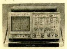
This 300-MHz Tektronix 2440 digital oscilloscope has dual-channel simultaneous data acquisition. As you can see it also has cross-hair style cursors.
