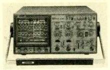
This is the control-panel of a Leader model 2100R 100-MHz oscilloscope. Note the horizontal cursors.
