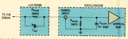
Fig. 2. This is the equivalent circuit of a typical oscilloscope input coupled to a  $\times 10$  probe. The two must be matched for accurate AC operation.
