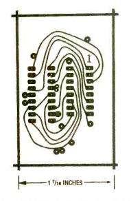
Fig. 5. The adapter board is very simple. It is single-sided, and this is the foil trace.
