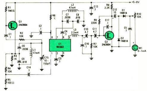
Fig. 3. The NE602 is the heart of the permanent magnet detector. By bringing a magnet close to either LI or L2, the circuit will respond by producing a meter reading, indicating the relative field strength of the magnet.
