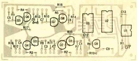
Fig. 3. Here is a parts-placement diagram corresponding to the template appearing in Fig. 2. Note that this diagram shows the placement of the on-board components only.
