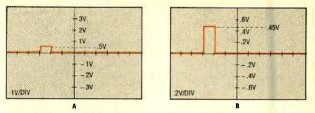
Fig. 4. Increased vertical sensitivity will enhance the accuracy of your readings. As proof of that, the detail lacking in A shows up in B.
