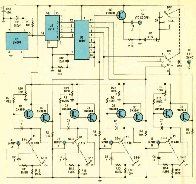
Fig. 1. The Quad Tracer is built around three IC's—an LM567 tone decoder (U1), a 4017 decade counter/divider (U2), and a 4066 quad bilateral switch (U3)—nine NPN transistors (Q1-Q9), and several miscellaneous support components.
