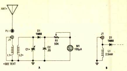
Fig. 6. To build a tuned RF wavemeter follow the schematic shown in A. For an untuned version replace LI, L2, and CI in A with LI in B as shown.
