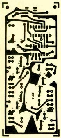
Fig. 2. The Quad Tracer was built on a printed-circuit board, measuring  $4^{7}/_{8} \times 2^{1}/_{8}$  inches; here is the full-scale template of that PC pattern.
