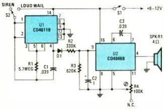
Fig. 6. This sounder has very low power consumption. It could sound-off for a long time before draining its battery power supply.
