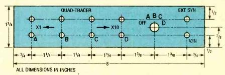
Fig. 5. If you decide to house the circuit in a cabinet like the one the author used, you can simply follow the front-panel layout shown here. In the author's prototype, potentiometers R20–R23 are lined up across the rear panel, directly opposite the positions of J3–J6 (inputs A through D).
