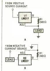
Fig. 2. Adjustable regulators that float can be used as current limiters. Positive regulators can limit the current from a voltage source to a load (A), and negative regulators limit the current from a load to ground.
