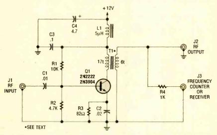
Fig. 4. This wideband-amplifier circuit has two outputs: one for equipment that needs some pre-amplification and another for devices that handle small signals.
