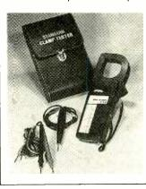
ture meter readings. Also supplied are a set of voltage test probes, a resistance test probe, a spare fuse, a carrying case, and an operating manual. The compact instrument weighs just over 16 ounces.
