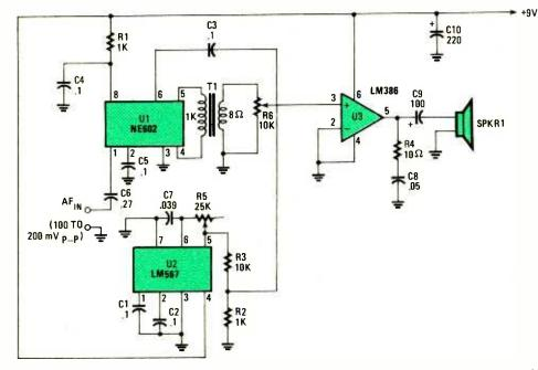
Fig. 2. In this single-mode inversion voice scramber/descrambler circuit, the NE602 is configured as a balanced modulator/demodulator.
