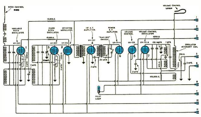
The theremin's wiring diagram shows the functions of all tubes (see the text); the lugs at right connect with the power pack (not shown).
