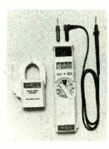
clamp meter. The units are packaged in drop-proof, contamination-resistant, fullysealed, yellow cases. Superior overload protection allows the meters to withstand 1000 volts DC and transients up to 6000 volts on any voltage range. Other ranges can withstand 500 volts. Metal-oxide varistors, instead of lower-cost spark gaps, are used in the meters for a greater measure of transient protection.
