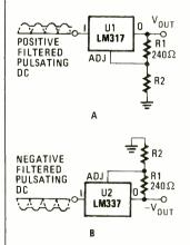
Fig. 1. Adjustable regulators are easy to use. Whether you need a positive (A) or a negative (B) output voltage, you just have to add two resistors and a filtered source of pulsating DC. have a short-circuit, shutdown feature; *i.e.*, short the regulator's output, it turns off and automatically turns on again once the short is removed. They also shutdown if they become too hot.
