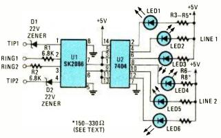
Fig. 4. If you have one or two phone lines that you need to monitor from remote extensions, then give this circuit a try.
