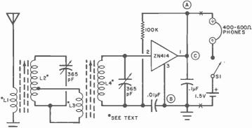
Fig. 2. A 15-foot antenna and tuning coils convert the circuit to receive station WWV.
