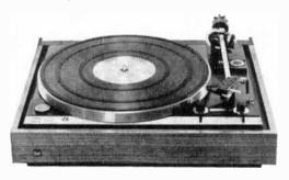
A stylus force gauge on the pivot structure is calibrated from 0 to 3 grams in increments of 0.1 gram up to 1.5 grams and 0.25 gram from 1.5 to 3 grams. The anti-skating compensation dial has two calibration scales (for conical and elliptical styli) that correspond to the tracking force in use. The cartridge mounts in a plastic insert, the latter supplied with a plastic jig that accurately locates the stylus for minimum tracking error.
