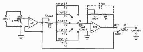
Fig. 3. Simplified buffer amplifier/differentiator has several RC time constants.
