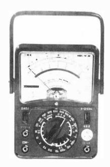
As a transistor tester, the instrument checks alpha from 0 to 0.9965 and beta from 0 to 285. Collector-to-base leakage current is checked in two ranges at 12 and 48  $\mu$ A full-scale for both upu and pup transistors.
