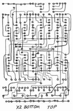
Fig. 2. Rearrange conductor pattern, using two colors, to obtain minimum-size layout.
