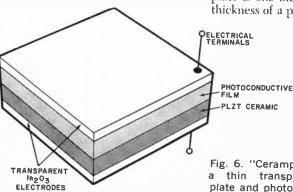
Fig. 6. "Cerampic" image-storing device has a thin transparent ferroelectric ceramic plate and photoconductive layer on one side.
