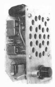
Photo shows how perforated board, with the components, is attached to the front panel.
