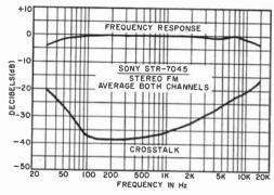
11,500 Hz. It was down 3.5 dB at 30 Hz and 15,000 Hz. Channel separation was 38 dB at middle frequencies and exceeded 20 dB between 30 Hz and 10,500 Hz. It was 16 dB at 15,000 Hz.
