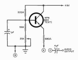
Fig. 3. Receiver performance is improved with voltage regulation and agc isolation.
