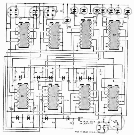
Fig. 1. Convert logic diagram to IC-package format. Indicate off-board components.
