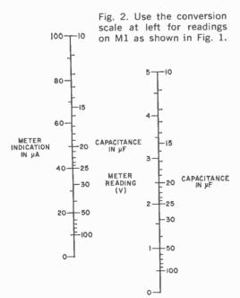
Fig. 3. Conversion scale for external 5-V meter.
