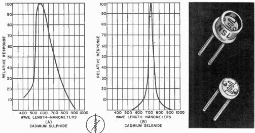
Fig. 2. National Semiconductor photoconductive cells, with spectral responses at left.
