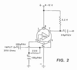
RC-Coupled A-F Amplifier. With only two resistors and three capacitors, the 703 becomes a high-gain RC-coupled audio amplifier as shown in Fig. 2. The 2200-ohm output resistor can be replaced by 2000-ohm headsets or an output transformer (see Fig. 1 for hookup). Note that the input impedance of this amplifier is low—only about 200 ohms.
