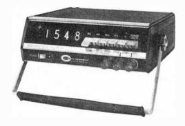
put resistance and ac volts input impedance are both 1 megohm on the 2-volt range and 10 megohms on all other ranges. Resistance measurements are made in seven ranges from 200 ohms full scale to 200 megohms, with a 100-milliohm low end limit. Currents in the resistance mode range
