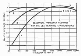
Institute in Standard S1.4-1971. In simple terms, the sound level meter is an a-c voltmeter with a microphone to convert sound energy into an a-c voltage. The addition of a step attenuator, some special filtering networks, and a shaped-characteristic meter sets it apart as a sound level meter.
