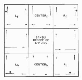
Fig. 10. E-V disc through Sansui decoder.
