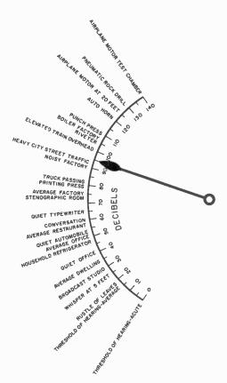
Fig. 1. Normal sounds fall in range from 0 to 140 dB. Instruments which are used to measure sound read in dB.
