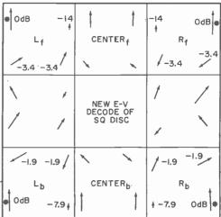
Fig. 13. CBS disc through new E-V decoder.
