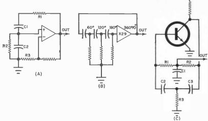
Fig. 1. Various methods of generating sine waves. The Wien bridge is shown at A; the phase-shift oscillator at B; and the twin-T configuration at C.
