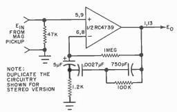
Fig. 3. RIAA phone preamp using the RC4739 has gain of 40 dB at 1 kHz, noise level of 1.7 microvolts referred to the input, S/N 75 dB below 10 mV.
