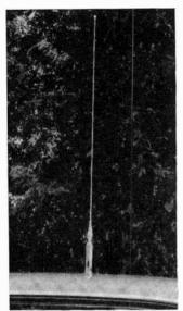
Fig. 4. Another arrangement is the roof-top mounting.
