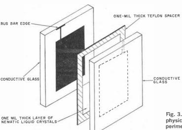
Fig. 3. The diagram shows the physical arrangement of an experimental transmission-type nematic liquid crystal cell.
