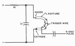
Fig. 1. In basic flash-tube circuit, C1 discharges through tube, after a trigger pulse partially ionizes gas.
