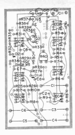
Fig. 2. Actual size foil pattern is at right with component layout above.
