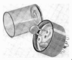
Control chamber consists of an octal tube base, plastic pill container and cover, crystal socket, and two PTC devices. The latter are available at \$2.80 each from Alpha Research Corp., Box 1005, Merritt Island, FL 32952.
