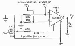
Fig. 4. OTA gain-controlled amplifier
