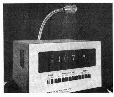
A noise exposure meter compines a sound level meter and an exposure calculator designed to provide unattended operation and a correct readout.
