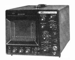
justment control). A built-in sync separator in the TV positions produces stable sync from a composite video input signal. The horizontal amplifier can also be driven from the power line or from an external source. Its gain control can be used to permit up to 2X trace expansion for close examination of any waveform. A pair of positioning controls completes the lineup.
