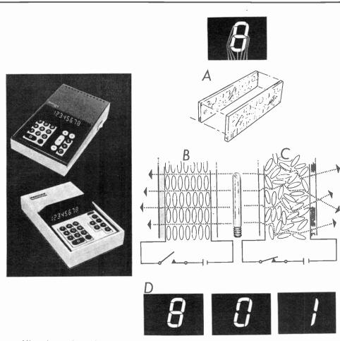
Microelectronic calculators such as those above with liquid crystal displays, are being manufactured in volume by such companies as North American Rockwell. In the display shown at (A), each digit has seven segments, each with an electrical lead, formed on glass plates with transparent tin oxide. Two glass plates are bonded together with about 1/1000 of an inch between them. This space
