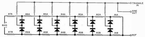
of the six segments for the positive-going portion of the synthesized sine wave. Resistors R1B through R7B bias the lower diodes for the negative peaks of each of the six segments that form the negative-going portion.
