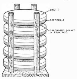
The first part of Volta's paper described the construction and effects produced by his electric pile: ". . . if the sets of triplets of the plates be added 20 or 30 more, disposed in the same order, the actions of the extended pile will be much stronger, and be felt through the arms up to the shoulders; and by continuing the touchings, the pains in the hands become insupportable."
