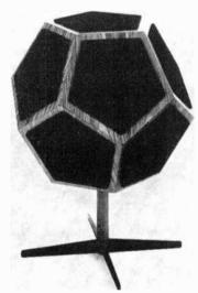
full 360° in a given listening area. Its power response is given at  $\pm 2$  dB from 30 Hz to 15,000 Hz. The system employs nine  $2\rlap/2''$  cone tweeters, a 5" midrange driver, and a 10" high-compliance woofer. A choice of wood finishes and grille colors is available.
