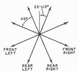
Fig. 4. Scheiber system produces modulation axes  $22\frac{1}{2}^\circ$  rotated from those used in Hafler's system.
