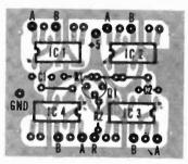
Fig. 8. When mounting electrolytic capacitors, diodes, IC's, and transistors on circuit boards carefully orient them exactly as shown here.
