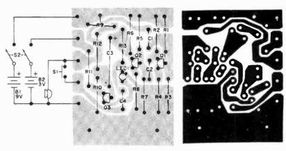
Fig. 2. The PC board foil pattern is shown actual size. When installing the components, use a heat sink on the LED (D1) and make sure that the window is facing the component side of the board. Make the board larger than the foil pattern to allow mounting holes.
