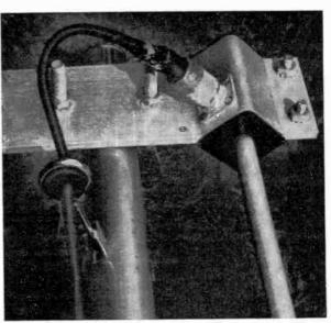
Don't forget to caulk coax cable plug when it is attached to the Astro-Plane input connector. The liberal use of caulking prohibits moisture from corroding the silver plating on the connector and keeps it from entering the coaxial cable.
