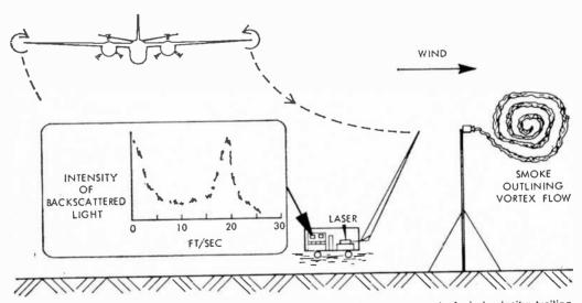
Schematic diagram of the laser doppler technique used for remote measurement of wind velocity; trailing vortex detection experiment. Varying wind velocities are one of the chief causes of CAT. (NASA diagram.)
