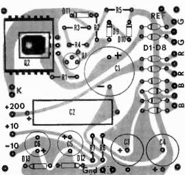
Fig. 2. Actual size etching guide for power supply printed circuit board is provided above. At left is components location and orientation diagram. Carefully follow color coding when secondary leads of T1 are connected to circuit board (holes at near left).
