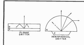
Fig. 3. The critical interface problem. Much more light is emitted by hemispheric diode but some is lost in the thick n-region. Some planar emitters are provided with a reflector to give greater light output.
