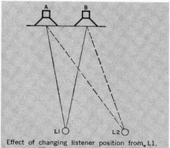
Effect of changing listener position from L1, on-axis with two speakers, to L2, off-axis. Difference in sound path lengths at L2 makes phase shift. Cancellation occurs if difference is ½ wavelength (phase shift of 180°).
