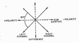
Fig. 1. Stylus motions in two-channel disc groove. Dotted arrows are resultants of left/right axes.
