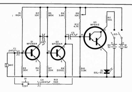
Fig. 1. The LED transmitter consists of a two-stage audio amplifier driving a Darlington modulator. When S1 is depressed, the audio amplifier is converted to an audio oscillator, used for making the original optical setup.
