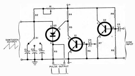
Fig. 1. Programmable unijunction transistor, Q3, is used in sweep/frequency divider circuit to deliver either sawtooth or pulse waveforms synchronized with an external signal.
