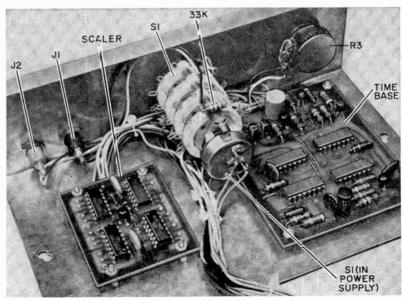
Fig. 10. Time Base and Scaler circuit boards fasten to chassis with 4-40 machine hardware and spacers. A 33,000-ohm resistor ( $\frac{1}{2}$ -watt) is used to limit current through decimal point in readouts. Wires connect to foil sides of boards.
