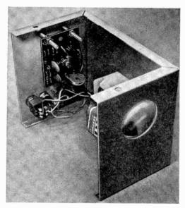
In assembling the transmitter, arrange the board and lens mounting so that the LED window is on the center line of the lens. The text explains how to adjust the board to make the lens focus at the window of the light-emitting diode on board.
