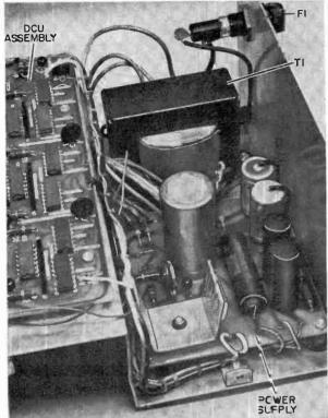
Locations of power supply (right) and  $3\frac{1}{2}$ -digit decoder/driver assembly, reset switch, and display time control (below) are shown mounted on respective sections of main frame chassis.
