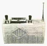
ered with a decorative adhesive-backed vinyl). Finally, connect the batteries and antenna to the appropriate terminals on the radio, and solder the capacitor between the antenna and chassis of the radio to permit peaking the antenna trimmer. You'll find that the converted radio has excellent sensitivity and selectivity, good sound (especially if it has a tone control), and more than enough power for comfortable listening.
