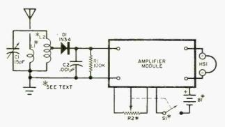
Circuit of the modulation monitor consists of simple crystal detector coupled to audio amplifier module.
