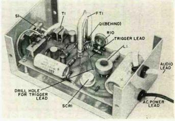
Be especially careful when installing the strobe tube as it is fragile and it cannot withstand mechanical shock.
