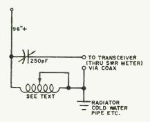
can be used (depending on frequency). Adjust the coil tap and tune the variable capacitor for lowest reflected power. A collapsible whip antenna can be employed, provided that it is 96 inches or *longer*. The coil is made of 30 turns of #14 wire, 8 turns per inch, 2½" in diameter.
