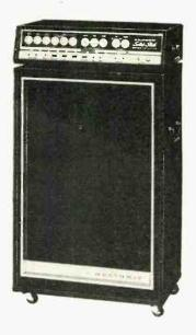
nels with 2 inputs each; "fuzz", brightness switch; bass boost; tremolo, reverb; complete controls for each channel; foot switch; 2 heavy duty 12" speakers plus horn driver. Also available separately kit or factory assembled (Kit Amplifier TA-17, \$175; Assembled \$275; Kit Speaker TA-17-1 \$120; Assembled \$150; Kit TAS-17-2, amp. & two speakers \$395; Assembled TAW-17-2, amp. & two speakers \$545).
