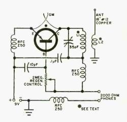
made from two one-inch lengths of #18 insulated wire, twisted together for best results—probably between 1 and 3 turns. Any number of transistors can be used—among them the 2N1023, 2N1026, 2N1397, 2N1233, 2N1469, 2N1474A, 2N1395, and SK-3008.
