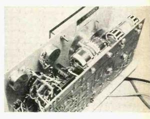
This less-than-\$20 transistorized VOM is expected to usher in a new era of portable test instruments. Test leads are permanently wired to the VOM—one lead for grounding, one for d.c. volts, a third for a.c. volts and ohms. The VOM is housed in special tough plastic case. Two batteries are required to power the solid-state circuit. Assembly takes about four hours. The IM-17 features a panel-mounted polarity-reversing switch.
