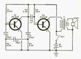
Fig. 3. The two-transistor CPO devised by Charles Rankin utilizes an RC phase-shift oscillator operating at an approximate frequency of 750 Hz.
