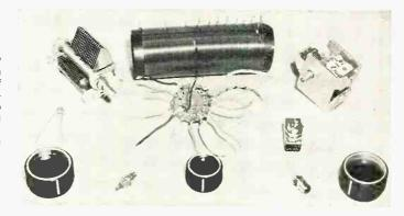
turn to press-fit a brass nail, used as a lug. Scrape the wire adjacent to the lug hole, insert a lug (this is lug #1), and solder to the coil.
