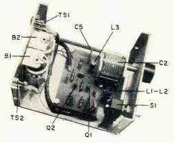
The "Ferret" fits snugly in metal box. You'll have to adjust the height of the metal spacers to permit the shaft of tuning capacitor C2 to clear hole.
