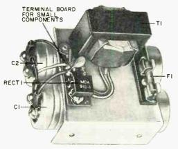
Fig. 6. The power supply is built on a 3" x 3" piece of heavy-gauge aluminum with a 11/2" mounting lip.
