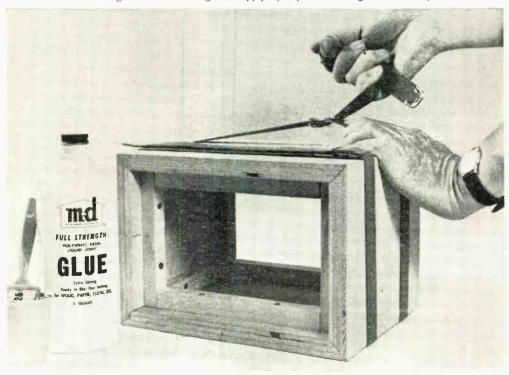
sets. One of the most convenient methods of applying pressure is to use two 48-inch canvas straps. When tightened, the straps force the sides into position for a perfect fit.
