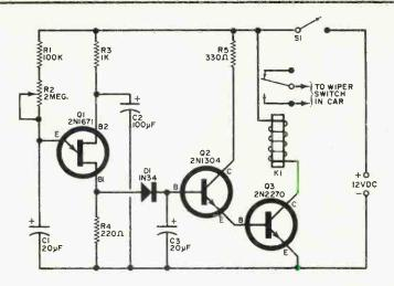
Each time relay K1 closes, it allows the wiper to make one full sweep, at full torque, before returning to its rest position.
