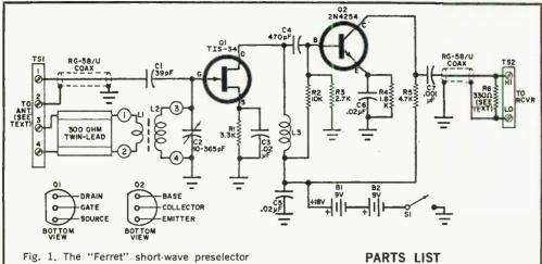
Fig. 1. The "Ferret" short-wave preselector has three optional inputs: one for single-wire-fed antennas, a second for coax-fed antennas, and a third for balanced 300-ohm twin lead.
