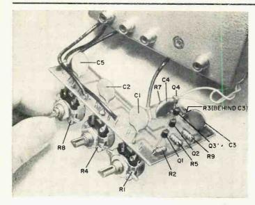
Top view of mixer shows location of some of the components. Potentiometers are soldered in place right onto the printed circuit board. Enlarge the holes for soldering to the lugs of the potentiometers. Hole in back of metal box is for a clamp to secure the battery in place. Carefully observe lead orientations of transistors.
