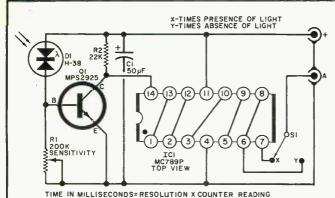
Fig. 11. This high-speed photo pickoff employing a silicon photo-diode is extremely useful in timing fast camera shutters, dragsters, or any high-speed phenomena where a beam of light can be interrupted. The switch permits operation either with presence or absence of light.
