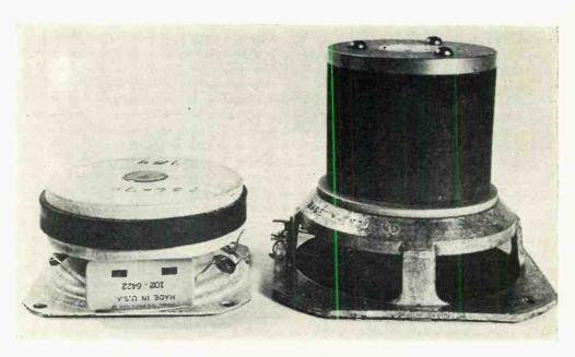
Massive magnet size of both tweeter (left) and woofer are apparent in this photo. Although low cost, these speakers are of modern design and capable of very good sound.
