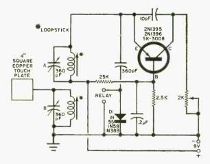
cause a 2-mA, 100-ohm relay to close. Transistors that can be used include the following: 2N1066, 2N1395, 2N1396, 2N1397, GE-1, SK-3007, and DS41. The coils should be mounted close to each other. To tune, set the capacitor in circuit "B" near minimum, and the capacitor in circuit "A" about 3/4 maximum. Adjust the potentiometer for relay closing without touching the plate. Then tune circuit "B" for relay opening. If you touch the plate now, the relay will close.
