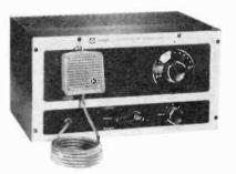
The evolution of CB transceivers is shown by two Knight-Kits (Allied Radio) introduced in 1960 and 1963. Top: the newest kit has double-conversion receiver, multiple channels, maximum utility power supply. Bottom: the older kit, with poor selectivity receiver and only one crystal-controlled channel. system where distance and possible channel interference are involved.
