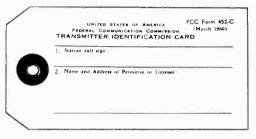
This identification tag should be attached to each CB transceiver. Patterned after FCC Form 452-C, it is supplied by manufacturers with their equipment.
