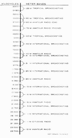
Frequency and wavelength subdivisions in the short-wave bands. On the right-hand side of the vertical bar in each case is the "colloquial" name used in referring to a particular band. On the left-hand side are the upper and lower frequency limitations for each band, which have been set either by international treaty or through accepted usage. These subdivisions apply mainly to frequency allocations and assignments in North and South America.
