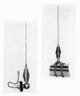
Mobile whip antennas should be spring-mounted to protect both car and antenna. Two methods of attaching base springs are shown here. The mount at left requires a hole in the body of the car. At right is a chain support wrapped around the bumper.
