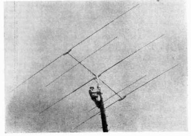
When you spot an antenna like this one, you can bet it belongs to an active ham. Atop the 50' telephone utility pole is Mike Hrindak, W9EHH, Gary, Ind. This rotary beam is designed to function on 10, 15 and 20 meters.
