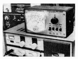
Sitting atop this Olson RA-530 "Spotter" is a General Radiotelephone Model 615 test meter. It can be used to measure power output, feedline performance, and field strength of your own radiated signal. The model 615 meter is typical of the many "combination" test instruments available to the cb'er.
