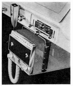
Some CB equipment manufacturers are also producing transceivers for the Business Radio Service. This is the E.F. Johnson "Viking 202," suitable for BRS use between 25 and 50 mc. Sold for about \$200.00, it consists of a 10-tube AM circuit.
