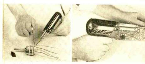
Joining wires, or making connections to tie lugs, pigtail leads or terminal strips, is accomplished efficiently with a 100-watt gun. Instant-heating feature of electric gun is useful for work on printed circuits.
