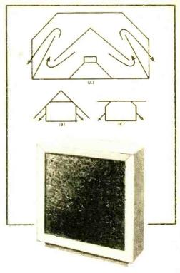
Sound path in Stephens enclosure (above) is shown by arrows. Horn is formed by the cabinet's internal paneling which permits placement against wall if corner is not handy. Below, Cabinart's Model KR-3, which depends on corner placement for proper horn loading. Sound path provided by KR-3's structure is somewhat shorter, needs room walls. This model can be built from kit. In both types, highs radiate from front of speaker, bass from rear via the path of the folded horn.
