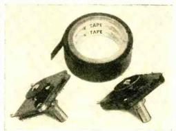
rators. To prevent this, seal the four open sides. The capacitor at the left is shown as it came from the factory. The capacitor at the right was sealed on all four sides with a ½"-wide strip of Mystik tape. Any type of pressure tape could have been used instead.
