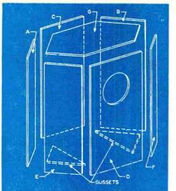
opening will not be visible through the grille cloth. Then the grille cloth can be pulled tightly over the face, around the edges, and tacked to the back side. This panel is now screwed, not glued, in place.
