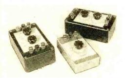
Potentiometers mounted in plastic or metal boxes are handy to have around the workshop or test bench. Paper scales, calibrated with a VOM or v.t.v.m., are glued to top of box. Binding posts connect the potentiometers to the circuit under construction,
