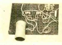
Light-shield tube can be 3" to 12" long. Paint the inside flat black. For maximum sensitivity, insert a flashlight lens in tübe to concentrate rays.
