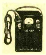
ables the user to connect an electrical load equal to the load of the appliance to be installed on the line. Only three simple steps are necessary to operate it: (1) plug wall cord into outlet to be checked; (2) set load switch No. 1 to the load position
