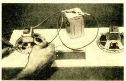
speaker and note the direction in which the speaker cone is moved. Label the terminals according to battery polarity. Do the same with the second speaker, reversing the battery leads if necessary in order to obtain the same direction of cone movement as with the first speaker. Label the terminals, and connect the two speakers with the speaker cord.
