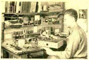
ASSEMBLING A PROJECT. In addition to putting together kits for people in his spare time, Phil can also handle complete hi-fi installations. Here, he is starting to assemble a hi-fi AM tuner.
