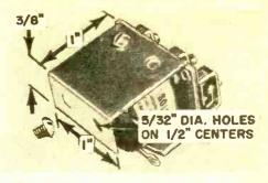
Make a bracket for the relay from scrap metal Space mounting holes to match your relay and leave top screws accessible for adjustment.
