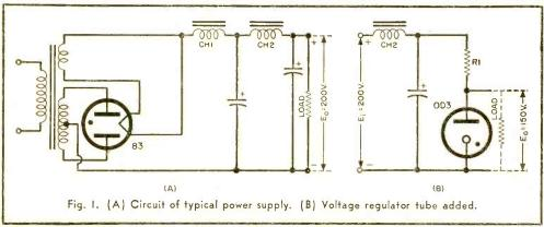
ments, other elements in a power-supply circuit still have to be reckoned with. Figure 1 (A) illustrates a common type of full-wave power supply using a mercuryvapor rectifier. Although this tube makes a substantial contribution to the stability of the supply, the constant resistance of the filter chokes (CH1 and CH2) is still present in the circuit. Hence, changes in load that cause varying drops in potential across these components will still be responsible for serious output fluctuations.
