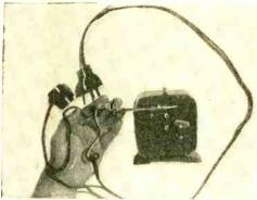
tion of the switch before it affects the circuit again. Reverse the position of the switch in the clip, and your timer will turn devices either on or off.
