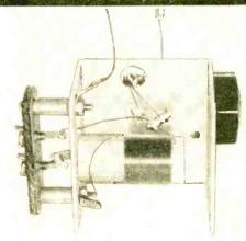
Variable capacitor essentially constitutes this little unit, compared in size with a pack of cigarettes at top of page. Construction is shown directly above, wiring diagram below.
