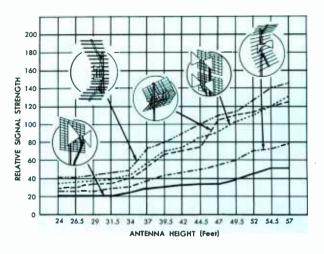
Fig. 6. Vertical Field-Strength Patterns of Several Antennas Tested at Position 2 (Virginia Beach).
