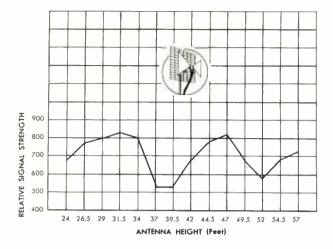
Fig. 17. Vertical Field-Strength Pattern at Position 11.
