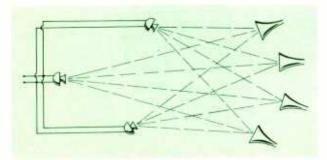
Fig. 4. Single-Channel Pickup of Multiple Sounds With Multiple Microphones.
