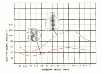
Fig. 11. Vertical Field-Strength Patterns at Position 7 (South Mills).
