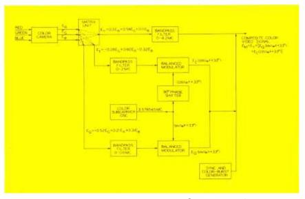
Fig. 2. Block Diagram of Video Section of a Color-TV Transmitter.
