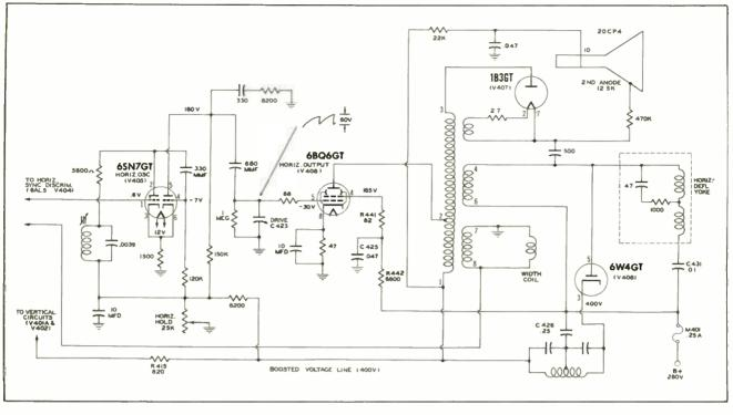
Fig. 6. The Horizontal-Deflection Circuits of an Admiral Model 21F1 Receiver.
