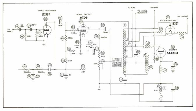
Fig. 3. Partial Schematic of General Electric 2117 Showing High-Voltage Stabilizing System.
