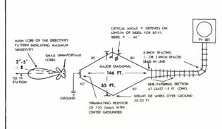
Fig. 4. Plan View of Final Rhombic at Receiver.
