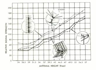
Fig. 7. Vertical Field-Strength Patterns of Several Antennas Tested at Position 2 (Virginia Beach).
