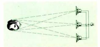
Fig. 6. Listening With Two Ears to Single-Channel System With Multiple Laudspeakers.
