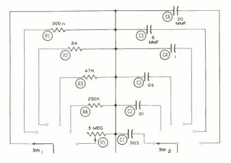
Fig. 4. A Schematic Diagram of the Substitution Box.
