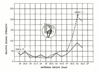
Fig. 4. Vertical Field-Strength Patterns at Position 1 (Pinewell).
