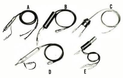
Fig. 3. Typical Test Probes (A) Crystal Detector (B) Self-Bucking Detector (C) Balanced-Input Detector (D) Grid-Leak Detector (E) Cathode Follower.
