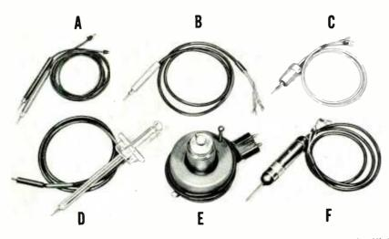
Fig. 1. Typical Test Probes (A) Test Leads (B) Isolation (C) Audio Tracer (D) High Voltage (E) Capacitive-Voltage Divider (F) High Impedance.
