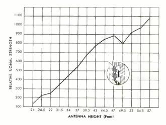
Fig. 18. Vertical Field-Strength Pattern at Position 12.
