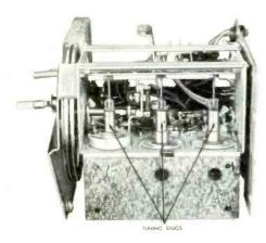
Figure 13. Side View of Turner Model TV-3 with Shields Removed Showing Underside of Tuner.
