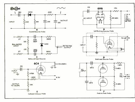
Fig. 4. Schematic Diagrams of Several Test Probes.
