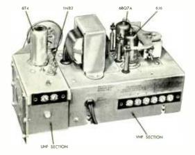
Figure 3. Top and Rear View of Astatic Model CB-1 Chassis.
