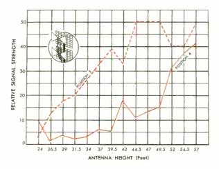
Fig. 9. Comparison of Field-Strength Patterns Illustrating the Effect of Dense Foliage on a UHF Signal.
