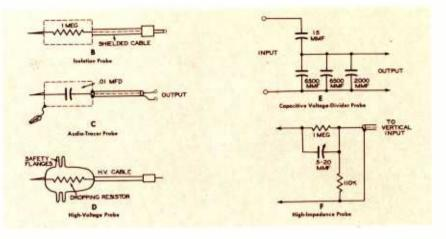
Fig. 2. Schematic Diagrams of Several Test Probes.
