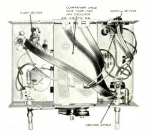
Figure 10. Bottom Chassis View of the Silverline Model 63A, **UHF** Converter.
