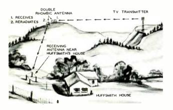
Fig. 1. A Sketch of the Relay System Devised by Dr. Webb to Bring a Signal to Colonel Huffsmith's House.
