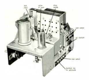
Figure 9. View of Silverline Model 63A, UHF Converter Showing Top Chassis Components and External Connections.
