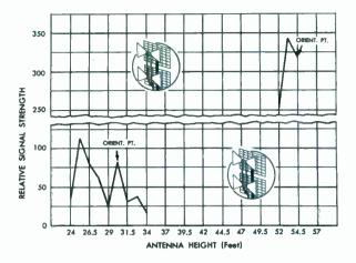
Fig. 5. Comparison of Signal Strengths at Lower and Higher Antenna Elevations. Location is Position 1 (Pinewell).
