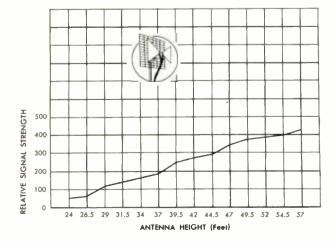
Fig. 19. Vertical Field-Strength Pattern at Position 13.
