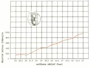
Fig. 21. Vertical Field-Strength Pattern at Position 15.
