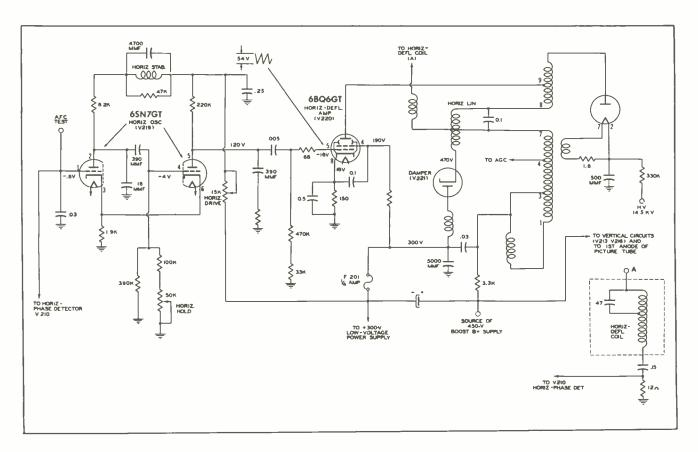
Fig. 5. Horizontal-Deflection Circuits of Some Models of DuMont TV Receivers.
