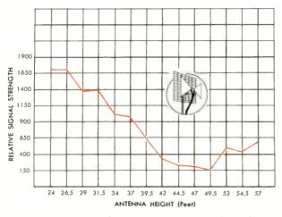
Fig. 13. Vertical Field-Strength Pattern at Position 9 (End of Willoughby Spit).
