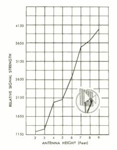
Fig. 14. Field Strength at Low Antenna Elevations (Position 9).
