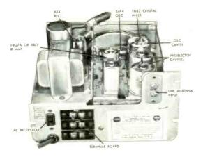
Figure 12. Top Chassis of Turner Model TV-3.
