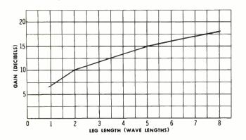
Fig. 3. The Gain of a Rhombic Antenna Increases With Leg Length.
