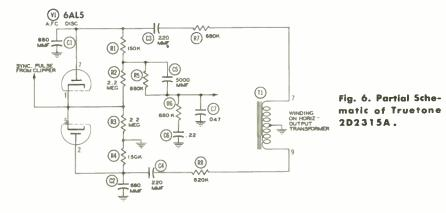
one feedback voltage, this set uses two feedback voltages of opposite polarity and one synchronizing pulse.
