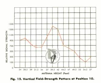
for a satisfactory picture, was reached at a height of 31 1/2 feet. A maximum reading of 250 was noted at the 57-foot level.
