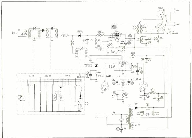
Figure 7. Schematic and Partial Pictorial Drawing of Silverline Model 63A, UHF Converter.
