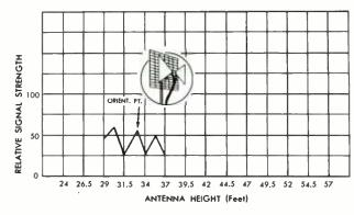
Fig. 3. Changes in Signal Strength at Lower Antenna Elevations. Location is Position 1 (Pinewell).
