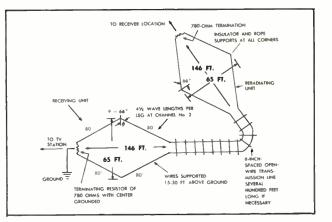
Fig. 2. Diagram Showing How the Receiving and Reradiating Rhombics Are Mounted and Interconnected.
