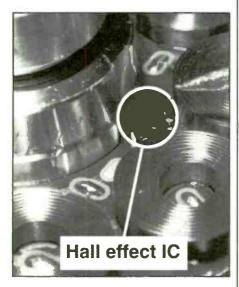
Figure 11. Hall effect ICs are used in VCR motors to control direction and speed.
