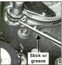
Figure 17. Disassembled record changers showing motor and gear lubrication.
