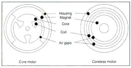
Figure 3. Comparison of a motor with a core and a coreless motor.
