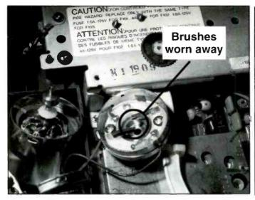
**Figure 12.** This photograph shows the inside of a brushed VCR tape loading motor in which the carbon brushes have worn away after many hours of play.
