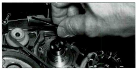
Figure 7. Loosening the shaft collar at the bottom of a VCR cylinder motor.
