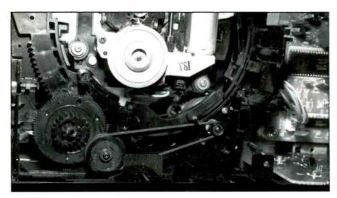
**Figure 14.** In this Pioneer compact disk player, lubrication of the motor assembly and installation of a new belt solved tray opening problems.
