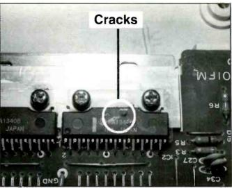
Figure 13. Failed motor driver ICs in a dot matrix printer. The cost of labor and parts to replace them may exceed the value of the machine.
