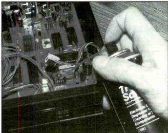
Figure 16. Intermittent connections can also cause motor related problems in consumer products such as in this Kenwood unit which had TOC errors.
