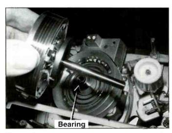
**Figure 8.** Removing the upper video head cylinder in this video cassette recorder reveals the top bearing of the cylinder motor.
