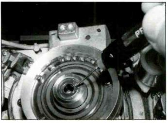
Figure 9. In a cylinder motor, bearings can be lubed with a little oil.
