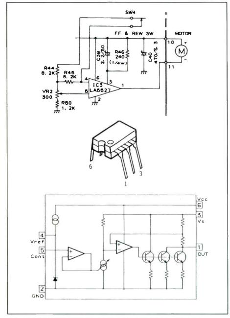
Figure 5. A typical motor speed control circuit used in a portable cassette recorder.
