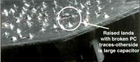
Figure 18. The circuits in radio controlled cars often have broken connections that can affect motor operation.
