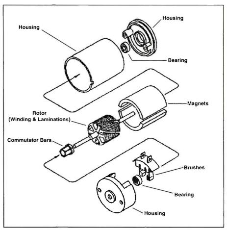
Figure 2. A typical permanent magnet brushed motor design.
