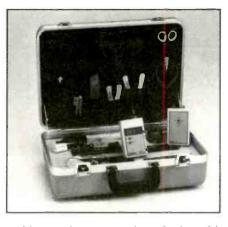
and instructions to terminate both multimode and singlemode fiber in the field and an option for reading the test data into a notebook computer.
