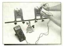
We added an extra pair of circuit board arms to a Model 372 so we could easily test two boards at once. PanaVise holders make it easy to work on circuit boards from 1/8" to 12" wide.
