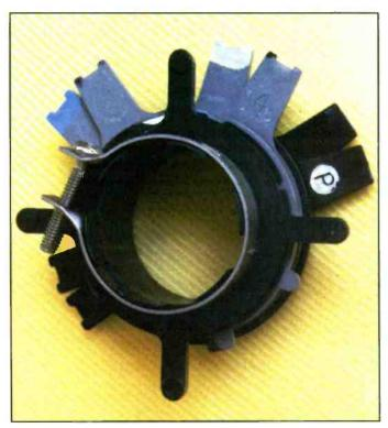
Figure 4. Note that the "lock" on this yoke has four tabs and the others only two each. Turning the lock counterclockwise allows you to move the tabs easier. You may have to break loose a paint-like substance before you can move the tabs. This substance was used to prevent moving the tabs accidentally after the last convergence.
