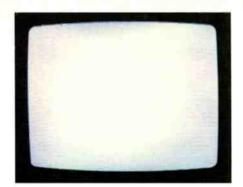
Figure 10. With the brightness control still on mid range without a video signal, turn the red blue and green screen controls up or down until you have a white center screen as shown here. You may or may not have some discoloration around the sides, but if the center is solid white, you're on your way to good convergence.
