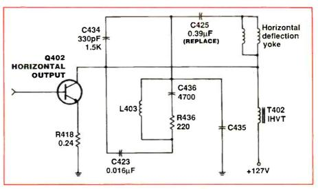
Figure 2. Suspect C425 when Q402 is found to be short circuited.
