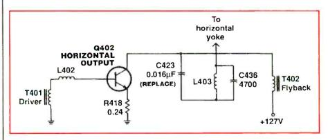
**Figure 8.** Check C423, C425, C426, CR411 CR412, C431, C432 and C433 if the set has shut down and Q402 was damaged.
