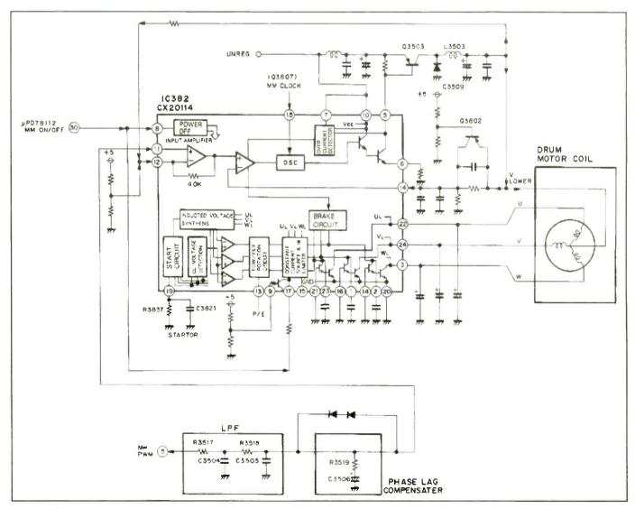
Figure 1. The head drum motor in a VCR is a three-phase motor. The motor drive circuits provide the three-phase alternating current signals needed to generate the rotating magnetic field that spins the motor.
