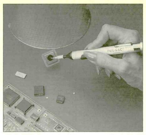
Photo 2. Vacuum-operated component handling devices come in a variety of shapes, sizes and handling capacities. (Photo courtesy Virtual Industries)
