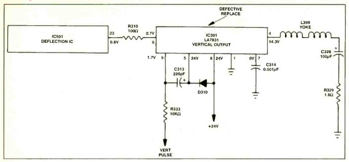
Figure 7. Intermittent and absent vertical sweep was caused by a defective output IC301 in a Goldstar CMT2612.
