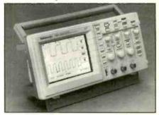
The new scopes rely on digital realtime (DRT) oversampling technology to provide high waveform quality, update rate, and stability. Both models sample at 1 GS/s, at least 10 times their bandwidth. This advanced high-speed technology enables users to capture signal details invisible on analog scopes.
