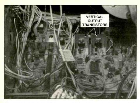
Figure 3. Locate the vertical output transistors by looking for separate heat sinks on the PCB.
