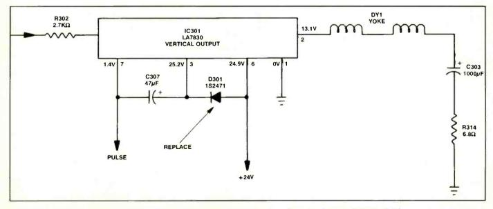
Figure 8. Intermittent vertical sweep and bounce were caused by a defective diode D301 in a Goldstar CMS9841T TV.
