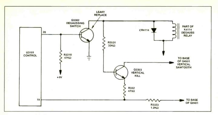
Figure 14. In one RCA CTC166 chassis, a defective degaussing switch transistor (Q3302) killed the vertical output at pin 20 of U3101.
