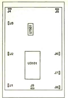
Figure 3. Loose connections between the tuner, microprocessor shields and the printed circuit board in the RCA CTC175/177 may cause no startup, snowy picture, loss of vertical deflection, no audio, and phantom front panel control operation, to name the most common problems. If you encounter any of these symptoms, remove the old solder, carefully inspect the circuit board for cracks, and resolder.
