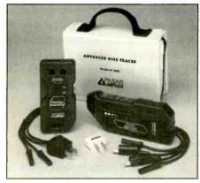
The transmitter can be directly connected to deenergized lines to search for opens or shorts or directly connected to energized lines to identify breakers and circuit paths. The receiver contains two user selected detectors for "Open" or "Current" tracing for a transmitter to receiver range of up to three feet. The circuit carrying the signal is confirmed when the receiver emits an audibly pulsed tome and displays the signal strength visually on the four LED signal strength indicator.
