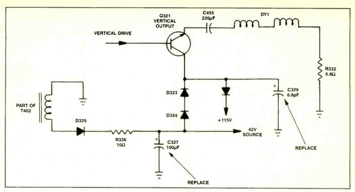
Figure 9. A black area at the top and bottom of the screen was caused by a defective C327 in the low voltage supply of a Goldstar CMR-4160 television set.
