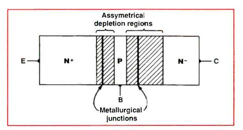
Figure 7. The asymmetrical doping profile and base thickness are important considerations in the design of BJTs.
