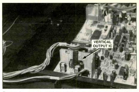
Figure 12. In modern sets, vertical output circuits are contained in a single IC. Look for this vertical output IC on a separate heat sink.
