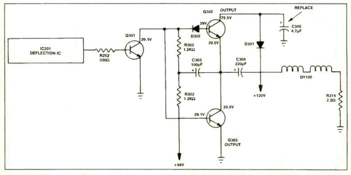
Figure 6. A defective capacitor, C305 (4.7µF, 160V), caused lines at the top of the screen in a Emerson MS250R.
