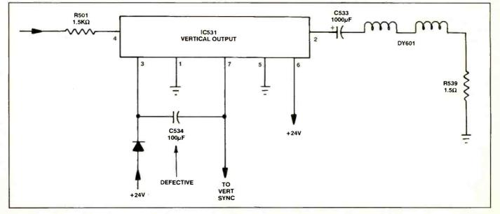
Figure 2. A defective C534 (100µF) capacitor between pins 3 and 7 caused a no vertical sweep in a Sharp portable.
