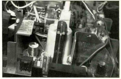
Figure 6. The yoke, transformer, high wattage resistors, degaussing coil, and flyback can arc over and burn.
