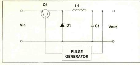
**Figure 4.** A switching power supply senses the output voltage, using it to vary the the duty cycle of a pulse generator that determines the on time of the transistor that provides energy to the output, thus keeping the output voltage relatively constant.
