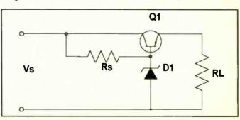
Figure 3. A transistor in the circuit, called a pass transistor because the current passes through it, improves the operation of the basic regulated linear power supply.
