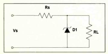
Figure 2. By connecting a Zener diode as shown here, the output voltage of the power supply can be kept relatively constant.
