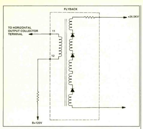
Figure 3. The secondary or high voltage winding of the horizontal output transformer will not show continuity on the highest range of meter.
