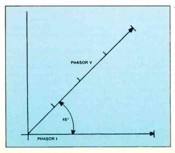
Figure 1. In this drawing, phasor V is ahead of phasor I, that is, phasor V is leading phasor I. Another way of saying the same thing is that phasor I is lagging phasor V.
