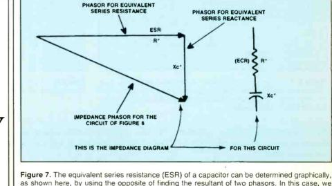
**Figure 7.** The equivalent series resistance (ESR) of a capacitor can be determined graphically, as shown here, by using the opposite of finding the resultant of two phasors. In this case, we resolve a resultant impedance into its capacitive reactance and its resistance. That resistance is the ESR of the capacitor.
