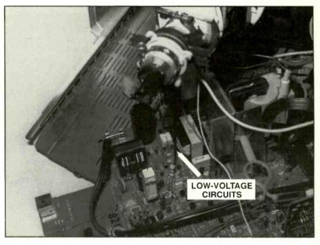
Figure 1. Shorted power line components in the low voltage power supply can cause a fire.
