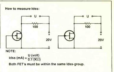
Figure 6. The characteristics of Q203 and Q204 in the Tandberg TPA3006A are critical. Replacements for these transistors must be carefully chosen.
