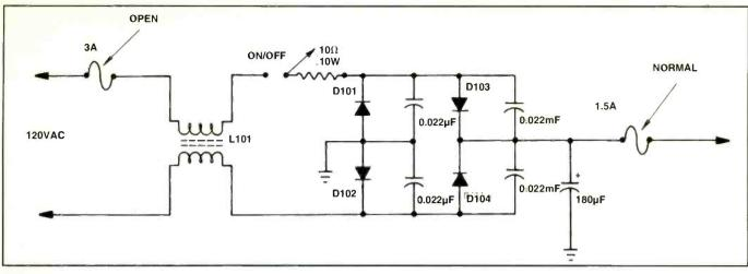
Figure 5. No leakage was found across the silicon diodes and filter capacitor in the low voltage power supply.
