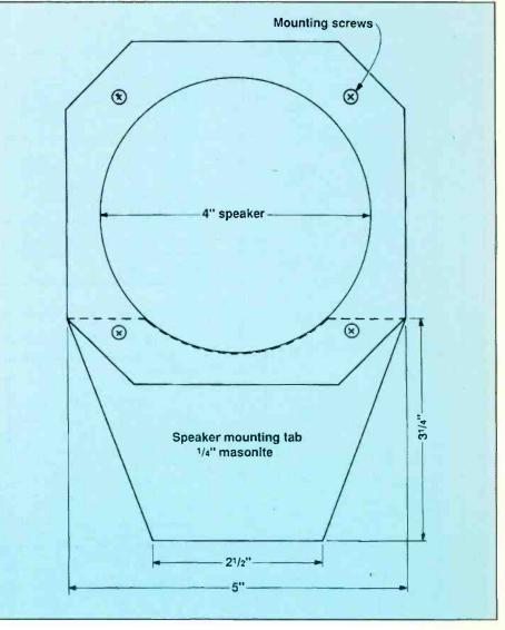
Figure 3. I attached tabs to the speakers as shown. With the tabs in place, mounting the speakers to the chair consisted of simply slipping the tabs between the cushions.
