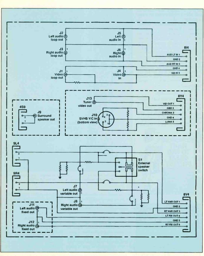
Figure 2. By connecting the speakers to the "Variable Audio" jacks, I can control the speakers volume at my chair using the TV remote control.
