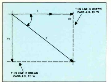
**Figure 3.** This is a different way of representing the circuit of Figure 2. Because current is the same throughout a series circuit, I is used as a reference in this phasor diagram.
