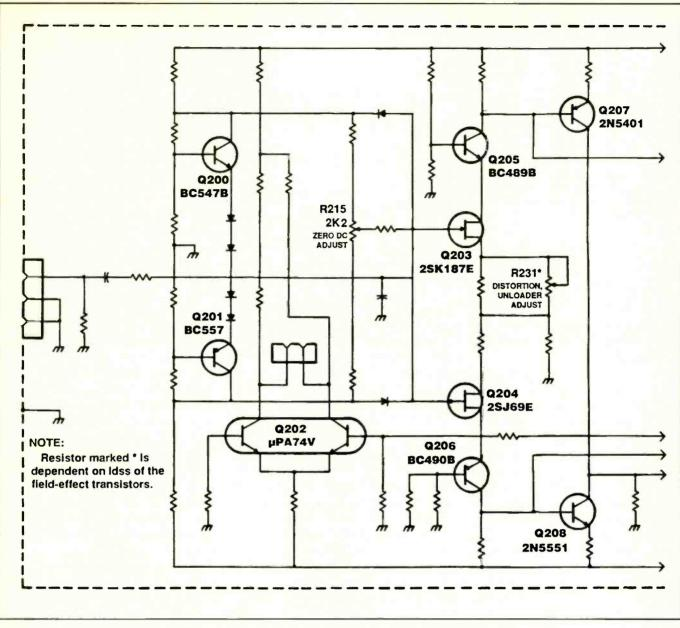
Figure 5. The problem in a Tandberg TPA3006A was caused by faulty transistors Q203 and Q204 in the input section.
