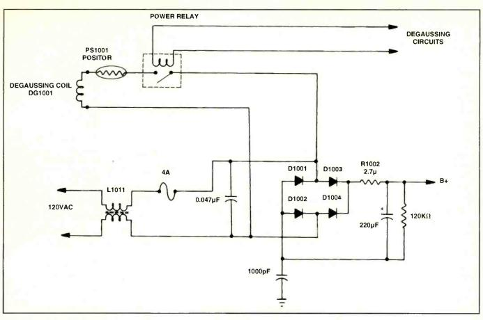
Figure 7. A power relay controlled by transistors or microprocessor closes the degaussing coil circuits to degauss the set.
