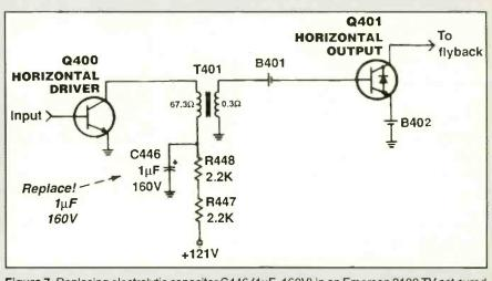
Figure 7. Replacing electrolytic capacitor C446 ( $1\mu$ F, 160V) in an Emerson 2100 TV set cured the problem of a hot output transistor (Q401).
