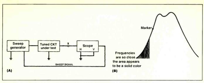
Figure 4. Sweep alignment is carried out using a setup such as this.
