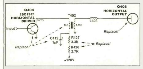
Figure 10. Replacing Q404, Q405, T402, C412, R427, solved the problem of overheating of Q405 in a Sanyo TV.
