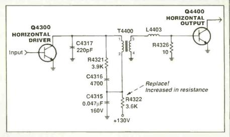
Figure 8. In this RCA CTC140 TV set, I checked R4322 and found that it had increased in resistance. Replacing it restored the set to normal operation.
