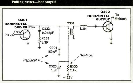
Figure 9. Capacitor C323 and resistor R330 were the culprits responsible for a hot Q302, and C301 (150pF) caused pulling at the top of the picture in a Sanyo TV.
