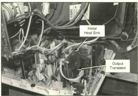
Figure 6. The horizontal output transistor is located on a separate heat sink.
