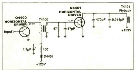
Figure 4. Check the output transistor and components for hot grounds when taking voltage, resistance and waveform tests.
