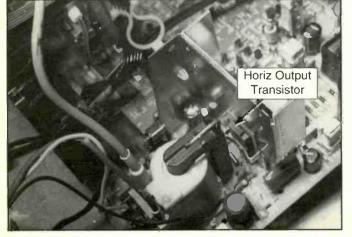
Figure 1. Check the horizontal output transistor after replacement to see if it's still operating hotter than normal.
