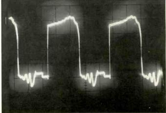
Figure 2. Check waveforms at the base and collector of the horizontal driver transistor, and at the base of the output transistor.
