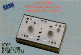
Use this han by semiconductor curve tracer with any oscilloscope (must be ecuipped with X-V mode) and test transistors, triads, UJTs, SCRs, FETs, MDSFETs, as well as zener, signal and rectifier diodes. The LTC-905 will measure (both in and out of circuit) gain (beta), cutoff, leakage and output admittance. Alforcably priced and full featured, the LTC-905 is a "must have" for any serious repair center.
