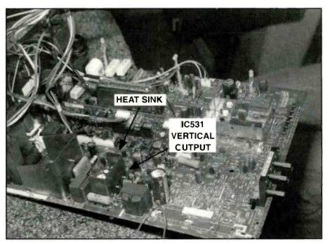
Figure 3. The vertical output IC, IC531, is located on a separate heat sink.
