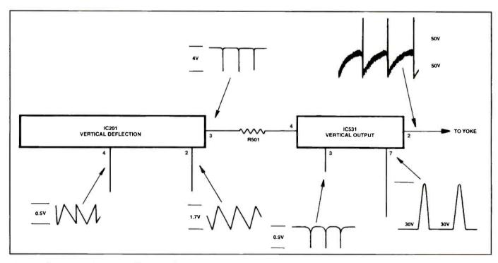
Figure 5. Observe waveforms on IC201 and IC531 to determine what stage the defective component is located in.
