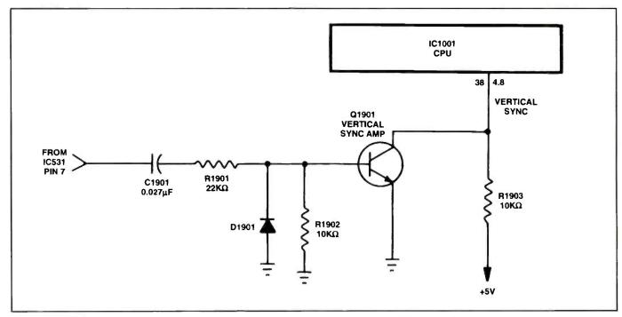
Figure 8. Intermittent vertical sync amplifier (Q1901) terminals produced the intermittent vertical symptom.
