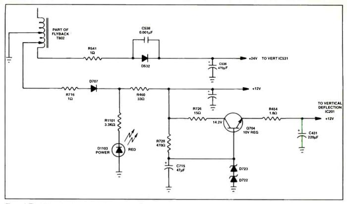
Figure 4. The 12V regulated source supplies voltage to IC201 deflection circuits, and a 24V source is fed to the vertical output IC, IC531.
