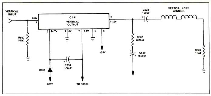
Figure 7. Leaky IC531 can cause improper or no vertical sweep and a low 24V power source.
