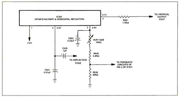
Figure 2. The vertical and horizontal deflection circuits of the Sharp 19SB60R are in IC201.
