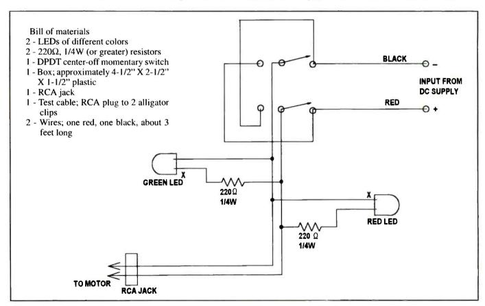
Figure 1. Use this easy to build circuit to diagnose the condition of dc motors.
