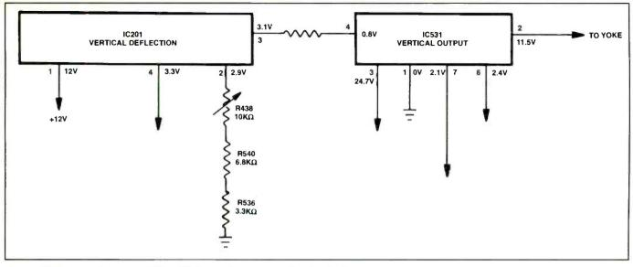
Figure 6. Measure voltage on IC201 and IC531 to determine if either IC is leaky.
