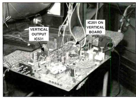
Figure 1. This photograph shows the various vertical semiconductors located on the Sharp
