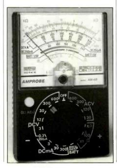
supersede the AM-6A, while providing additional functions and extended range capabilities such as: 1.5V battery test scale, dB scale; for telecommunication applications, higher input impedance  $(4K\Omega/Volt)$ , fuse and diode protected for misapplication up to 250V, 5µA to 300mAdc current measurement capability, 10mV to 600Vdc voltage measurement capability, dual resistance scale up to  $1M\Omega$ , and a larger mirrored display.
