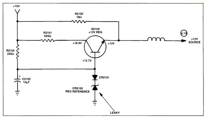
Figure 5. A leaky zener diode, CR210, caused low voltage in the 12V source, which resulted in a very poor picture.
