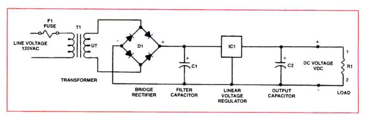
Figure 1. A typical linear power supply.
