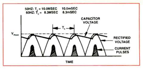
Figure 3. The filtered output of the bridge rectifier looks like this.
