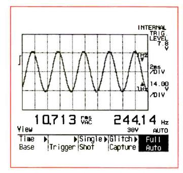
Figure 5. Primary and secondary readings show simultaneous readings of two variables, for example, voltage and frequency.
