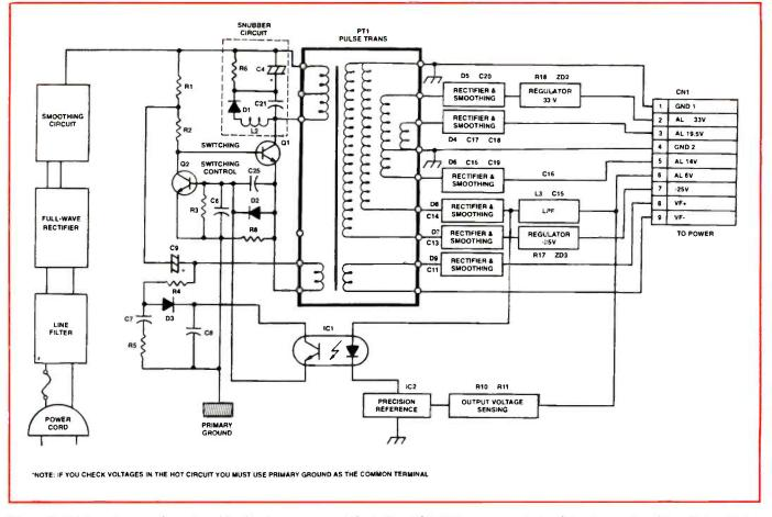
Figure 7. This is a diagram of a real world switching power supply found in a VCR. This power supply is a flyback regulator with multiple outputs. The schematic shows the building blocks of a SMPS described in the article.
