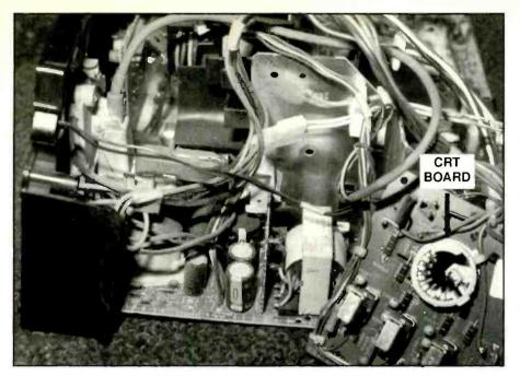
Figure 10. In most modern TV sets, color output transistors are located on the CRT board.
