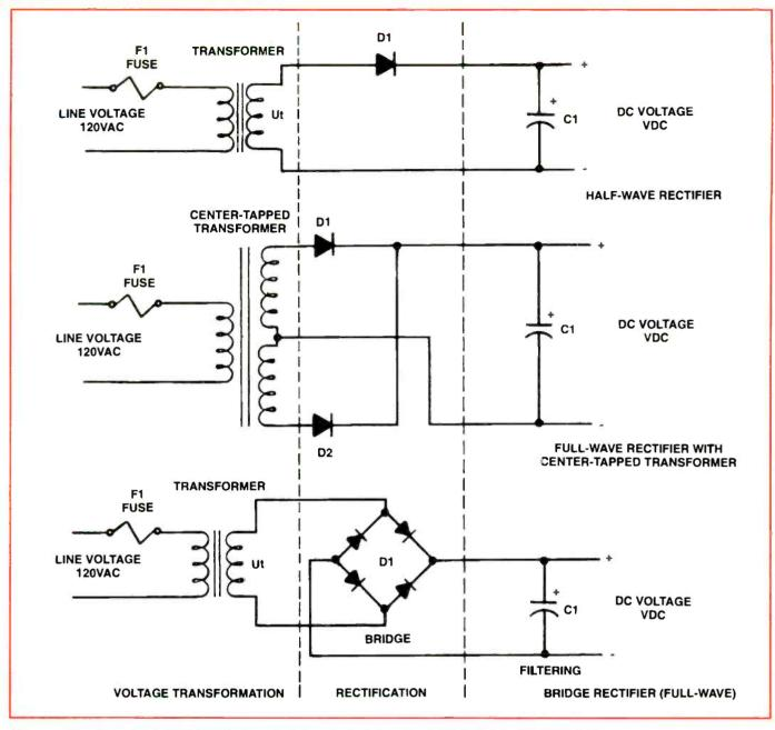
Figure 2. Several variations of the linear power supply have been commonly used in consumer electronics products.
