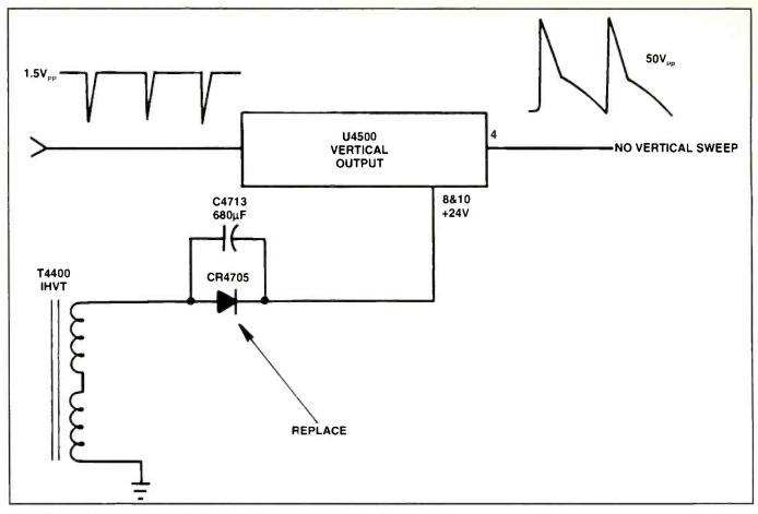
Figure 8. A leaky CR4705 in the 24V source caused the vertical sweep to collapse.
