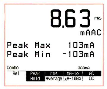
Figure 3. Peak current readings, both minimum and maximum, from the motor.
