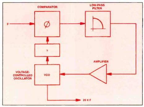
Figure 1. What is the name of the block marked "?" in this diagram?
