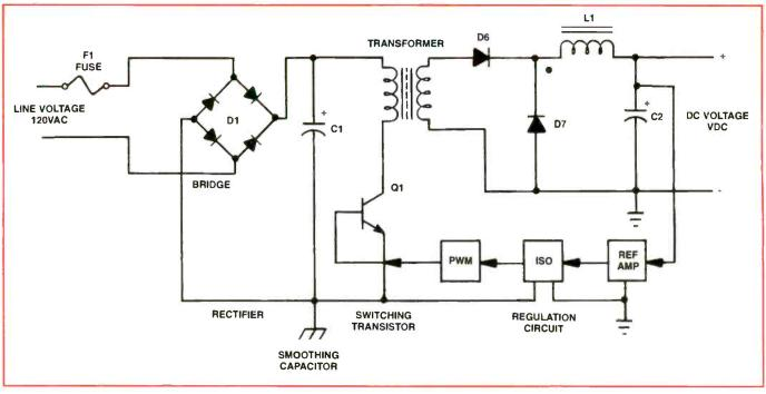
Figure 6. This is a forward switched mode power supply. Although the circuit looks almost like the flyback converter, there are fundamental differences in the operation. This circuit does not store a significant amount of energy in the transformer but in the output inductor.
