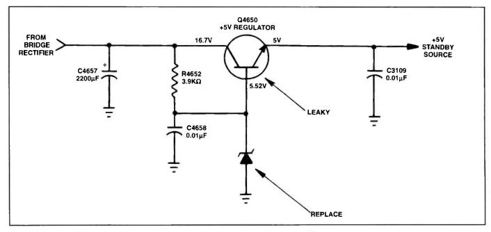
Figure 6. Absence of remote control operation was caused by a leaky zener diode in the 5V power source.
