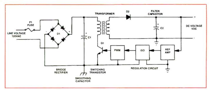
Figure 5. For many consumer electronic applications the flyback regulator, such as this one, is used. A diode bridge is used to rectify the 120Vac/60Hz line voltage. There is no need to use a line voltage transformer before rectification.
