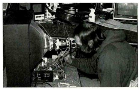
Figure 1. A technician probes a section of a printed circuit board to help locate the intermittent component
