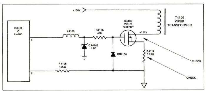
Figure 2. When replacing the VIPUR output transistor, Q4100, in an RCA CTC140, always check R4111.
