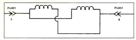
Figure 2A. The vertical windings were incorrectly shown in parallel in this diagram.
