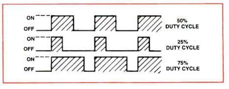
Figure 4. In pulse-width modulation, during the on cycles the pulse train energy is stored in a magnetic field. During the off cycles this energy is used to provide output power.
