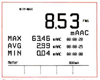
$\textbf{Figure 2.} \ Minimum \ and \ maximum \ rms \ current \ readings \ from \ the \ motor.$
