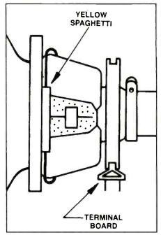
Figure 1. The vertical windings of this picture tube yoke are spliced together inside the yellow section of spaghetti.
