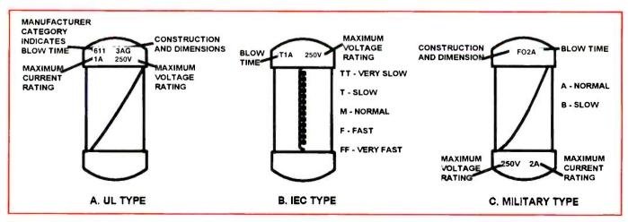
Figure 2. You may encounter different types of fuses, depending upon the type of equipment you work on. These are some of the fuse types you may run across.
