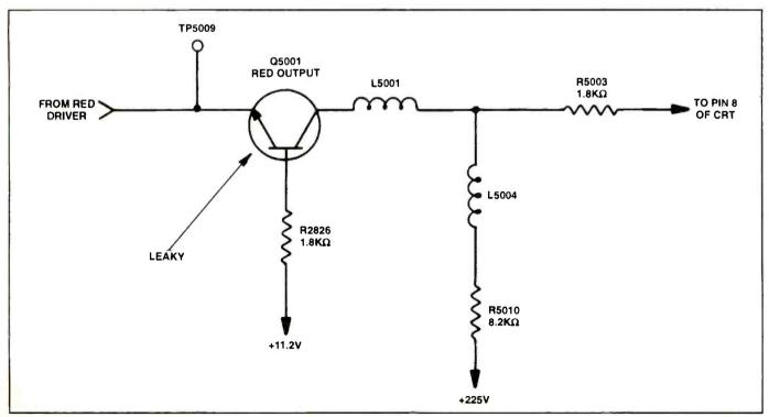
Figure 11. A leaky Q5001, red output transistor, eliminated the color red from the picture.
