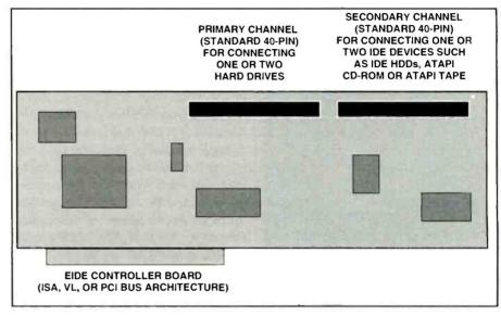
**Figure 1 -** IDE allows two drives (master and slave) to reside on the same port (1F0h) and Interrupt (IRQ 14), but it does not support any other devices. EIDE seeks to overcome this limitation by adding a second "channel" to the EIDE controller.
