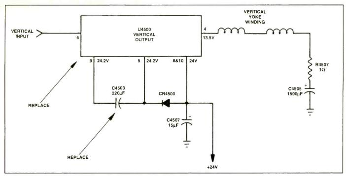
Figure 7. Intermittent vertical sweep was solved by replacing C4503 and U4500.
