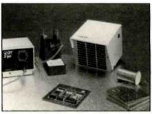
remove solder fumes and other airborne contaminants from the working environment. A powerful fan pulls the fume from the worker's breathing zone. The fumes then pass through an activated carbon filter mat to absorb the noxious gases and odors. This unit is compact in size (8"x 6" x 6") and is useful for situations where benchtop space is at a premium.
