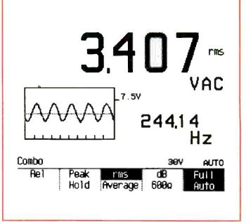
**Figure 6.** Numeric and graphical views combine the features of a multimeter and scope.
