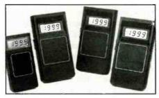
The HHG-14 is a low-cost model with a range of 0.2 to 199.9mG, while the HHG-15 includes an autoranging function which allows accurate measurements from 0.1 to 1999mG. Both models are for measuring 60Hz magnetic emissions. The HHG-16 adds a built-in ability to measure both Extremely Low Frequency (ELF) and Very Low Frequency (VLF) emissions. Both the HHG-15 and HHG-16 offer an optional dc analog output for continuous recording.
