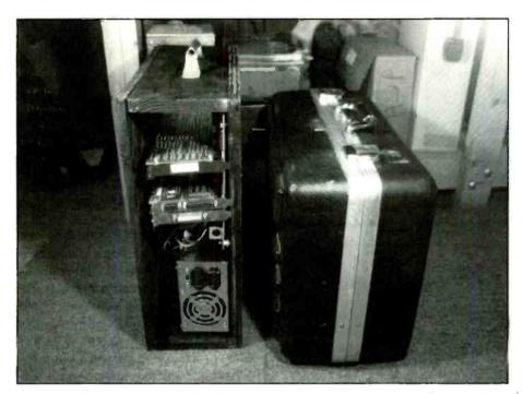
Figure 2. Adding a top provides a place to put a monitor and a handle makes the fixture portable
