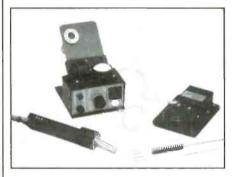
uum flow. Continuous vacuum is achieved through a pneu-vac foot pedal activating a venturi system for an instant vacuum force of 20 to 23 inches of Hg. The station also features an integral temperature control panel. The system requires an inhouse air supply filtered and regulated from 60 psi to 120 psi.
