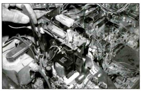
Figure 1. The secondary voltage sources are derived from several windings upon the IHVT flyback.
