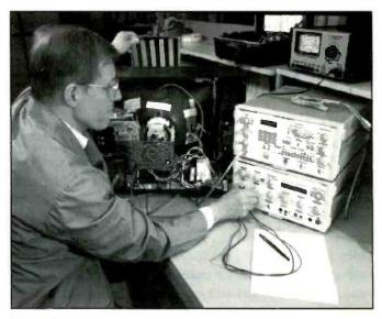
Figure 2. Injecting a vido signal can help narrow the problem to a single defective functional block.
