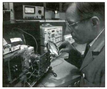
Figure 1. Checking for obvious defects can save troubleshooting time.
