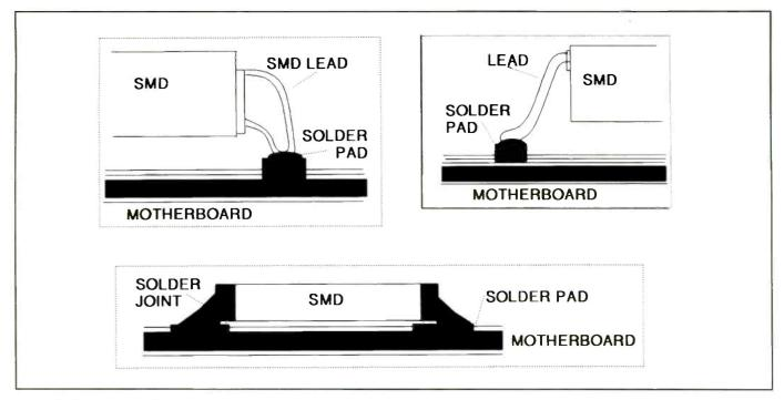
Figure 2. Three types of Surface Mounted Devices.
