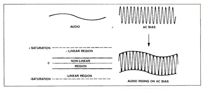
Figure 2. To place the audio signal in the linear region, an ultrasonic bias, in the range of 60KHz to 100KHz, is used.
