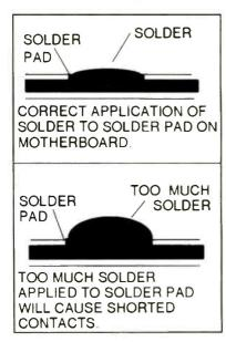
Figure 3. It does not require much solder on the pad to hold the SMD properly.
