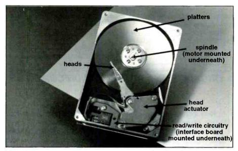
Figure 2. Here is a current hard drive assembly showing the five critical elements.
