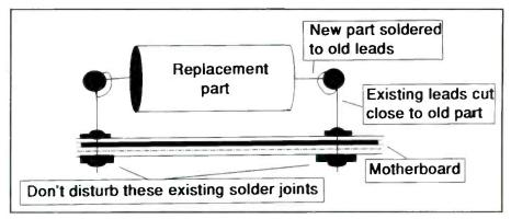
Figure 1. Leave the existing leads in the motherboard by cutting close to the old part. Then, bend the old leads and solder the new part in without disturbing the motherboard.
