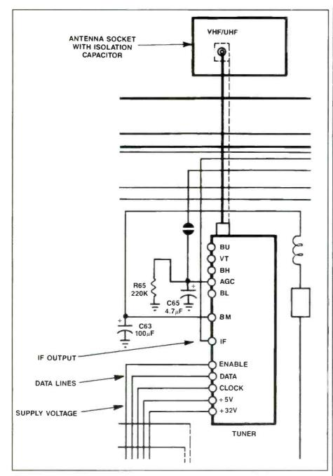
Figure 6. The tuner of the Toshiba TV, CF1311J
