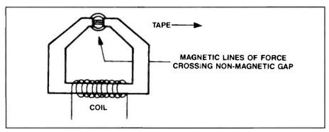
Figure 3. The head places the varying alignment of the magnetic domains on the tape.
