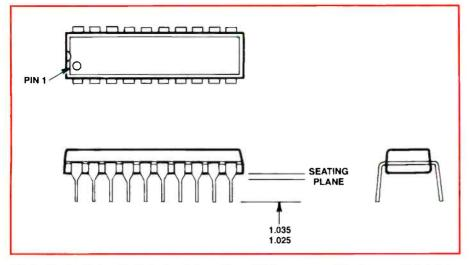
Figure 3. The 20-pin plastic dual-in-line package (PDIP) was one of the early, and still popular, types or IC package.
