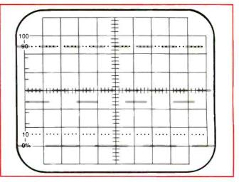
Figure 7. These waveforms show the speed PWM (top) and the phase PWM (bottom) outputs after the problem was corrected.
