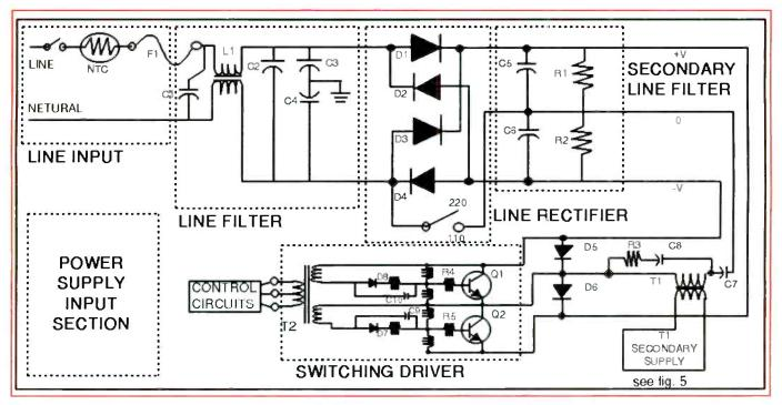
Figure 4. A typical computer power supply input section. In the line input section you will notice the off/on switch, fuse, and the NTC (negative temperature coefficient) thermistor. This thermistor has a high resistance when cold, and as it heats up its resistance decreases. This limits the surge of current when the supply is switched on.
