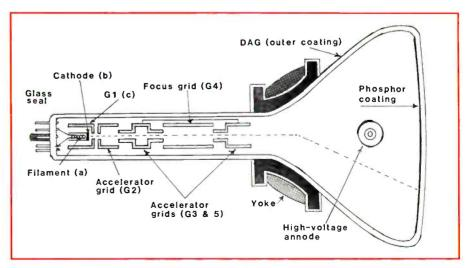
Figure 2. The more commonly used magnetic deflection tubes require a "yoke" mounted on the neck of the tube to deflect the electron beam.
