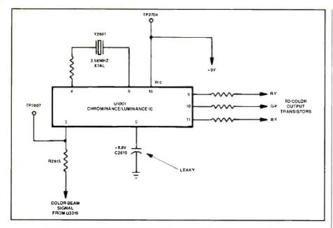
Figure 6. Capacitor C2810 was found to be leaky in an RCA CTC156 chassis that had no color in the picture.
