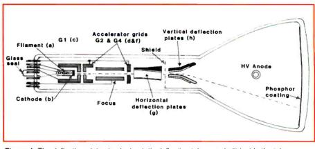
Figure 1. The deflection plates in electrostatic deflection tubes are built inside the tube.
