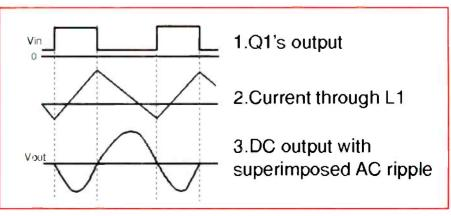
Figure 2. The self-oscillating regulator of Figure 1 will produce an output signal that looks like this.
