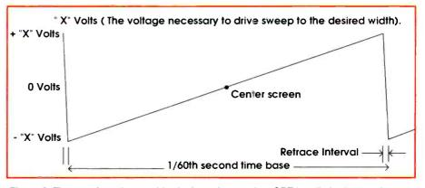
**Figure 3.** The waveform that provides horizontal sweep in a CRT is called a "sawtooth waveform" because of its appearance. It must move the electron beam in the tube horizontally at a constant rate of speed in order to faithfully reproduce the signal applied to the vertical plates.
