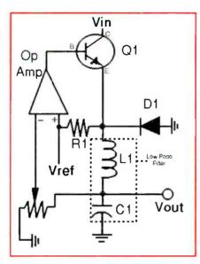
Figure 1. This switching circuit is known as a self-oscillating regulator. The transistor Q1 used in this circuit is commonly known as a pass transistor. L1 and C1 form a low pass filter. When Q1 is off, the current stored in L1 and C1 during Q1's last on state, becomes the source of load current. The diode D1 gives the inductor current a return path, and it is often known as a freewheeling diode.
