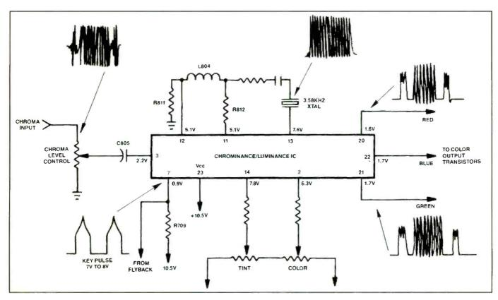
Figure 2. These are typical waveforms and voltages on the chrominance/luminance IC.
