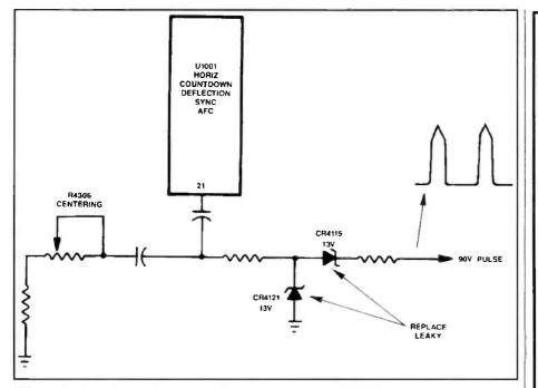
Figure 10. Weak horizontal sync and loss of color in an RCA CTC169 were caused by leaky zener diodes CR4121 and CR4115.
