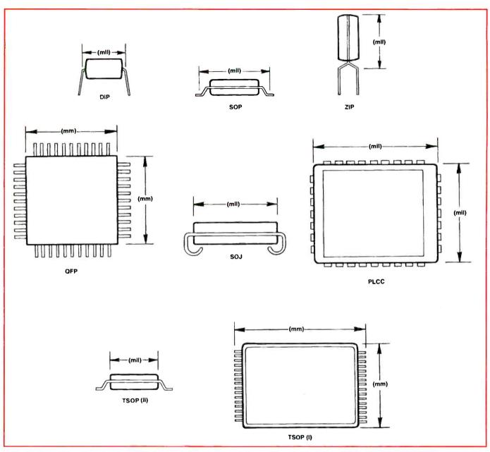
Figure 2. These IC package drawings illustrate some of the package shapes, and give a rough idea of the magnitudes of the packages.
