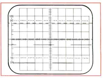
Figure 3. The top waveform is the separated PG pulse output at pin 1 of IC2003. The lower waveform is the separated and stretched PG pulse at pin 14 of IC2003 used for headswitching and phase compar-
