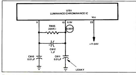
Figure 7. Absence of color in the picture of an RCA CTC117 was found to be caused by a leaky capacitor C811.
