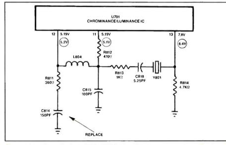
Figure 9. Intermittent color in the RCA CTC120 chassis was caused by an intermittent bypass capacitor, C814.
