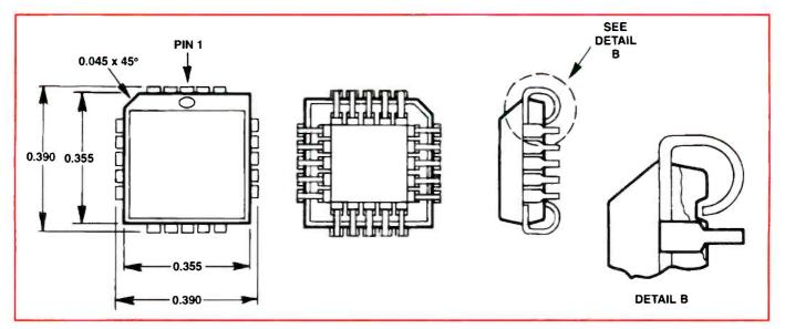
Figure 4. The J-lead plastic chip carrier (PLCC) has leads that exit the body then turn under the component in a curve that resembles the letter J. The leads and the solder joints are relatively strong, but because the solder pads are under the package, removal of these ICs during service can be a problem.
