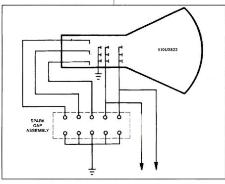
Figure 11. A bright blue raster followed by chassis shutdown was caused by dust in the spark gap assembly of a Samsung K25 chassis.
