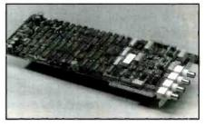
The generators also provide 0.01% frequency accuracy, five selectable output filters, gain and offset controls, and nine built-in waveforms. The output waveforms are accessible via BNC connectors as is the sync out signal. An input BNC connector is provided for signals triggering the generator or for use with an external reference clock. Both generators are capable of 10MHz sine waves and pulses with 20ns widths and 12ns risetimes.
