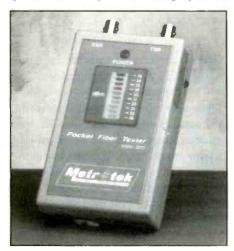
cator measures absolute optical power in 2dBm steps. The tester is available with ST or SMA connectors. Since it contains both a source and a receiver, the unit can be used to test a jumper or a spool of cable. A pair of testers can be used to test long fiber runs between equipment bays or between buildings.
