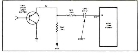
Figure 8. The cause of a negative picture and no color in an RCA CTC131 was determined to be a shorted capacitor C612.
