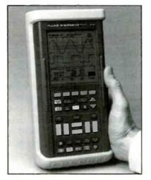
The menu offers direct access to 30 common measurement functions. The user selects the requested measurement from the menu, and the test tool configures itself to make the measurement.
