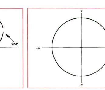
**Figure 2.** This Lissajous pattern is obtained with two sinewaves of equal frequency and equal amplitude. What is their phase relationship?
