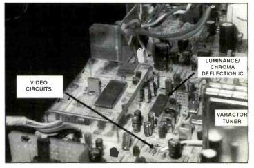
Figure 3. Usually the video circuits are near the luminance/chrominance IC, if and tuner components.
