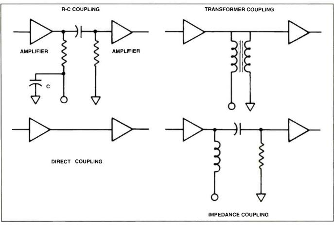
Figure 1. There are only four basic methods of coupling energy from one amplifier to another. R-C coupling, direct coupling, transformer coupling and impedance coupling.
