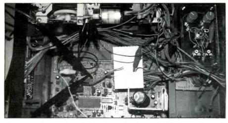
Figure 4. I opened the capstan motor control line and connected the device's positive lead to the motor side of the line and the negative lead to the VCR's ground.
