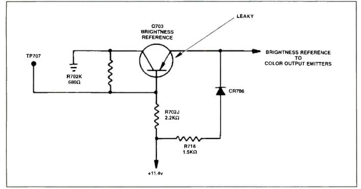
Figure 8. Excessive brightness in an RCA CTC121 chassis was caused by a leaky brightness reference transistor (Q703).
