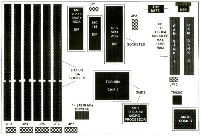
Figure 2. The primary components of a typical 386-SX-40Mhz motherboard. When the motherboard fails, always look first at the simple things. It may be nothing more than a loose jumper or connector. The only socketed chip on this motherboard is the 40-pin 8041 keyboard and I/O interface chip.
