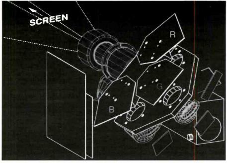
Figure 8. The fully digital prototype of TI's high-definition digital micromirror display based on the digital mirror device technology.
