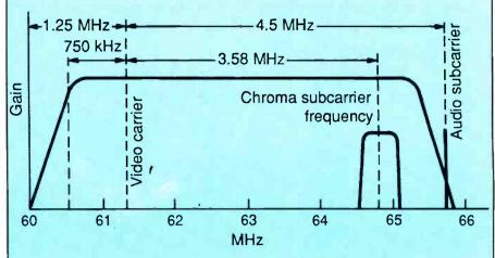
Figure 3. The frequency spectrum of a typical rf channel.
