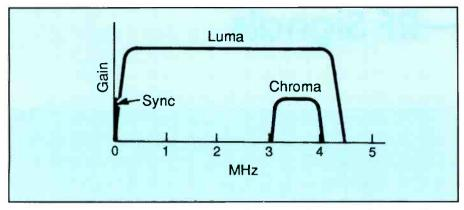
Figure 2. The composite video signal is the product of four different signals: V-sync, H-sync, luma and chroma.
