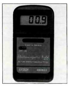
ELF frequency bandwidth of 30Hz to 300Hz. The unit is accurate to 4% at 50Hz to 60Hz with a sampling rate of 2.5 conversions per second to ensure reliable readings. Offering a  $3^{1}/_{2}$  digit 1.5 inch LCD readout with overrange indication, the EMF/ELF Meter monitors electromagnetic radiation levels from video terminals, fans, wiring, power lines, and numerous other sources.
