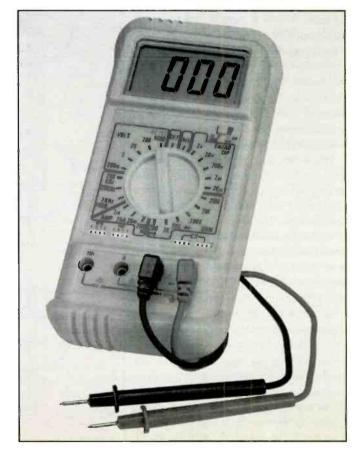
many consumer electronics service centers perform much current reading: that requires that you break the circuit and put the meter in the line.
