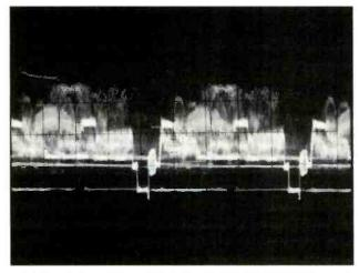
**Figure 2.** The waveform observed with a tuned broadcast station and signal tracing the video circuits with the oscilloscope.
