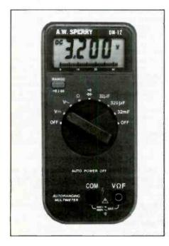
This new pocket-sized autoranging DM-12 is ergonomically contoured for the hand, it has a 200-hour battery life, and recessed safety designed input terminals. Additional features include overload protection on all ranges, a diode test function, capacitance test function and auto power off.
