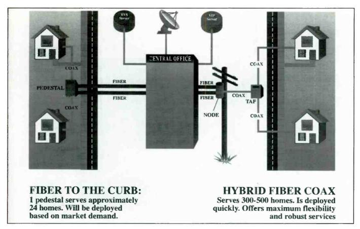
Figure 2. In a switched digital fiber-to-the-curb system, video programming and information are provided in a digitally compressed format (MPEG) by the video information providers and transported digitally by fiber optic equipment to the central office.
