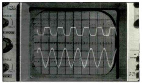
Figure 7. After replacing R259 I could see a clean trapezoidal wave (the correct signal) at the op amp's output regardless of the motor's speed.
