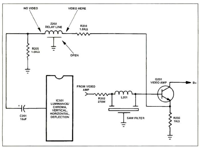
Figure 7. A Goldstar CMT-9428 portable set had no video. The cause of the problem was signal traced to an open delay line (Z202).
