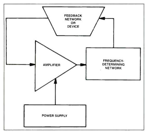
Figure 2. This block diagram is representative of all of the oscillator types, and is useful in troubleshooting any malfunctioning oscillators.
