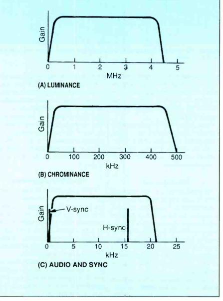
Figure 1. The frequency spectra of the various TV signals.
