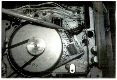
Figure 2. The capstan motor speed/phase control line originates at the servo IC and ends at the capstan motor board after passing through the integrators. At the motor board this line is yellow, whereas all other lines are gray.
