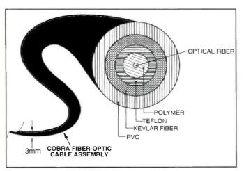
Figure 6. Optical fiber cables consist of an optical fiber, which has a greater tensile strength than steel, jacketed in layers of polymer, kevlar fibers and other plastics. The finished cable has an outside diameter of three millimeters, less than an one-eighth of an inch, and is lighter and more flexible than wire cable.
