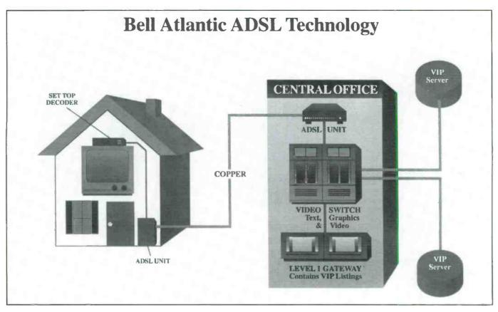
Figure 3. ADSL, in its present state of development, permits the multiplexing and transmission of a one-way, 1.544 Mbps digital signal along with the POTS (Plain Old Telephone Service) or basic rate ISDN (Integrated Switched Digital Network) signal, and a two-way signaling channel on an integrated basis over a single non-loaded copper pair.
