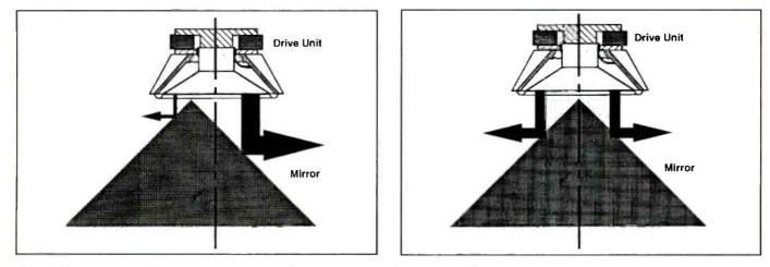
Figure 11. In this system, the sound is aimed at specially designed acoustic mirrors, which produces a stereo listening area greater than the area produced by conventional speakers.
