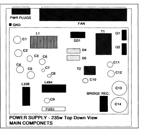
**Figure 1.** The primary components of a 235W power supply. The easily diagnosed and replaceable components include the power plugs and cords, fan, various common capacitors and resistors, input diodes and/or bridge rectifiers, L339, L494, and the fuse.
