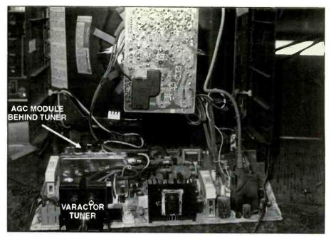
Figure 5. Tapping the AGC module in a Sony KV-139R portable, would cause the picture to pop in and out. At times the picture was a negative image.
