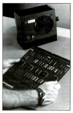
The ionizer is a self-contained, bipolar, intrinsically balanced ionized blower that neutralizes static charge on nonconductors such as insulative tapes, plastics, and circuit board substrates.
