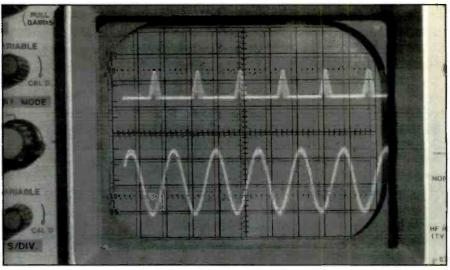
Figure 6. This oscilloscope photo shows the FG signal at pin 2 of IC203 (sinewave at bottom), a quad op amp. Pin 2 was the inverting input of the amp labeled "C.FG AMP". The spike at the top of the screen is the output of the op amp. The positive spike, present only when the motor was running well above its normal speed, occurred during the interval of the negative peak.
