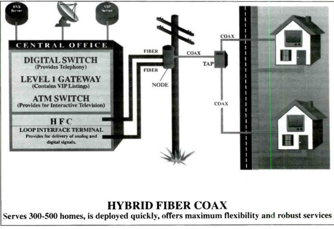
Figure 1. A switched digital hybrid fiber-coax platform will be used in the initial mass deployment of the Bell Atlantic Network. This system, which combines properties of fiber and coaxial architectures, can provide 100 or more analog channels using a bus architecture.
