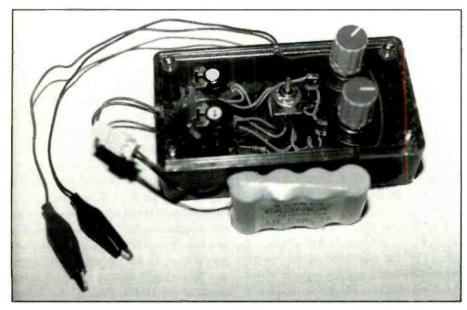
Figure 3. This is a photo of The diagnostic device I constructed. I used a 4.8V Ni-Cd cordless telephone battery to power it.
