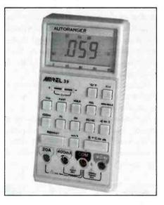
graph. Measurement ranges are 4nF to  $4\mu$ F for capacitance measurement, 100Hz to 600KHz for frequency measurement, 400mV to 1000Vdc, 400mV to 650 Vac, and 400mr to 40M\Omega for resistance measurement. They also offer relative mode, data-hold, min./max., memory/read function and true RMS (Model 37).
