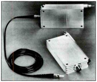
ment (Figure 3), permits the multiplexing and transmission of a one-way, 1.544 Mbps digital signal along with the POTS (Plain Old Telephone Service) or basic rate ISDN (Integrated Switched Digital Network) signal, and a two-way signaling channel on an integrated basis over a single non-loaded copper pair.
