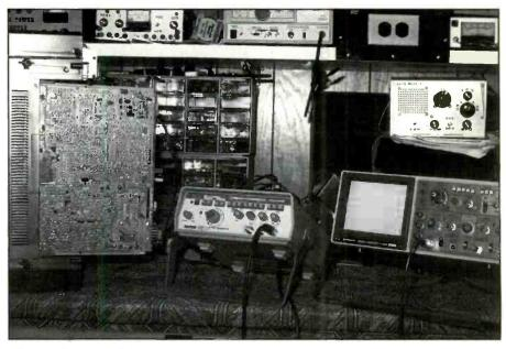
Figure 1. Video circuit problems can be diagnosed by signal tracing using a color dot-bar generator or a sine wave generator, with an oscilloscope as indicator.
