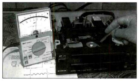
Figure 1. Measurement of the infrared power output of the laser head assembly using a laser power meter may uncover a defective laser diode assembly.
