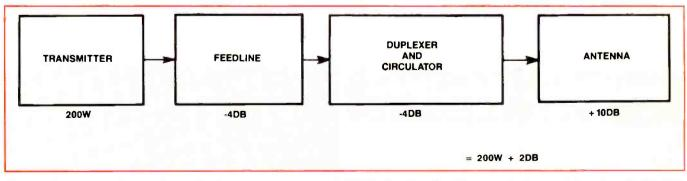
Figure 1. A system consists of a transmitter that has a power output of 200W, a feedline with 4dB loss, a duplexer and circulator with 4dB loss, and an antenna with 10dB gain. What will be the effective radiated power of this system?
