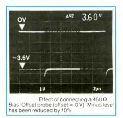
Figure 7. The same pulse as that in Figure 6, acquired with a 450 $\Omega$  probe added.
