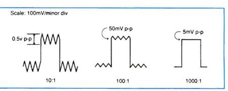
Figure 12. "Cleaning up" a signal by increasing the CMRR.
