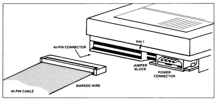
Figure 3. The IBM-compatible IDE interface cable connection.
