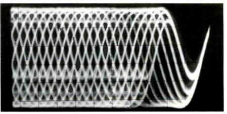
Figure 4. Presence of the EFM (eight-to-fourteen) waveform indicates that the laser optical assembly and rf amp are normal.
