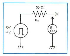
Figure 4. The principle of operation of a bias offset probe.
