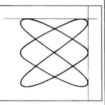
Figure 3. To solve TYEK question number 6, draw horizontal and vertical lines against the curve as shown here. The number of times the curve touches the vertical line divided by the number of times it touches the horizontal line is equal to the horizontal frequency divided by the vertical frequency. In this case 3:2 = 450:f<sub>V</sub>. Therefore, f<sub>V</sub> = (450 x2)/3 = 300Hz.
