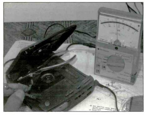
Figure 7. The plastic lid of the portable CD player provides interlock protection as the lid must be closed before the unit will play.
