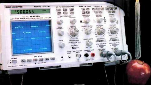
Autoranging....Now you can move your probe from test point to test point without taking the time to re-adjust controls. The exclusive, autoranging timebase and vertical attenuators of the SC3100 "AUTO TRACKER" eliminate this wasted time. By the time you look up from the circuit, the waveform will already
