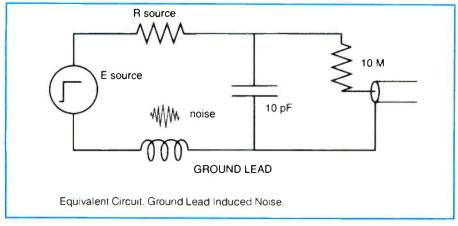
Figure 2. An equivalent circuit of induced ground lead noise.
