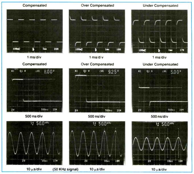
Figure 1. Compensating the probe.
