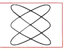
**Figure 2.** In this Lissajous pattern, the horizontal sinewave frequency is 450Hz. What is the vertical frequency?
