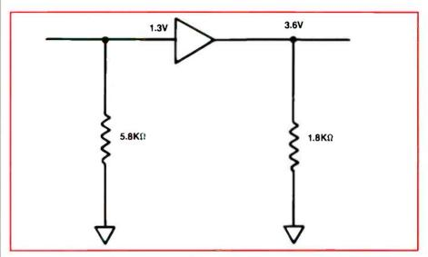
Figure 1. What is the dB gain of this amplifier?
