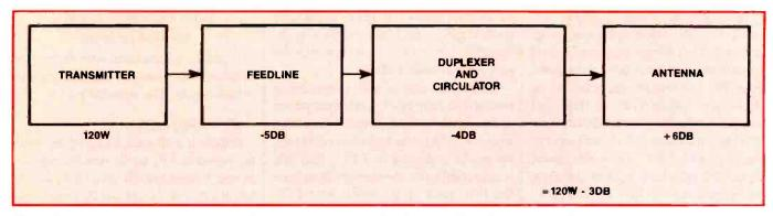
Figure 2. A system consists of a transmitter that has a power output of 120W, a feedline with 5dB loss, a duplexer and circulator with 4dB loss and an antenna with 6dB gain. What will be the effective radiated power of this system.
