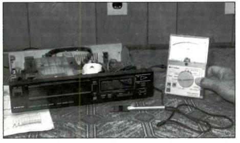
Figure 1. The portable laser power meter will accurately indicate if the laser diode is emitting signal against the underside of the CD disc.
