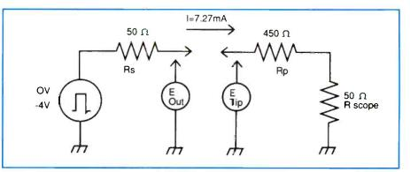
Figure 5. A bias offset probe connected to a  $50\Omega$  source.
