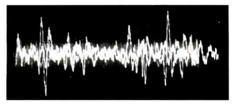
Figure 7. Connecting the oscilloscope across the focus coil winding indicates if signal is present at the coil assembly.
