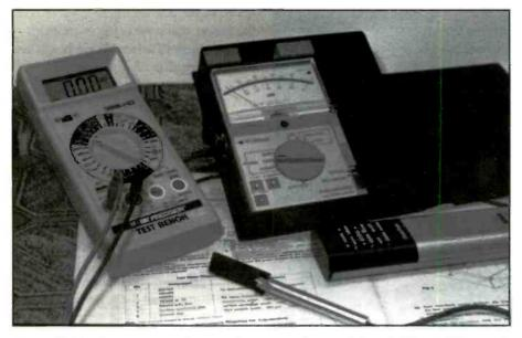
Figure 5. The laser power meter may also be used to test infrared TV and VCR remote transmitters.
