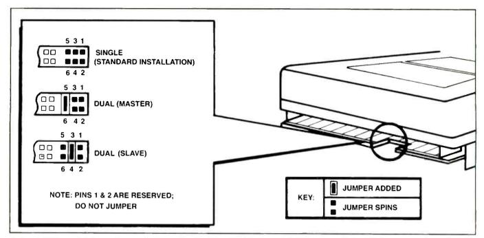
Figure 4. IDE hard disk drives do not have terminating resistor packs. However, a set of jumpers on the underside of the drive can be used to configure the drive as a master or slave. On a Western Digital Caviar drive, those jumpers are placed as shown here.
