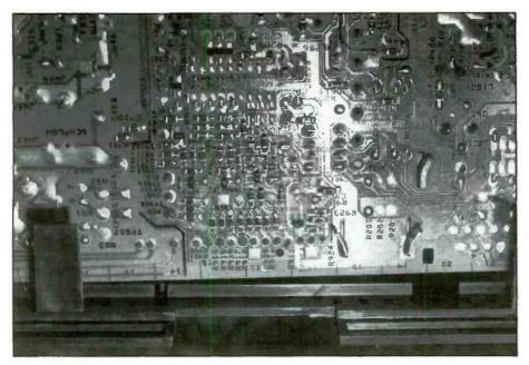
Figure 8. Look for fine SMD breaks and poor pc board connections when flexing the board chassis.
