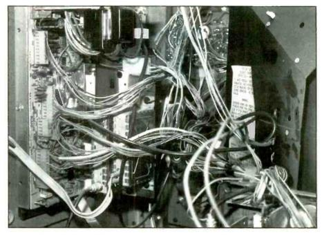
Figure 1. Poor crimped wires and plug connections may cause intermittent problems.
