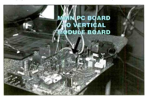
**Figure 5.** When the board module was probed the vertical raster would come and go in the Sharp TV portable.
