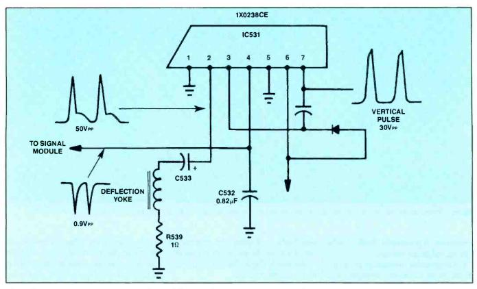
Figure 4. Intermittent vertical foldover in a Sharp 19SB60R portable was caused by a board connection of the signal board module.
