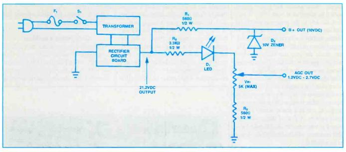
Figure 2. The schematic of this sample project tuner subber was built entirely from discarded parts found around the service center. Because the power supply is more or less typical, it is shown in block form, though the voltages pertinent to the project are indicated.
