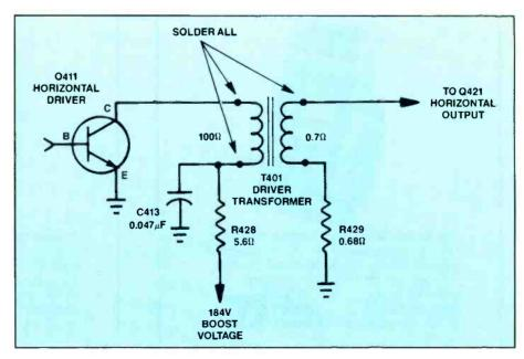
**Figure 2.** Solder the board connections when the problem is intermittent. The horizontal driver transformer in the horizontal circuits of this RCA GER654 model caused intermittent start up and shutdown.
