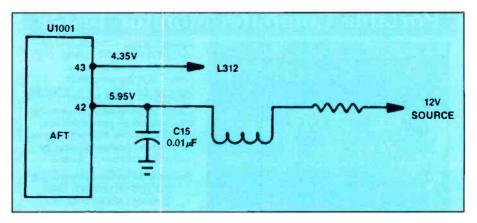
Figure 7. A poor connection in L312 caused the channels to change spontaneously in an RCA EXR345ER model.
