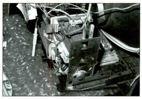
Figure 6. Suspect socket and harness connections when the problem is intermittent.
