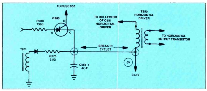
Figure 3. The no-raster, no-HV, no-sound problem was caused by a break in an eyelet at the pc wiring of a JC Penney 681-2018A model.
