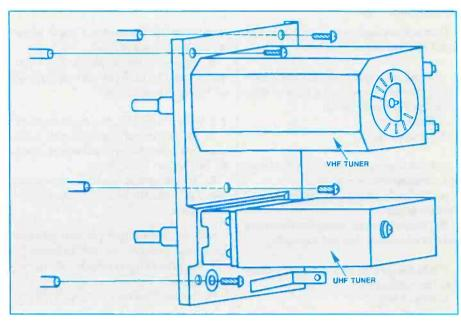
Figure 1. Many television sets have their tuners (both VHF and UHF) mounted on a single plastic or metal frame, which is, in turn, mounted inside the cabinet of the receiver.
