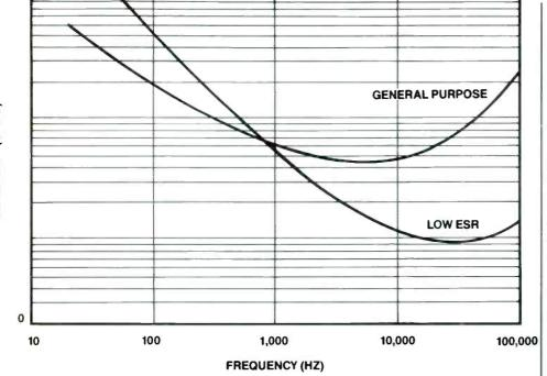
Figure 2. ESR is frequency dependent. If you viewed the frequency versus ESR graph chart of a low-ESR electrolytic you would find the ESR is biased so that the ESR is lower at high frequencies than it is at low frequencies.
