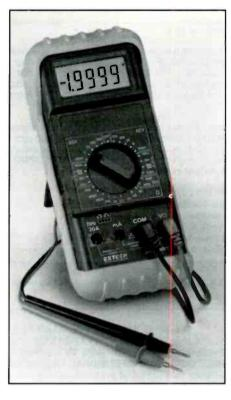
200mV to 750V, dc current and ac current in five ranges from 200µA to 20A, and resistance in seven ranges from  $20\Omega$ to  $20M\Omega$ . Basic de accuracy of 0.05%. Also includes audible continuity, diode, and transistor test. The large LCD readout reads up to 19,999 counts for resolution to  $10\mu V$ ,  $0.1\mu A$  and  $0.01\Omega$ . Also indicates function, polarity, low battery and overload. Fuse protected. Comes complete with test leads, rubber protective holster, and 9V battery.
