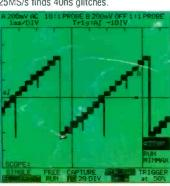
8:23 AM, Security Monitor not working. 3-1/2-digit DMM indicates bad ground.
