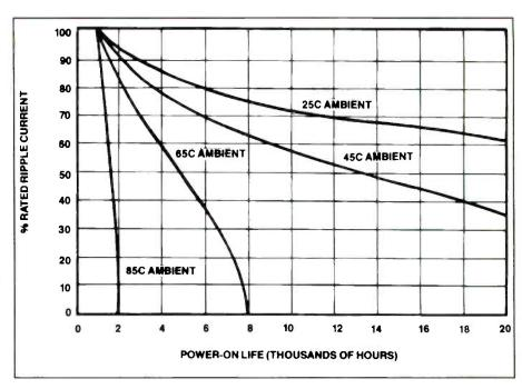
**Figure 1.** The operating life of an electrolytic capacitor depends on the temperature to which it is subjected. This temperature must be 30 degrees below its maximum temperature rating in order for it to operate reliably for five years during moderate use. If operated at 40 degrees below its maximum temperature, its lifetime would be 10 years. Other things being equal, your replacement must have at least the same maximum temperature rating as the defective part.
