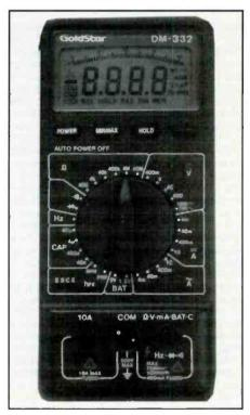
transistor check, frequency counters, min/max hold, relative, bargraph, etc.
