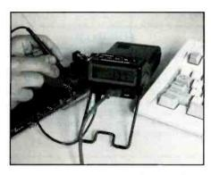
ature measurement capabilities include twelve °C/°F ranges from -200C to +1372C (-328F to +2500F) with 0.1C resolution to +1000C.
