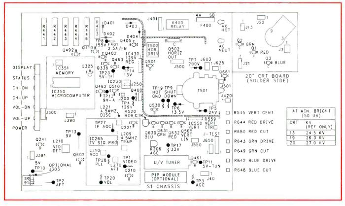
Figure 3. This layout shows where the various components are located on the S1/S4 chassis.
