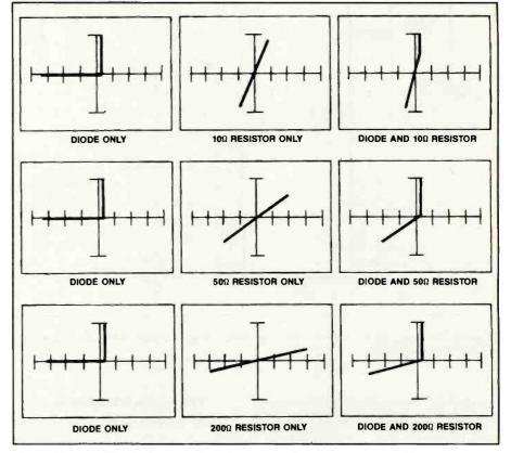
Figure 48. A 1N4001 diode in parallel with various value resistors yields different signatures. When the resistor is over  $1k\Omega$  it contributes very little to the signature: the signature mainly shows the effect of the diode.
