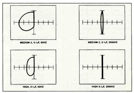
Figure 49. A 50k  $\Omega$  resistor in parallel with a 0.1  $\mu F$  capacitor yields this signature.
