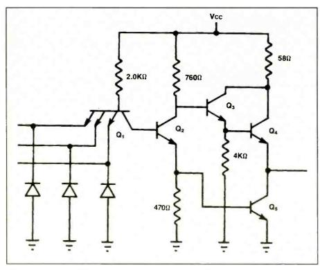
Figure 51. A typical TTL (transistor-transistor logic) gate. These gates are similar in that they have an input gate, phase shifter, (Q2) with emitter and collector load resistors, a pull- up mechanism (Q3/Q4) and a pull-down transistor (Q5).
