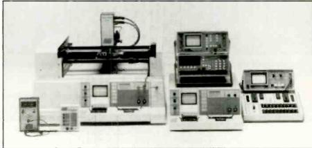
Figure 57. This family of trackers, in combination with an IBM or compatible computer, can digitally store device signatures for future troubleshooting.
