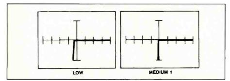
Figure 53. The signature between the  $V_{CC}$  pin and ground of a 7410 TTL triple three-input NAND gate at 60HZ.
