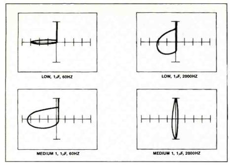
Figure 50. The signature of a  $1k\Omega$  resistor in parallel with a  $1\mu$ F capacitor.
