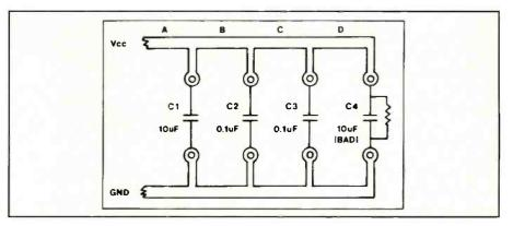
Figure 55. The shorted capacitor of these four paralleled capacitors will draw the most current, more than the other three non-shorted capacitors, thus allowing the user of the short circuit tracker to find the bad capacitor.
