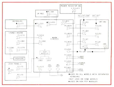
Figure 2. This simplified wiring diagram shows how the various portions of the S1/S4 sets are connected together.
