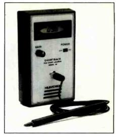
Figure 54. The Shortrack allows the user to probe a PC board to determine where current falls off, and therefore where there is a short circuit.
