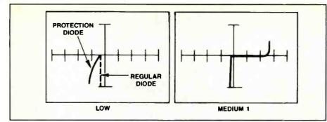
Figure 52. The signature between the input pin and ground of a 7410 TTL triple three-input NAND gate at 60Hz.
