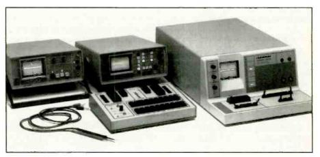
Figure 58. The instrument on the far right provides the capability to handle 64-, 40-, and 20-pin IDC connector sockets. It has a 40-pin ZIF (zero insertion force) socket built in, and an IEEE-488 interface.
