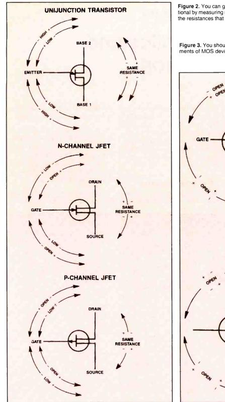
Figure 2. You can get an idea if a unijunction transistor or JFET is operational by measuring resistances between elements. These drawings show the resistances that you will measure if the unit is functioning properly.
