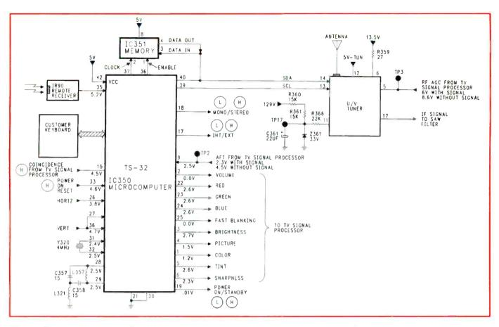
Figure 5. The tuning system in this TV set, as in many modern products, contains a microcomputer, with its attendant memory, to provide a wealth of functions electronically.
