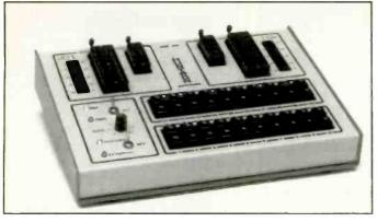
Figure 56. A. A switcher allows a technician to compare the signature of a device against that of a known-good device of the same type. This is a manual switcher. B. An automated switcher, shown here below an analog signature analyzer, allows the switching to be done automatically.
