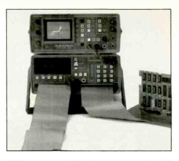
This device has dual inputs so it routes signals from a known good part and the suspected bad part to a signature analyzer. All you do is attach a clip to the IC being tested and use the switcher's 40 push buttons to display the signature at each of up to 40 pins. You can even customize the cable with special edge connectors or interface devices.
