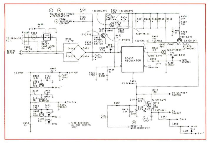
Figure 4. The power supply of the S1/S4 chassis employs a full-wave bridge rectifier, filtering capacitors, and a voltage regulator IC (IC430) which injects 155Vdc into the system. These chassis incorporate a "standby" circuit which is activated when the set is turned off.
