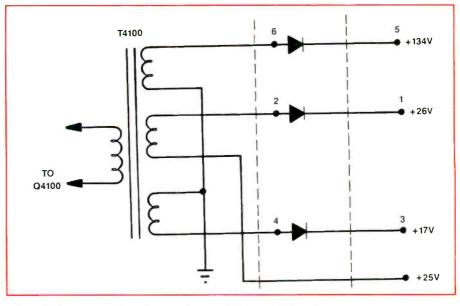
Figure 6. Solder each diode terminal to correct the intermittent off/on problem.
