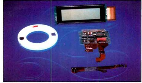
Figure 1. 3M's Z-Axis Adhesive Film (ZAF) is a new concept in connecting flexible printed circuits and Tape Automated Bonding (TAB) circuits to printed circuit boards, glass substrates, and other flex circuits.
