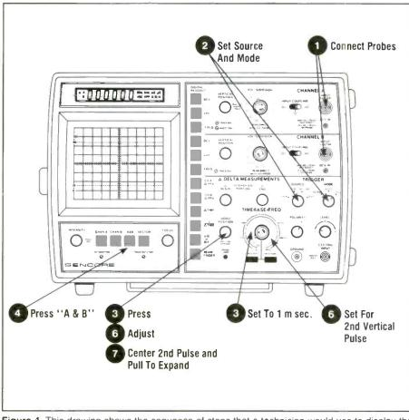
Figure 4. This drawing shows the sequence of steps that a technician would use to display the head-switching signal on the Sencore Waveform Analyzer.
