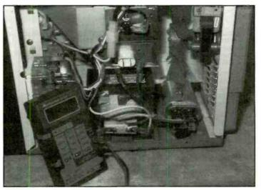
Figure 5. Do not use a small DMM or VOM to measure high voltage in the microwave oven. Use the DMM only for continuity and resistance measurements.
