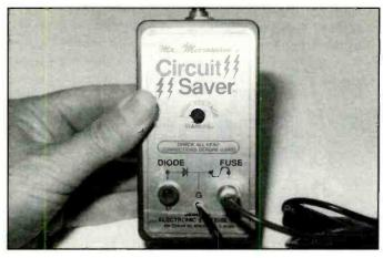
**Figure 9.** When the microwave oven keeps blowing the fuse, clip the Circuit Saver across the fuse holder and just reset the circuit breaker, instead of replacing those expensive chemical fuses each time.
