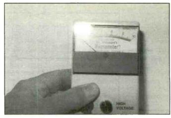
Figure 7. The Magnameter has a yellow area up to 2kV, a green area from 2kV to 4.5kV, and a red area from 4.5kV to 10kV.
