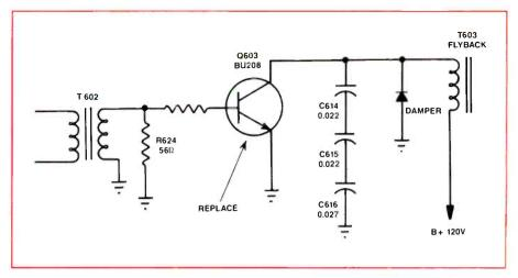
Figure 4. The leaky BU208 horizontal output transistor was replaced with a GE-38 universal replacement.
