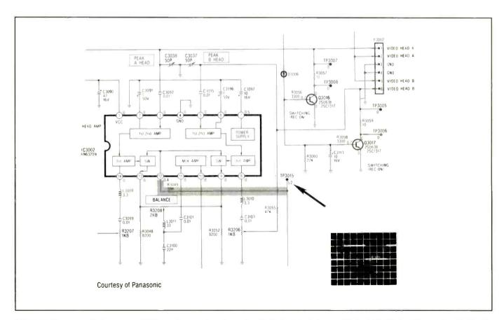
Figure 1. The head switcher uses a 30Hz square wave from the servo circuits to turn off the amplifiers of the head which is not contacting the tape.
