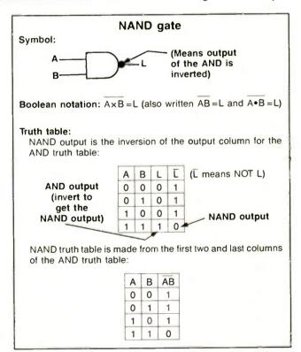
Figure 2. The NAND gate is obtained by inverting the output of an AND gate.
