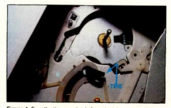
Figure 4. Free the tire completely from the idler so it is sitting on top of the idler wheel. Slip the idler tire through the top of the chassis.
