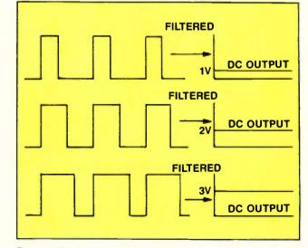
Figure 4. The digital circuit outputs a pulse train that, when filtered or averaged into a dc voltage, creates an analog dc voltage. The dc voltages are then amplified to the required magnitudes by dc voltage amplifiers.
