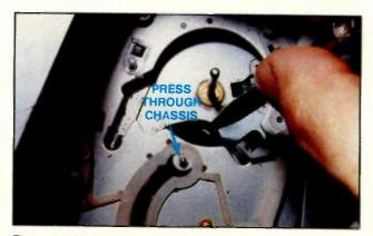
Figure 3. With the idler almost all the way to the right, gently press it through the chassis. Roll the tire free from the idler wheel, then grab it with a parts picker held in the right hand.
