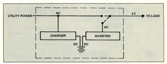
Figure 1. The off-line UPS is usually inexpensive and lightweight, but it does have some disadvantages: it causes a switching glitch of 5ms to 20ms; it has no line conditioning or regulation; it can be "fooled" by brownouts and frequency shifts; it usually doesn't have sine-wave output; and its switching time can triple during brownouts.
