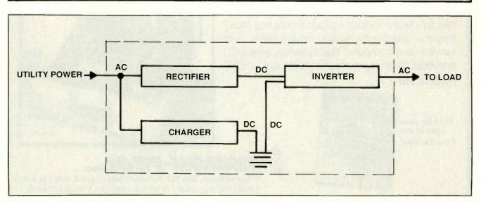
Figure 3. The on-line UPS offers no switching, 100% line condition and regulation, sustained brownout protection and sine-wave output. However, it is usually more expensive, larger and heavier. The unit's inverter powers 100% of the load at all times.
