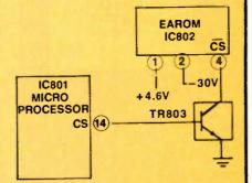
Figure C. This schematic drawing of the timer board that controls the tuner functions shows IC801, the control microprocessor, and IC802, an EAROM.
