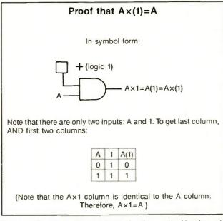
Figure 5. Circuits can be used for proving these rules. Use the truthtable method.
