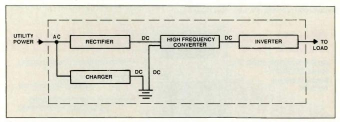
Figure 6. Newer generation UPS systems provide on-line topology with a sine-wave output generated by a high-frequency, PWM inverter. A low-impedance filter replaces the output transformer. These units can be smaller, lighter and nearly the same price as off-line and hybrid systems.
