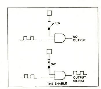
Figure 6. In Figure 5, if you put a switch in series with the lead to logic 1, the circuit becomes an ENABLE. When the switch is open, no signal passes through (A AND 0 = 0). With the switch closed, the output signal is the same as the input signal (A AND 1 = A).
