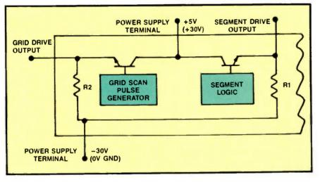
Figure 2. Two different biasing schemes for display driver ICs are in common use. The most popular type uses a high negative voltage supply. The other uses a high positive voltage supply.
