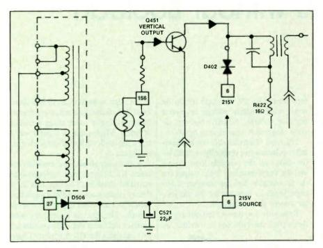
**Figure 1.** An open R422 suggested excessive current might have caused a vertical deflection problem. Although the vertical output transistor, Q451, checked out OK, replacement brought the TV back in operation.
