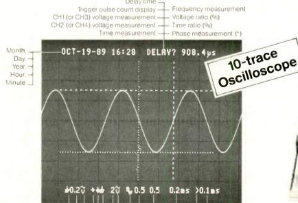
CH1 grounded Sweep time (B) setting value A (or B) sweep variable CH1 UNCAL condition (UNCAL condition) CH1 attenuator Sweep time (A) CH1 attenuator units CH4 attenuator setting value ADD (CH1 + CH2) CH3 attenuator setting value CH2 inverted CH2 grounded BWL mode selected CH2 attenuator units CH2 UNCAL CH2 attenuator
