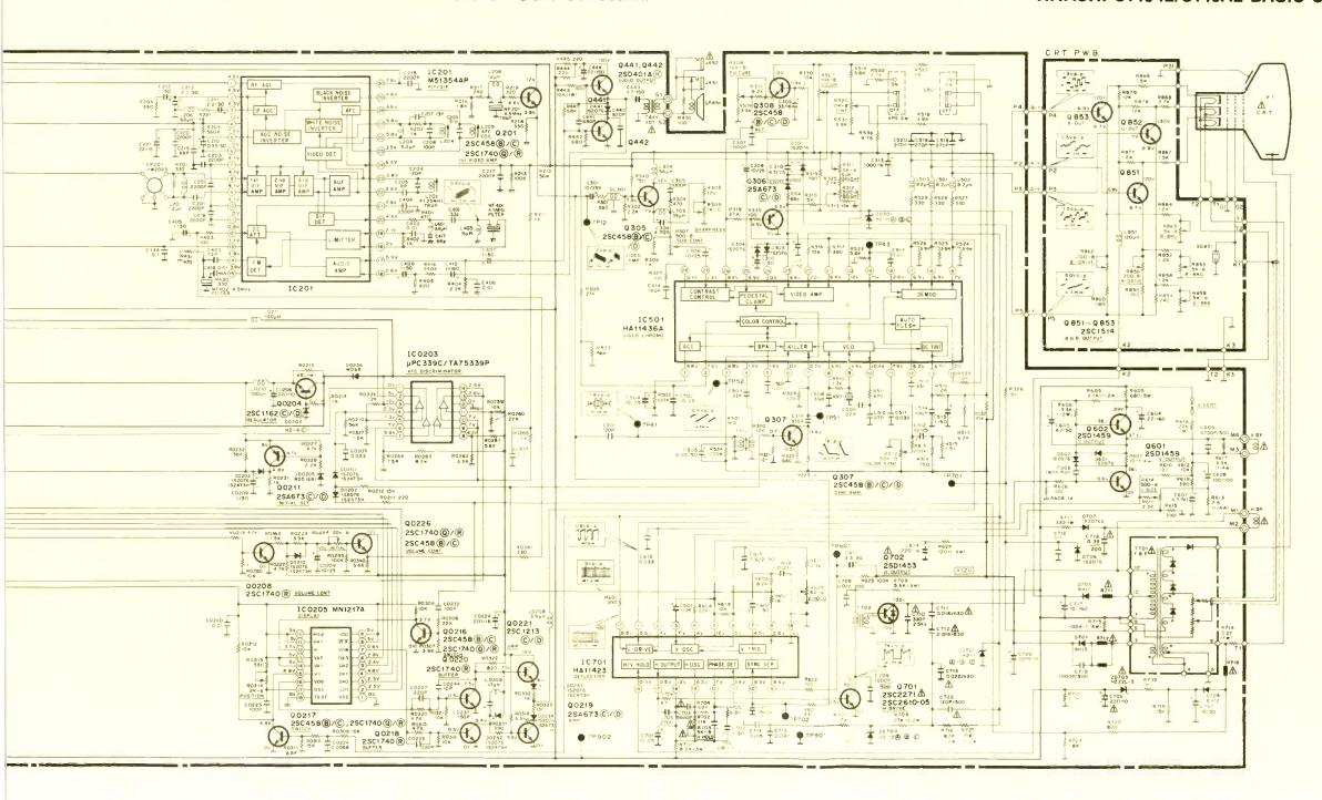
Product safety should be considered when component replacement is made in any area of a receiver. Components marked with a ! and shaded areas of the schematic diagram designate sites where safety is of special significance. It is recommended that only exact cataloged parts be used for replacement of these components.
