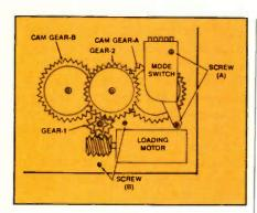
Figure 1. To remove the mode switch assembly, first disconnect the DS and DQ plugs from the assembly. Then remove the two mounting screws (A), and the mode switch.
