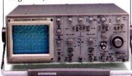
Model 9106, 60MHz, 3 Channel, Dual Sweep (A & B).
