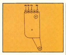
Figure 4. The mode switch on the HS-430UR is a 6-position rotary switch that informs the mechanical control microprocessor as to the current status of the tape-transport mechanism.
