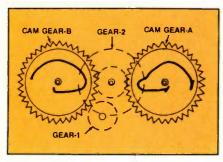
Figure 2. To set the loading mechanism to the eject position, you need to remove the two loading motor mounting screws (B in Figure 1), then move the loading motor away from gear 1. Manually rotate gear 2 counterclockwise until a stop is reached. Finally, reposition the loading motor and install mounting screws (B). This figure illustrates the position of the cam gears in the eject position.
