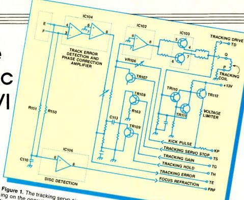
Figure 1. The tracking servo circuit uses a number of ICs and various transistors. Depending on the operation mode selected tracking servo control is achieved by making certain Figure 1. The tracking servo circuit uses a number of ICs and various transistors. Depending on the operation mode selected, tracking servo control is achieved by making certain
