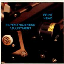
Figure 1. If the printer is printing light even after you have changed the ribbon, check the setting of the paper-thickness adjustment lever (to the left) before replacing the print head (to the right). This printer is the Star SG-10, similar in construction to the NX-10.
