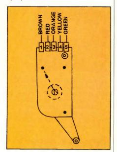
Figure 3. One of the first steps in installing the mode switch assembly is to manually rotate the gear on the mode switch until the pointer on the bottom of the gear shaft points to the black plastic guide.
