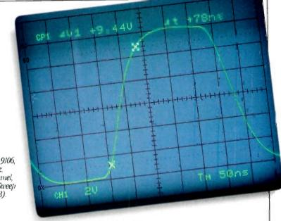
Five of six models feature two independently-adjustable time bases. Built-in intensity modulation allows you to select a small section of a main waveform for closer examination. This feature is ideal for measuring pulse rise times or checking sync pulse amplitudes in composite video signals.
