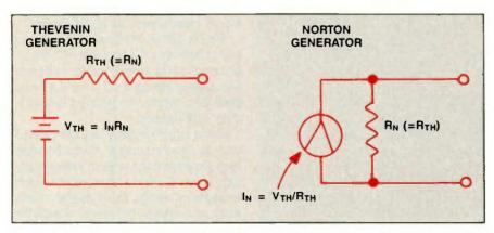
**Figure 3.** If the Thevenin circuit and the Norton circuit are both equal to the same active 2-terminal, then it follows that they are related to each other. The relationship is simply Ohm's law:  $I_n = V_{th}/R_{th}$  where  $R_{th} = R_{n}$ .
