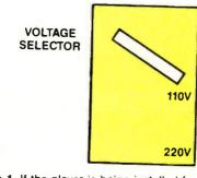
Figure 1. If the player is being installed for the first time, check to make sure it is meeting its power input requirements. Some players have a switch to permit the unit to be operated by different line voltages. Check the switch to make sure it is set to its correct position for the line voltage in your area.
