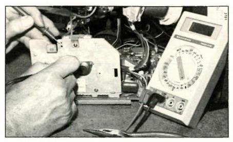
In a CT-330M Samsung portable, leakage of the STR-382 voltage regulator was located with a DMM's diode-junction test. Replacement of the defective regulator with a STR-382 original part number IC completed the repair.
