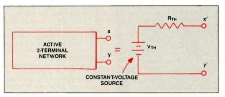
Figure 1. Any 2-terminal active network can be replaced by a Thevenin generator. It doesn't matter how many sources of voltage are in the 2-terminal circuit. (There must be at least one.) It also doesn't matter how many resistors and battery internal resistances are in the circuit.
