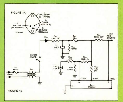
**Figure 1.**  $O_{801}$ , the B+ IC regulator of the Samsung CT-333KA portable, has the physical appearance of a horizontal-output transistor, except it has three terminals, not the usual two (Figure 1A). However, the STR-382 IC probably contains diodes, transistors and resistors in addition to the power transistor. A B+ adjustment control or an external voltage-stabilizing zener diode is not required, according to the Figure 1B schematic.
