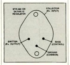
Figure 5. Not all good test-points of a voltageregulating IC are brought out to terminals. Therefore, many tests are not possible from the outside terminals. Fortunately, only three of the possible tests are often sufficient to prove whether the out-of-circuit IC is defective.
