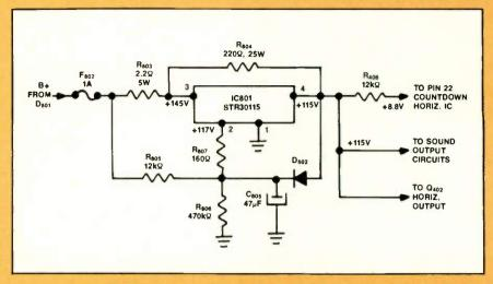
**Figure 3.** Regulated output voltage of +115V from IC<sub>801</sub> (STR-30115) provides voltage for the sound and horizontal circuits. During start-up, +8.8V for the horizontal countdown IC pin 22 is brought through  $R_{406}$  from the +115V supply. Troubleshooting circuits that have IC voltage regulators is very similar to troubleshooting others without ICs except that several components are not available for testing, and terminal-to-terminal IC tests show unusual readings.
