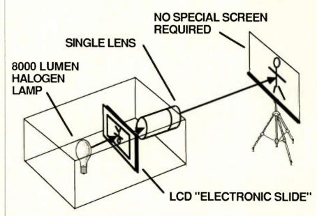
Figure 1. The portable color projection TV uses an 8,000 lumen halogen lamp and a single lens to achieve a high-resolution image without complicated optics or convergence.
