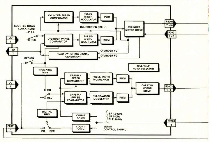
correct. The speed at which the tape is fed past the heads must also be correct, so signals recorded on the tape during record are fed to the capstan along with video-head speed and position information during playback to keep the video heads tracking accurately over the video tracks.
