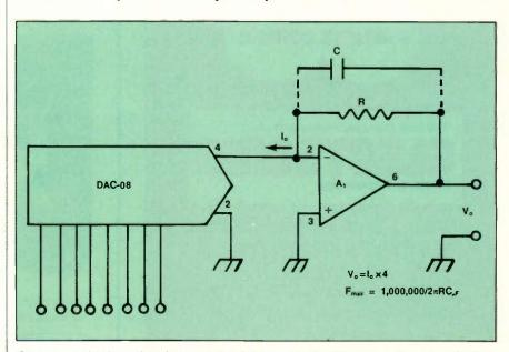
Figure 1. A simple method for converting  $I_0$  to an output voltage (V<sub>0</sub>) with a low output impedance (less than 100 $\Omega$ ) is to use an inverting follower operational amplifier. The output voltage is simply the product of the output current and the negative feedback resistor:  $V_0 = R \times I_0$ .
