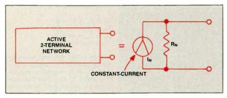
Figure 2. Like the Thevenin generator, the Norton generator can be used to replace any 2-terminal active network. It uses a constant-current generator and a single resistor.
