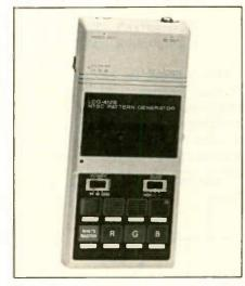
weighs less than 14 ounces, including six AA power cells, and features 75% color bars, dot, crosshatch and full raster signals of 100% white, red, green and blue. The unit features RF output on U.S. broadcast VHF and UHF channels in addition to  $1V_{p-p}$  video output into a 75 $\Omega$  load.
