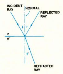
Figure 1. When light waves strike the boundary between two mediums, the rays are either refracted, or passed through the surface, or they are reflected back.
