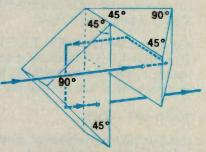
Although rarely used in TV optics, the double Porro prism with 45°-45°-90° angles allows realignment of light for easier viewing in high-quality binoculars.
