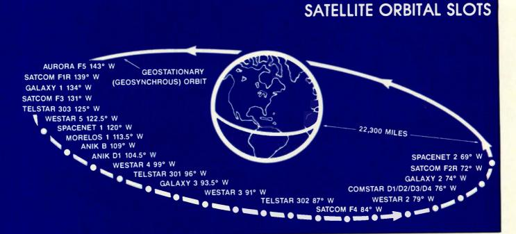
Figure 1. All of the domestic television satellites are located in an orbit directly about the earth's equator between 69° west longitude and 143° west longitude. Because their orbital speed just matches the rotational speed of the earth, each one is, in effect, stationary above a point on the earth.
