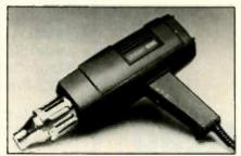
ounce gun reflows solder, loosens adhesives, applies heat-shrinkable materials, cures epoxy, heats liquids, shapes plastics and more. It has a heat-concentrating nozzle with stainless steel shielding, a permanent magnet motor and a reinforced, mica-insulated heating element.
