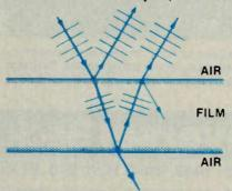
The angle of incidence is equal to the angle of reflectance, both measured from the normal, which is a line meeting the reflecting surface at an angle of 90°.
