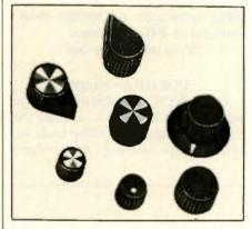
Mil-spec knobs, which are made of polycarbonate, are manufactured in 26 variations of the five most widely used styles and are available in 0.125 and 0.250 diameters. The commercial knobs, made of ABS thermoplastic with spun aluminum inlays, are available in 32 variations of the six most popular styles and come in 0.125 and 0.150 shaft diameters.
