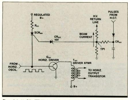
**Figure 3.** In this RCA CTC126 chassis, the overcurrent shutdown transistor and the overvoltage latch transistors shown in Figure 2 are missing. However, in both chassis, the horizontal deflection system is shut down by cutting off the drive to the horizontal output stage, in response to either overvoltage or overcurrent conditions. The 2-transistor latch has been replaced by a thyristor (SCR<sub>401</sub>) with a 10V zener diode (CR<sub>402</sub>) in its gate circuit.
