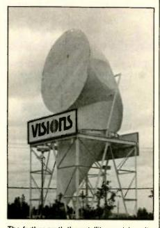
The farther north the satellite receiving site is, the lower the *look angle*. In Anchorage, Alaska, where the look angle is just above the horizon, ground clutter noise could be significant if an ordinary dish-type reflector is used. A highly directional antenna works better in this situation.
