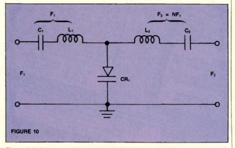
**Figure 10.** In this varactor tripler circuit, the input circuit is tuned to the input (fundamental) frequency by either an LC-tuned tank circuit or a micro-strip line. The output is similarly tuned but to a harmonic (N x  $F_1$ ) of the input frequency.
