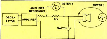
Figure 1. At a given frequency, you close the switch and adjust the amplifier controls for a 10V reading at meter 1. A voltage of 10V across the 1kQ resistor means that the current through it is 10mA. The second step is to open the switch and read the voltage across the speaker inputs. This voltage is caused by the 10mA of current through the speaker. The impedance of the speaker at that frequency will be the meter voltage divided by the current.
