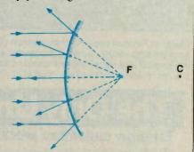
A concave mirror causes light waves to be reflected and converged at a focal point in front of the mirror.
