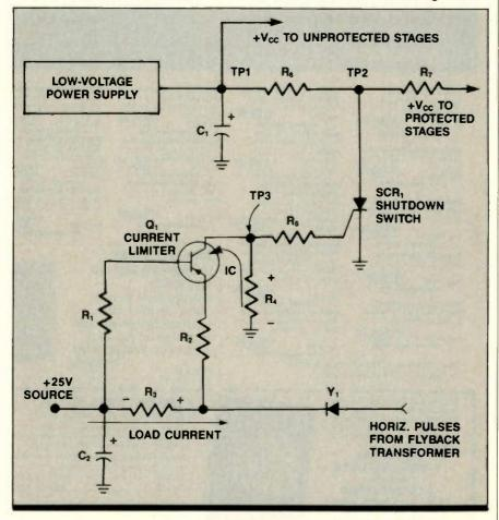
Figure 1. One way of providing shutdown protection is to incorporate a circuit that, under certain fault conditions, can reduce or completely kill the B+ ( $V_{cc}$ ) applied to vital stages, thus reducing or removing the power available to those stages so that overheating or excessively high voltage will not occur.
