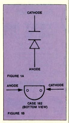
Flaure 1. Figure 1A shows the usual circuit symbol for varactors. In some cases, the "capacitor" at the top end of the "diode" symbol has an arrow through it to denote variable capacitance. Varactors come in several different standard diode packages, including the 2-terminal "sorta-like-transistor" Type 182 package shown in Figure 1B.
