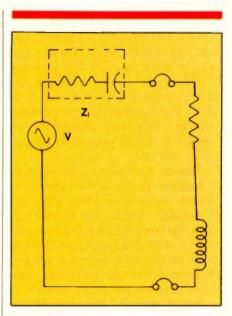
Figure 3. In the case of an ac circuit with a capacitive internal impedance, in order to transfer the maximum power to the outside world, make the load resistance equal to the internal resistance and use an inductance to resonate with the internal capacitance so that you have a series resonant circuit.
