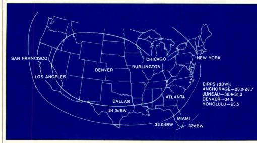
Figure 2. Effective isotropic radiated power (EIRP) is a measure of the relative strength of the satellite TV signal expressed in dBW. This footprint map graphically illustrates how strong the satellite signal is as it reaches various regions of the satellite's coverage area. Each satellite has a different coverage pattern. In many cases, different transponders on the same satellite will show a different EIRP. Where the signal is strongest is the area referred to as the boresight.
