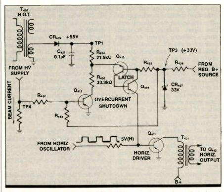
Figure 2. The protection circultry in this RCA CTC108 chassis schematic disables the horizontal deflection system by cutting off the horizontal drive if either high voltage or beam current increases beyond certain limits. Transistors  $Q_{413}$  and  $Q_{414}$  form an x-ray protection latch, and transistor  $Q_{415}$  senses excessive CRT beam current.
