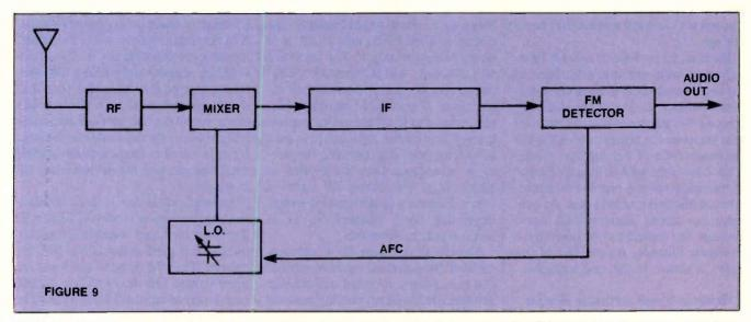
Figure 9. The varactor-tuned variable frequency oscillator is used as the LO in FM receivers. The FM detector produces an error voltage that indicates how far off center the tuning is and feeds it back via the automatic frequency control (AFC) line to the tuning voltage input on the tuner. The AFC voltage drives the LO operating frequency to the center-tune condition.
