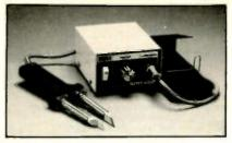
SMT-W2 SMD REMOVAL SYSTEM O.K. Industries introduces the SMT-W2, a hand-operated SMD removal tool. Featuring a variable temperature controller, tweezer-action handpiece, handpiece stand, and a wide variety of optional tips, the system affords an effective low-cost solution for SMD removal. The SMT-W2 tips have a high thermal capacity to support removal of the most demanding components. Dual 80W ceranic heating elements provide rapid heat recovery and
