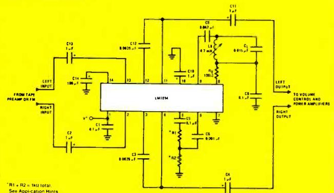
FIGURE 1. Component Hook-Up for Stereo DNR™ System
