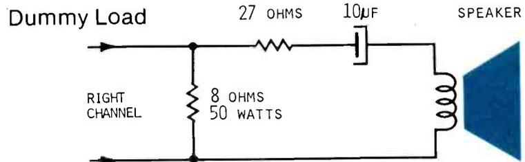
**Figure 4** Because the right-channel amplifier emitted 50V pulses of dc voltage when the erratic noise and amplification occurred, this dummy load was connected to the output. The series resistor and capacitor reduces the ac and steady dc current through the speaker to prevent ruining another test speaker.
