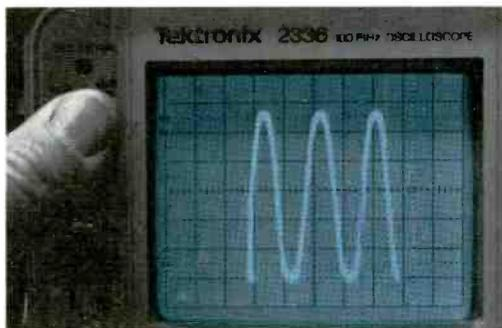
**Off-the-screen waveforms** can be identified by pressing the beamfinder switch button, which compresses the waveform, including both ac and dc components.
