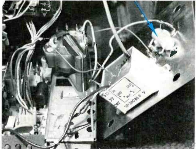
rent through the 4-wire capacitor (as is done in most other models). Instead, the cold end of the T800 base-drive transformer winding returns to the Q100 output-transistor emitter through two capacitor wires. An open circuit between those two wires would greatly reduce the amplitude of drive signal to the Q100 base, decreasing the high voltage, and probably giving center foldover as well.
