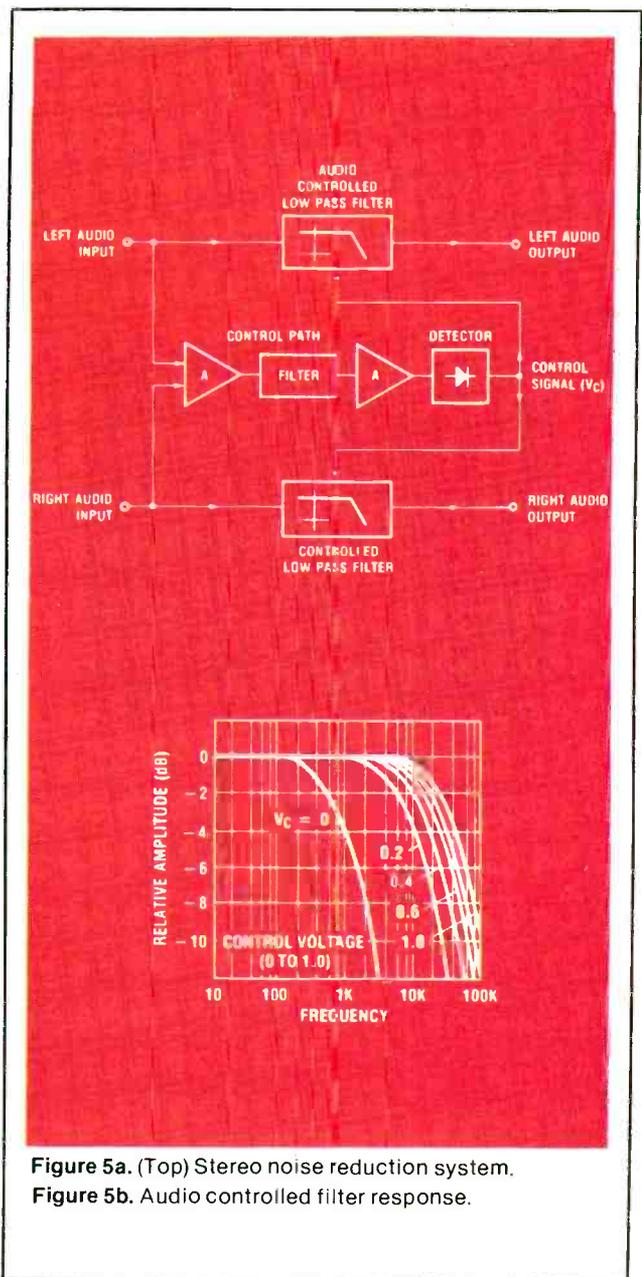
Figure 5a. (Top) Stereo noise reduction system.
