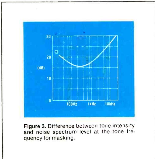
**Figure 3.** Difference between tone intensity and noise spectrum level at the tone frequency for masking.
