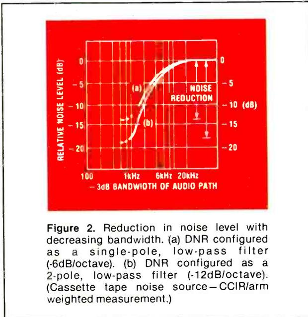
**Figure 2.** Reduction in noise level with decreasing bandwidth. (a) DNR configured as a single-pole, low-pass filter (-6dB/octave). (b) DNR configured as a 2-pole, low-pass filter (-12dB/octave). (Cassette tape noise source - CCIR/arm weighted measurement.)
