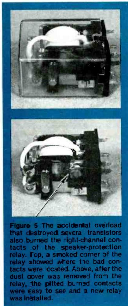
**Figure 5** The accidental overload that destroyed several transistors also burned the right-channel contacts of the speaker-protection relay. Top, a smoked corner of the relay showed where the bad contacts were coated. Above, after the dust cover was removed from the relay, the pitted burned contacts were easy to see and a new relay was installed.
