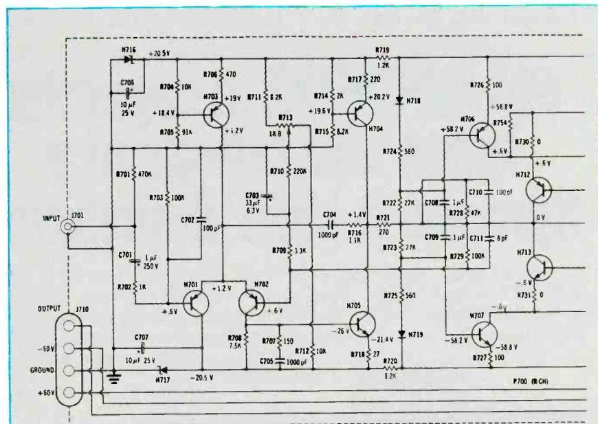
**Figure 2** This is the complete schematic for the right-channel audio amplifier in the 2325 Marantz. In the seven direct-coupled stages, only 10 transistors directly handle the signal and contribute to the voltage and power gains. The other nine are there for thermal and voltage stability. Because of the large number of direct-coupled stages, defects that affect dc voltages are difficult to identify.
