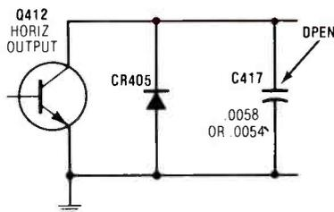
**Symptom** – Narrow picture with foldover and excessive high voltage
