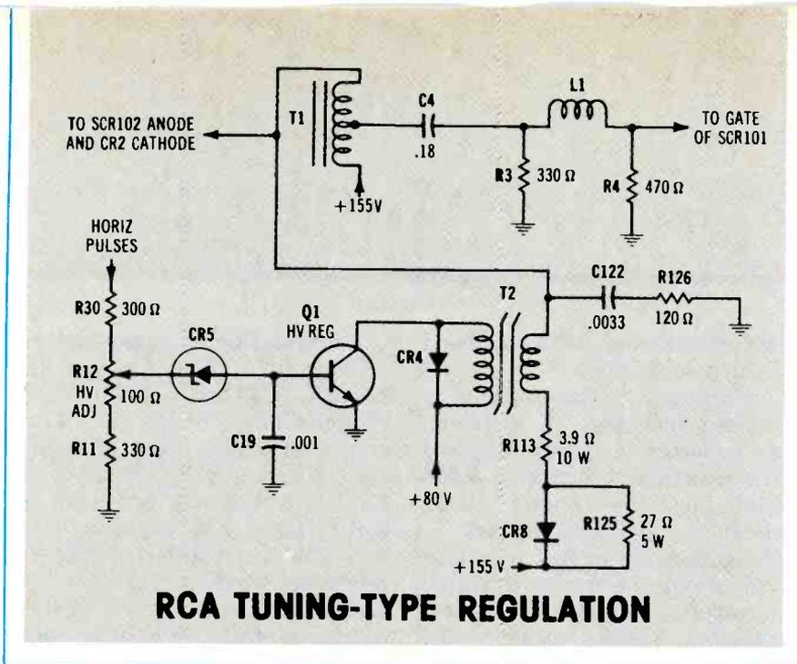
**Figure 2** High-voltage regulation in RCA receivers that have trace and retrace SCRs is accomplished by Q1 collector current which varies the T2 secondary-winding inductance. The inductance is tuned primarily by C122, so the varying inductance changes the resonant point. In turn, the varying resonant point changes the SCR102 anode voltage. SCR102 anode voltage when conduction begins determines the horizontal power and high voltage.
