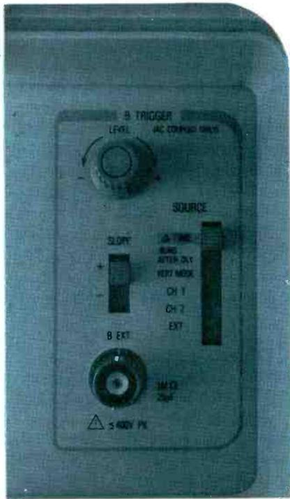
**Figure 7** Inside the hinged front cover in model 2336 are the controls for an external B-trigger function (above) and a sliding switch that can select B-triggering or delta-time functions. Located farther to the left (below) is the LCD digital readout that shows the time between intensified zones during the delta-time measurements.
