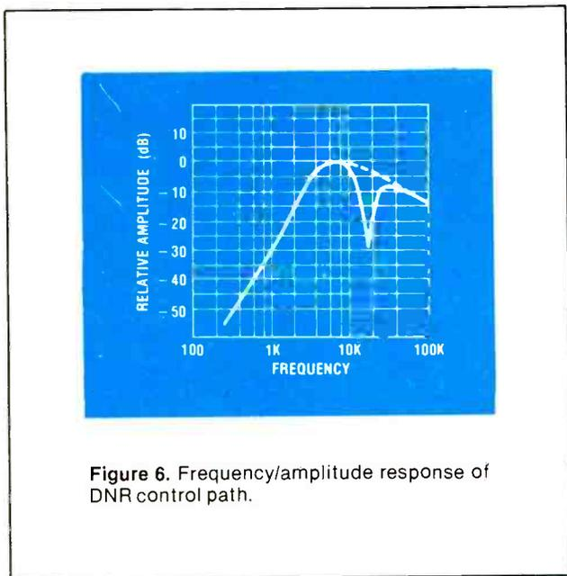
Figure 6. Frequency/amplitude response of DNR control path.
