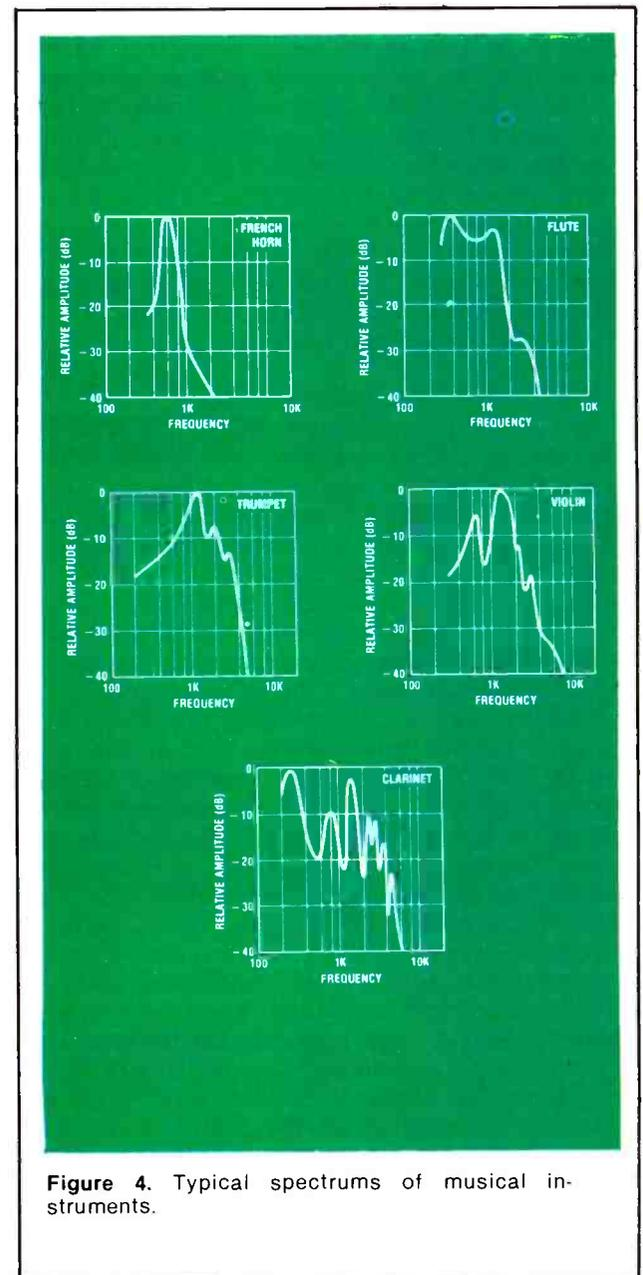
Figure 4. Typical spectrums of musical instruments.
