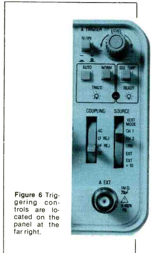
Figure 6 Triggering controls are located on the panel at the far right.
