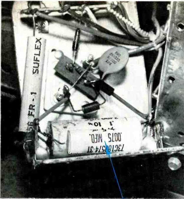
Figure 6 The arrow points to a 2-wire retrace-tuning capacitor in a color chassis (probably an older General Electric). These capacitors usually are connected in parallel with the damper diode.
