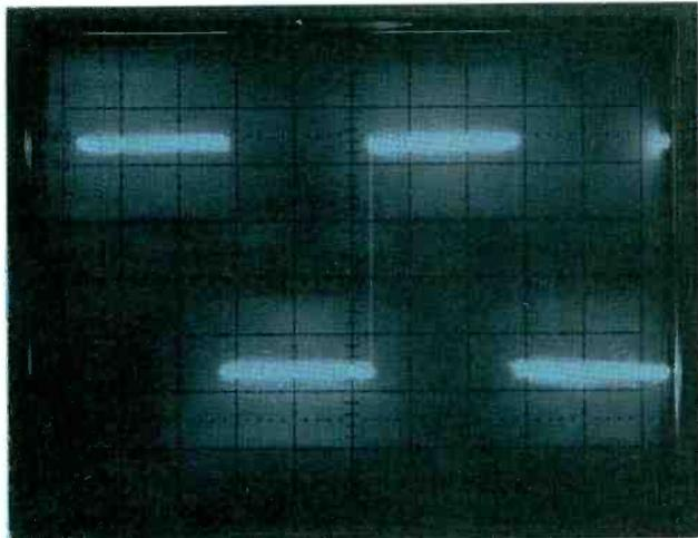
**Figure 8** These photographs show the probe-adjustment waveform without and with delta-time trace intensification. Above, in normal sweep mode, the horizontal sections of these square waves are very bright, while the fast rise and fall lines are dim. Below, delta-time trace intensification has brightened the square waves immediately following successive falling edges. Best accuracy was achieved here by moving each intensified area to the left until the falling edge *barely* was brightened.
