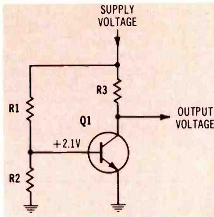
A non-defective diode is a good voltage regulator (within its wattage rating) because its forward-bias resistance varies rapidly with applied voltage across the junction. Of course, the B/E junction of a transistor has some characteristics of a diode.
