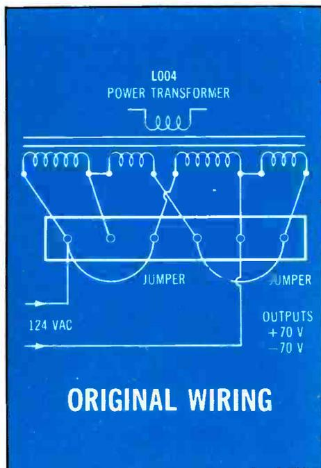
**Figure 8** The excessive supply voltages directed suspicion to the power-transformer wiring that had been changed from European voltages. The original wiring, left, had 124V applied to the 110V winding, and one 110V winding fed the other. Right, after rewiring, the 124V of shop line voltage was applied to both *total* 120V windings, with both sections properly powered from the line. The power transformer ran cooler, and the supply voltages were lower after the modification.
