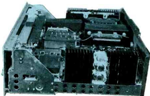
**Figure 1** The large fins of a cast heat sink identify the right-channel amplifier in the Marantz model 2325 AM/FM-stereo radio that also has inputs for a magnetic phonograph pickup and an external source such as a tape deck. Two PNP and two NPN power transistors are used in each audio channel. The accompanying circuitry is on a board fastened to the back side of the heat sink.
