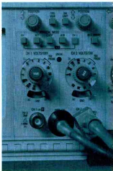
**Figure 4** Controls for the two identical vertical channels are located at the right of the screen. Notice the range marks for X1 and X10 probes near the volts/div switches. Two unusual push-buttons are supplied. The TRIG-VIEW button substitutes the triggering waveform for the signal waveform. The BW-LIMIT button restricts the bandwidth to about 20MHz. It is useful when unwanted high frequencies obscure desired low frequencies. One probe is shown plugged into the calibration jack.
