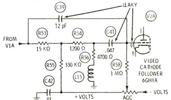
**Symptom**—Video blanks out, requiring adjustment of AGC
