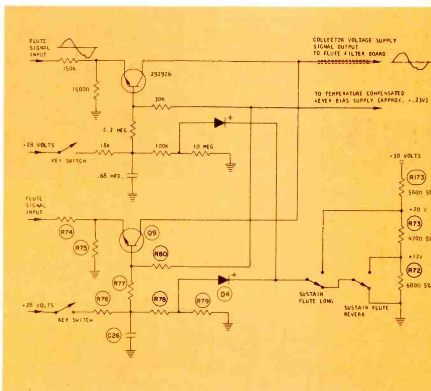
Fig. 8 The flute output from each Conn oscillator is keyed by changing the bias of a transistor, as shown. C26 delays the change of bias voltage to eliminate any clicks, and a fixed voltage through D4 determines the sustain time before the note dies away.
