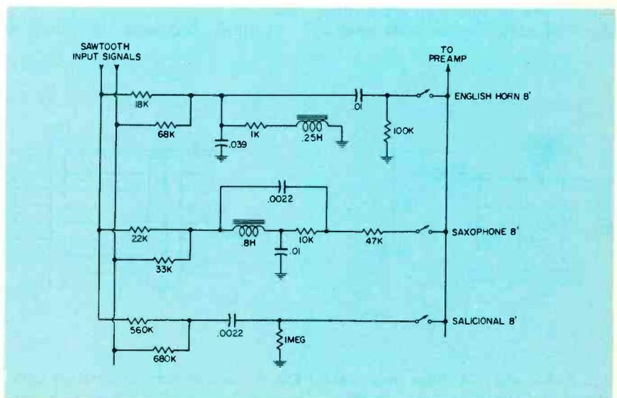
Fig. 4 These are examples of the stop filters used in some models of Baldwin organs.
