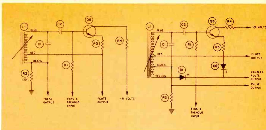
Fig. 7 These two examples of Conn oscillators show how two waveforms are obtained from one type, and three waveforms come from the top-octave type that has diodes acting as a doubler. These oscillators operate continuously. The pulse outputs are keyed directly as audio, while the flute outputs are keyed by transistors, with one transistor per note.
