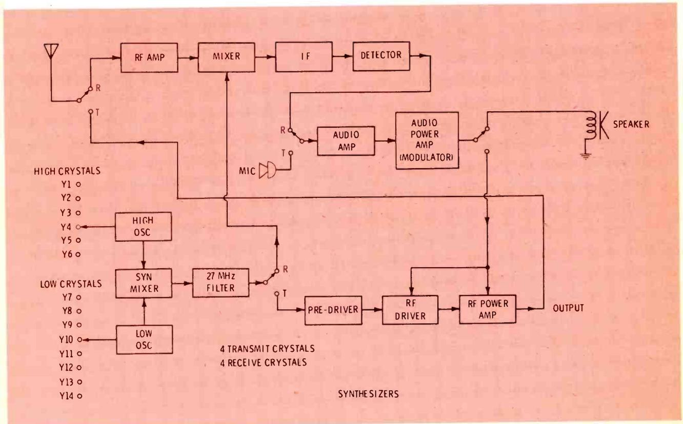
Fig. 3 This is the block diagram of a CB radio that has a synthesizer to furnish the oscillator signal for both receive and transmit functions. In the actual circuit, switching diodes take the place of the switches.
