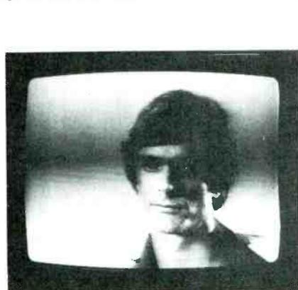
Fig. 9 Here are two examples of 60-Hz hum. Although the appearance can show in many different forms, two white or dark bars are produced by 120-Hz hum, and one white or dark bar is caused by 60-Hz hum.
