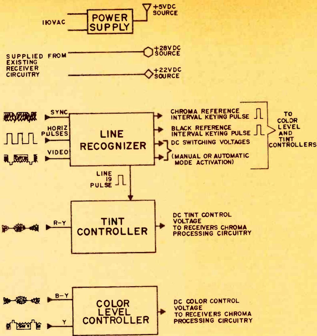
Fig. 3 Circuitry of the "Broadcast-Controlled" color feature can be classified into three areas: line recognizer and sensor of the VIR waveform, plus switching voltages for manual or automatic modes; tint controller; and color level controller.
