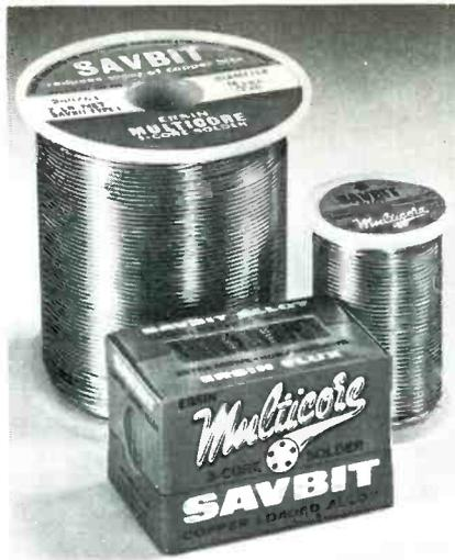
The new solder, called Savbit, is a copper-loaded, tin/lead alloy wire solder with 5 separate cores of rosin-base flux. Test results show it reduces the solution of copper by as much as 100 times.
