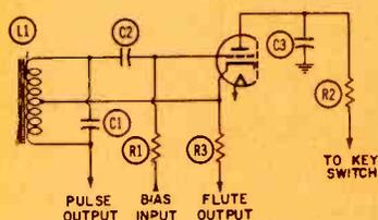
Fig. 5 R2 and C3 filter the plate voltage of Conn oscillators, to eliminate clicks, and to make the attack and decay times more natural.
