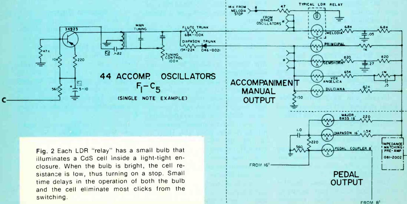
Fig. 2 Each LDR "relay" has a small bulb that illuminates a CdS cell inside a light-tight enclosure. When the bulb is bright, the cell resistance is low, thus turning on a stop. Small time delays in the operation of both the bulb and the cell eliminate most clicks from the switching.
