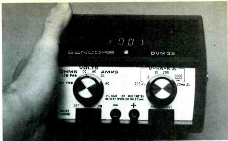
Fig. 5 Functions and accuracy of the DVM32 are similar to those of the DVM36, but there are separate knobs for function and range selection.
