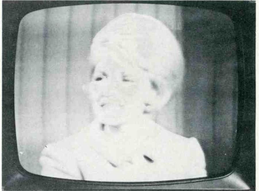
Fig. 3 Slow warmup and "sparkly" overload at high brightness and contrast characterize CRT with weak emission or gas. Focus may get bad as symptoms progress, but the main symptom usually annoys the viewer first.
