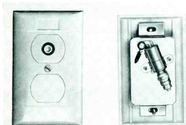
As the connector is withdrawn the house drop is terminated before the connection between the set and the drop is broken, preventing the generation of momentary standing-wave interference when the set is disconnected or moved to another outlet.
