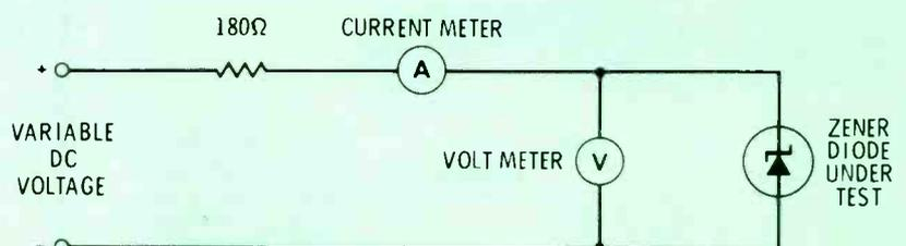
Fig. 1 Schematic of a circuit which can be used to test zener diodes by the voltage-current method.
