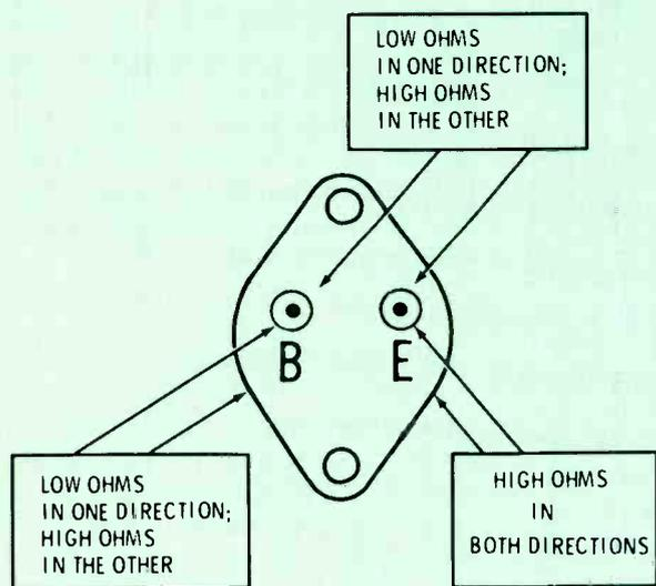
**Fig. 5** Checking power transistor with an ohmmeter identifies shorted junctions or open elements. This is a quick diagnosis tool.
