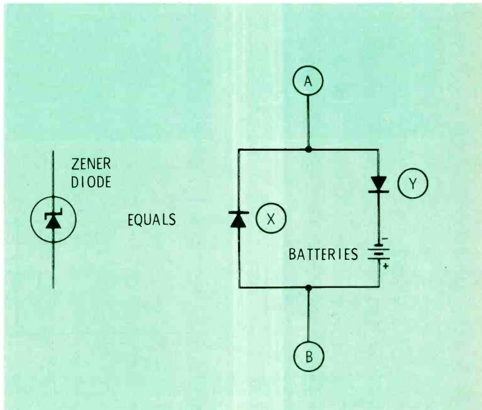
Fig. 3 A zener diode can be visualized as two rectifier diodes of opposite polarity connected in parallel, with a battery, used to provide a voltage delay, in series with one of them. Conduction can be obtained in either polarity, but at different voltages.
