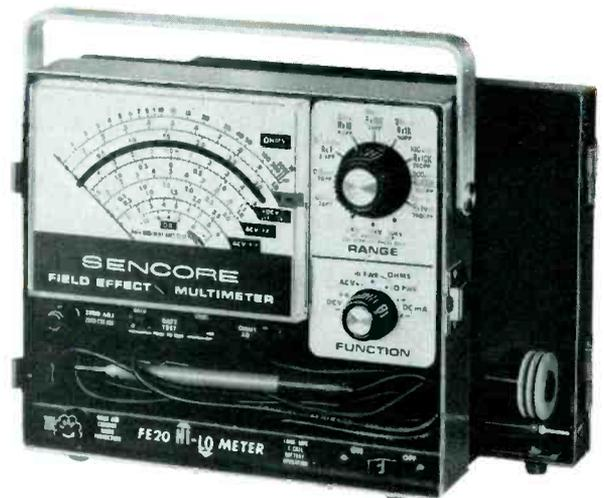
Fig. 1 Volt-ohm-milliammeters with field-effect transistors, such as those shown here, give all the bene-
