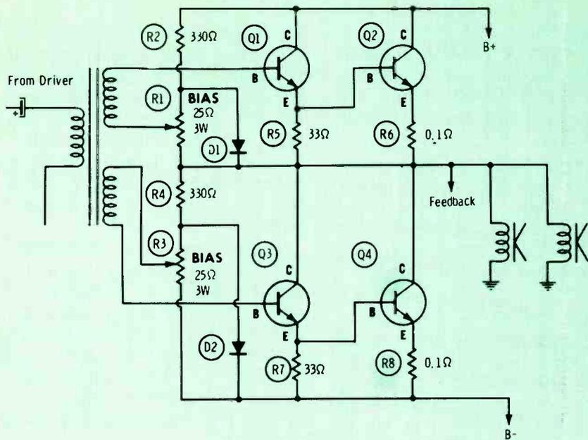
**Fig. 4** Four-transistor design boosts output power even higher. Transistors are all NPN, but because they are driven by a special transformer they operate push-pull. The output is transformerless.
