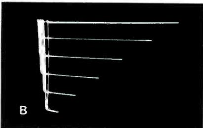
**Fig. 6** If you can find two transistors whose characteristic-curve traces coincide, you can be assured they match dynamically. Traces shown here were produced by A) a 2N411 PNP germanium and B) a small NPN silicon.
