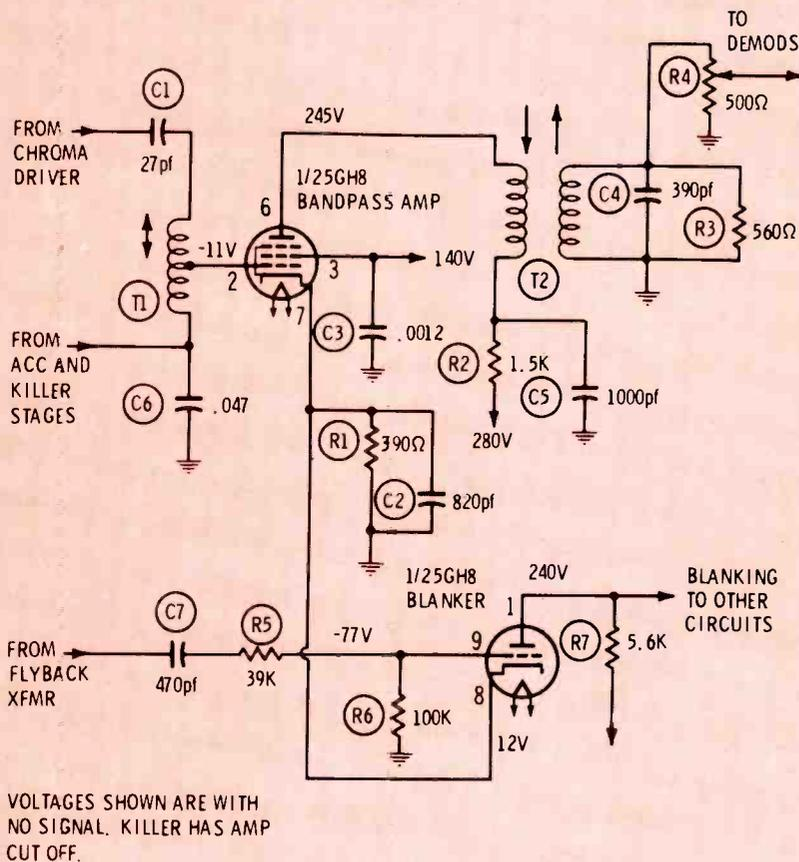
Fig. 2 Bandpass amplifier showing how the blanker applies its pulses to the cathode. Of equal importance in troubleshooting is the DC from ACC and color-killer stages.
