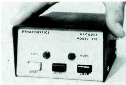
Frequency stability of the Model 201 reportedly is  $\pm 0.25$  percent for temperatures from  $-25$  degrees C to  $\pm 85$  degrees C. The input impedance is greater than 1 megohm, and operating time is 250 milliseconds or less, according to the manufacturer.
