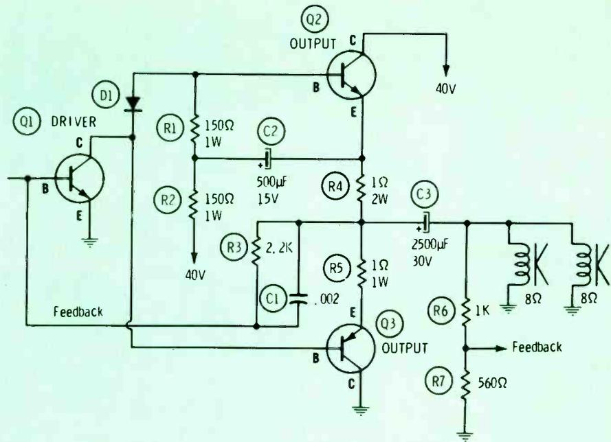
**Fig. 3** Complementary-symmetry output stage draws its name from opposite-polarity transistors, which complement each other and drive speakers push-pull, without a transformer.
