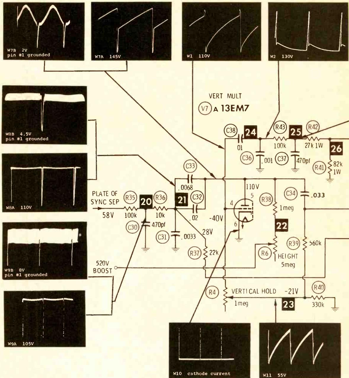
Fig. 2 Schematic of the vertical sweep circuit of the Sears Silvertone 528.51780 b-w television chassis.
