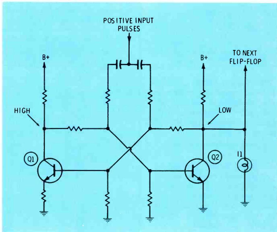
Fig. 1 The basic flip-flop multivibrator.
