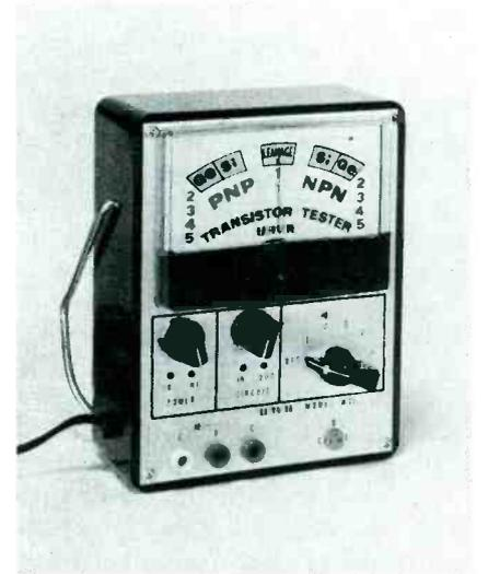
The unit operates on AC, is equipped with a wire-type handle which serves as a tilt stand for easier viewing, measures 6¾ inches x 5¼ inches x 3 inches and weighs 3 pounds.
