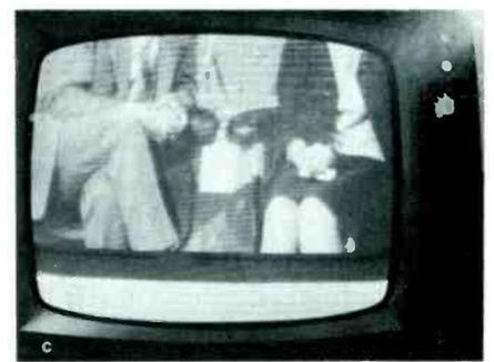
**Fig. 1** Correct locking involves more than just stopping the picture from rolling—both frequency **and** phase must be correct. **A)** Sweep frequency of 30 Hz produces two complete pictures with the vertical blanking bar between them. **B)** Sweep
