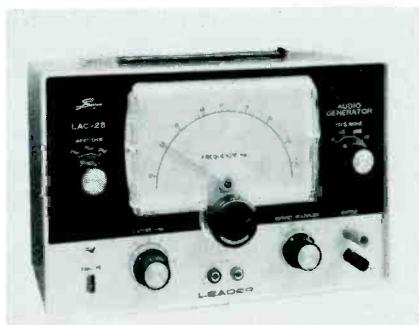
sine wave and a fast-rise square wave. Calibration accuracy is  $\pm 3$  percent ( $+2$ Hz) and is direct-reading, with a rated drift of less than 1 percent ( $\pm 5$  percent change in line voltage).
