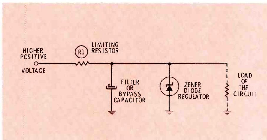
Fig. 5 Schematic of a typical power supply regulated by a zener diode. R1 limits the maximum current which can be drawn by the zener. The voltage across the load is regulated against input voltage changes or changes of the load current.
