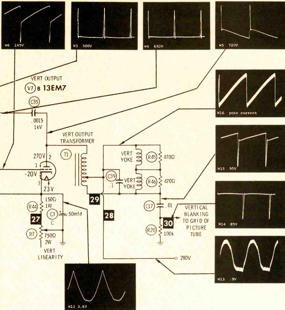
every second, from no height to a raster of about half the size of the 23-inch screen. Experience has taught me that this condition is often the result of excessive resistance from the cathode of the vertical output tube to ground.
