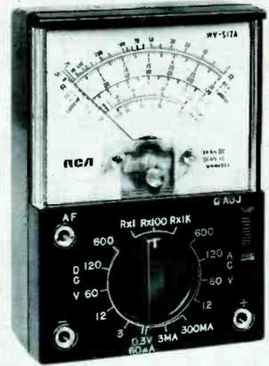
from 0.2 to 600 volts, in four ranges; DC current from one micro-ampere to 300 milliamperes, in three ranges; and resistance from one ohm to five megohms, in three ranges; and decibels from -20 to +37.
