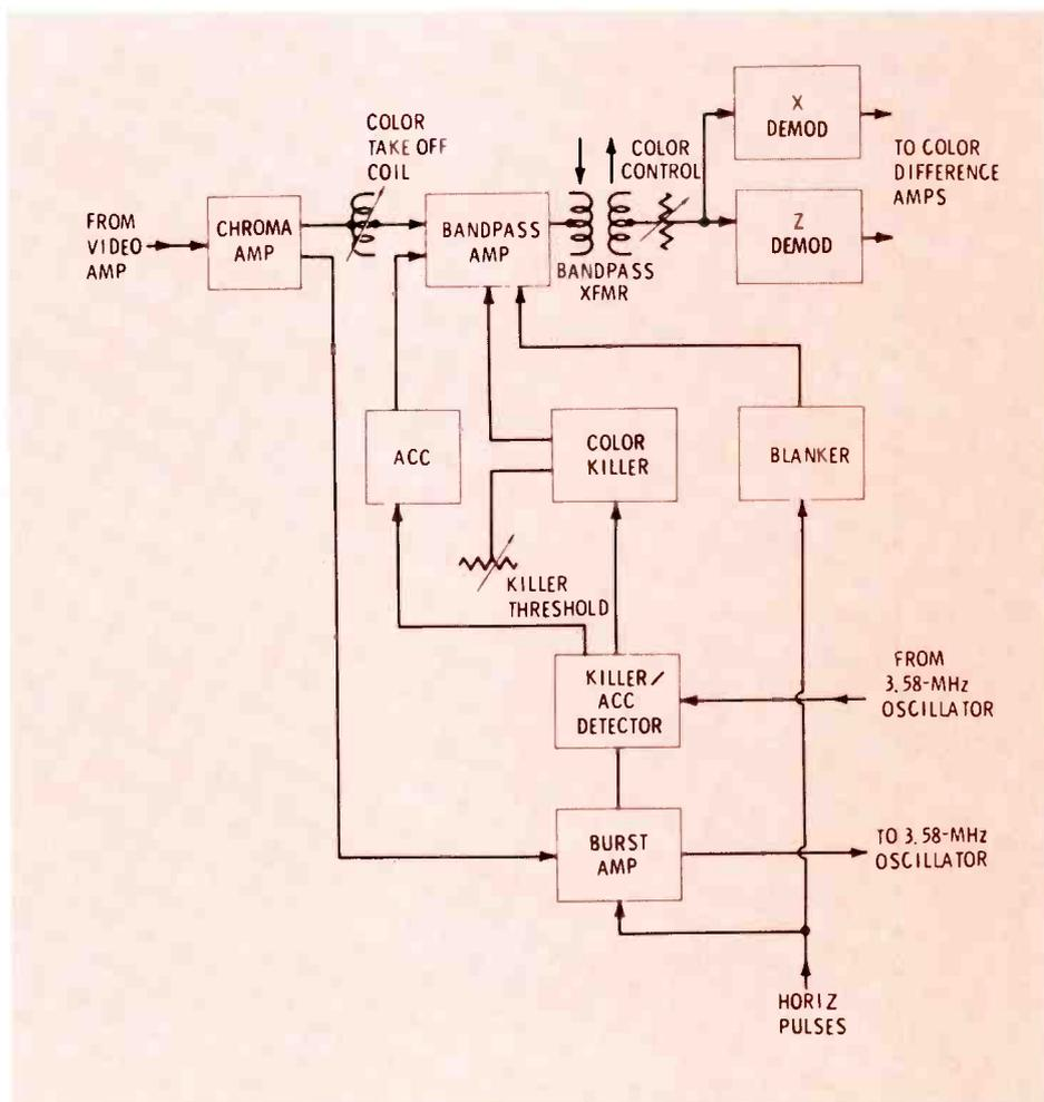
Fig. 1 This is the most common arrangement of stages in a chroma section. Some chassis might have a few more stages, like two bandpass amplifiers. The stage names might sound different: color IF, chroma amplifier, etc. But you'll find the relationships are remarkably the same regardless of who designed or who built the set.
