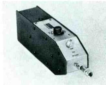
in conjunction with any VHF field-strength meter for the measurement of return loss, or VSWR, as well as the response, gain or loss of amplifiers, filters, cables and other CATV and MATV equipment, according to the manufacturer. It can also be employed to check the flatness of field-strength meters and make noise-figure measurements.
