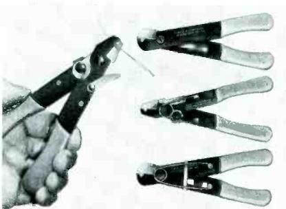
spring-equipped, self-opening handles. A slip ring holds the handles closed when not in use.
