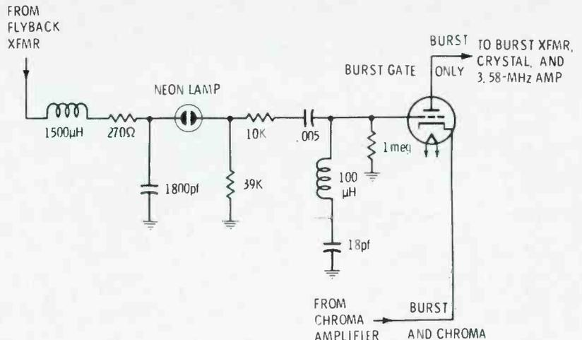
Fig. 4 Burst-gate stage in GE chassis has neon lamp input clipper. If the lamp doesn't fire, burst doesn't get through the triode. Without burst applied to the color-subcarrier amplifier, the demodulators can't produce color.
