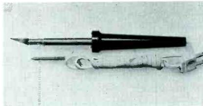
and epoxies, strip insulation from wires, carve foam plastics, and cut and seal ends of plastic rope and woven plastics, according to the manufacturer. With chuck removed, the soldering tip, which is also supplied, may be screwed in.
