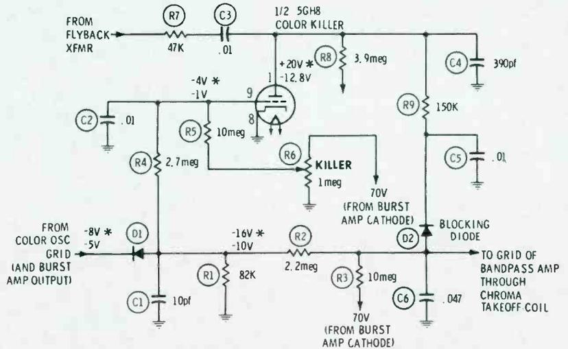
Fig. 3 The automatic color control (ACC) line is short and simple. It includes D1, R1, C1, R2, R3 (which brings in a "bucking" voltage), and C6. The color-killer stage is isolated from the ACC line by diode D2 whenever a burst signal is present and the plate voltage of the tube is positive.
