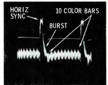
Fig. 2 When counting bars in a waveform, always omit the burst. The third color bar (red), therefore, is the fourth one to the right of sync.
