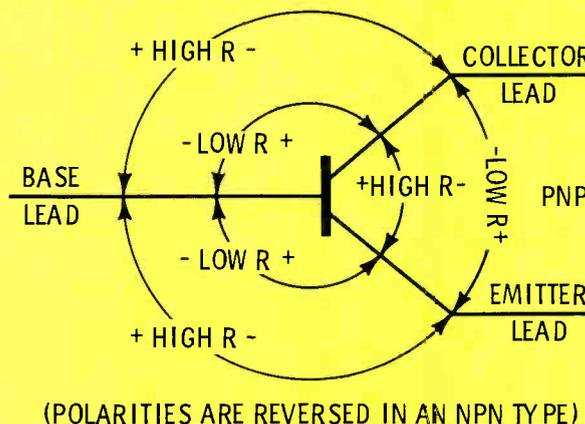
Fig. 3 Comparative ohmmeter readings for high-power PNP and NPN transistors.
