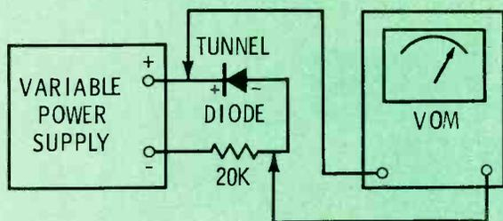
**Fig. 9** Testing tunnel diode for switching action.
