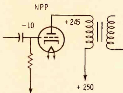
Fig. 3A Any tube could be called an NPP type since both grid and plate will pass current if they are positive in relation to the cathode. In practice, a tube is operated with a reverse-biased grid and forward-biased plate.
