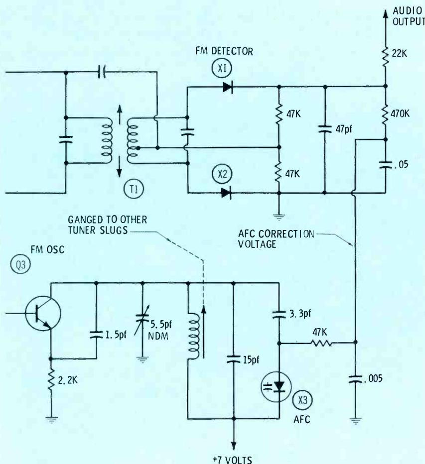
Fig. 1 A DC correction voltage from the FM detector changes the capacitance of X3, the AFC varactor, to compensate for drift or shift of receiver tuning. Circuitry shown here is employed in the Bendix Model 9FBM FM stereo auto receiver.
