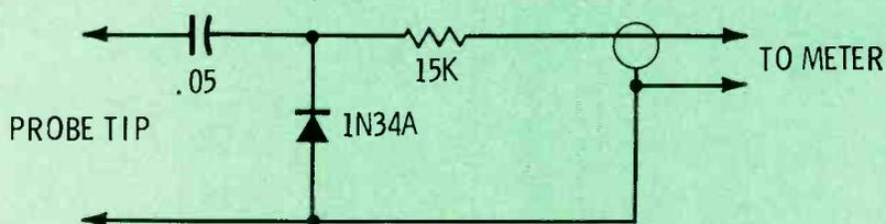
**Fig. 10** Half-wave signal-tracing probe for VOM. Use a low voltage range on the meter.
