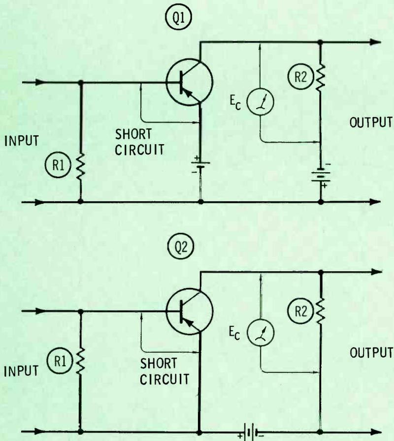
Fig. 5 Basic control-action, or turn-off, test. Voltmeter reading should decrease when base is shorted to emitter.
