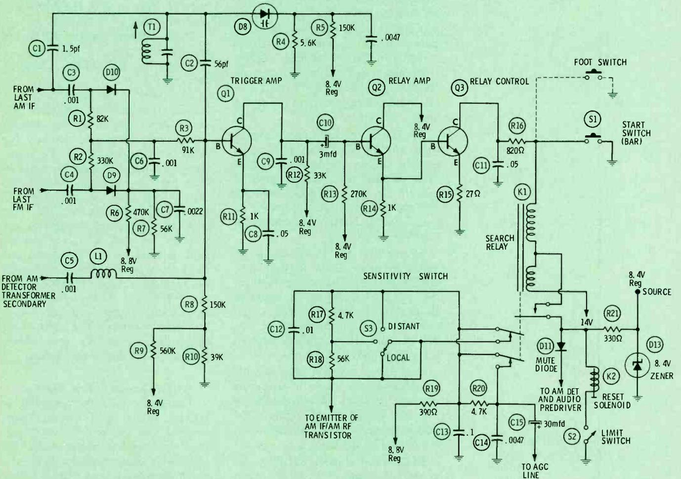
**Fig. 1** Simplified diagram of signal-seeker portion of a Delco AM/FM Wonder Bar auto radio. The relay control stage holds the search relay energized until a station turns on the trigger amplifier and stops the other stages from conducting.
