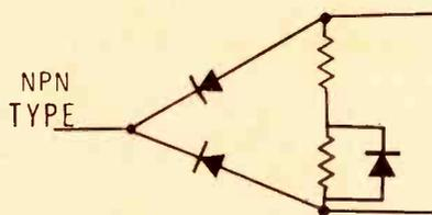
Fig. 2A This is the equivalent of a transistor when it is measured by an ohmmeter.
