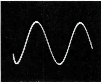
Fig. 6 Waveforms you see if you scope a normally functioning color oscillator.
