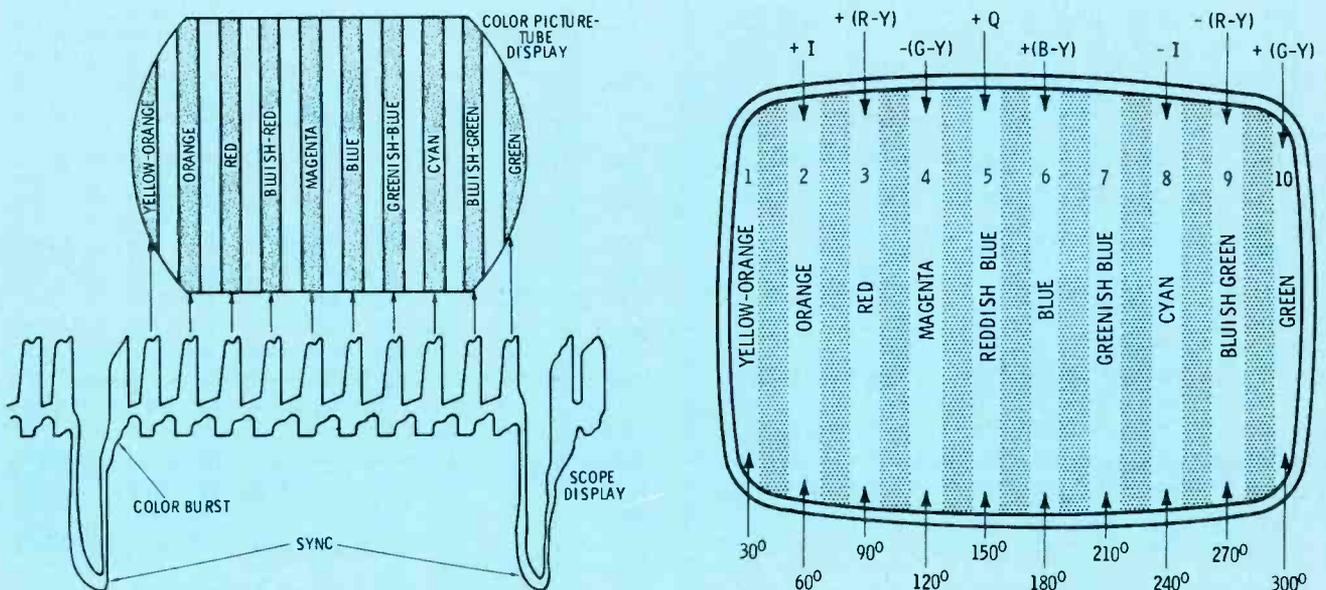
Fig. 1 Color-bar generator of keyed-rainbow type produces the series of bars shown here. The burst bar can't be seen on the screen because it is too far to the left side.
