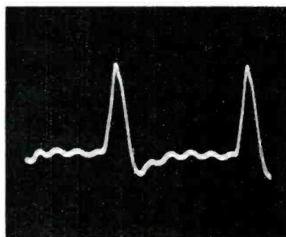
(A) Flyback pulse turns on the burst amplifier.
