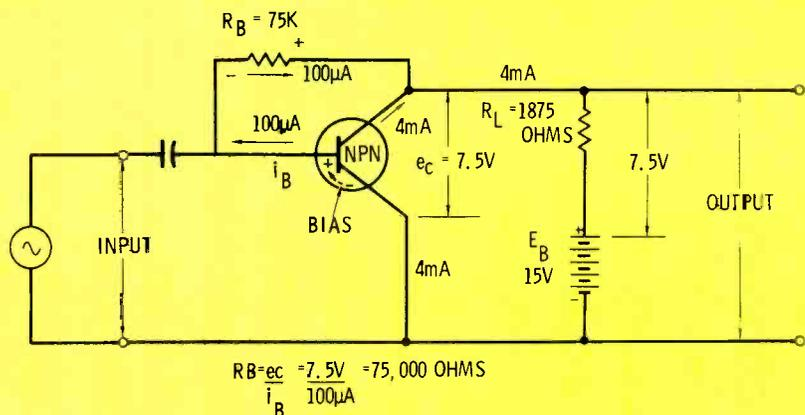
**Fig. 6** Limited control-action test can be made. Voltmeter reading should double when  $R_B$  is bridged with another 75K resistor.
