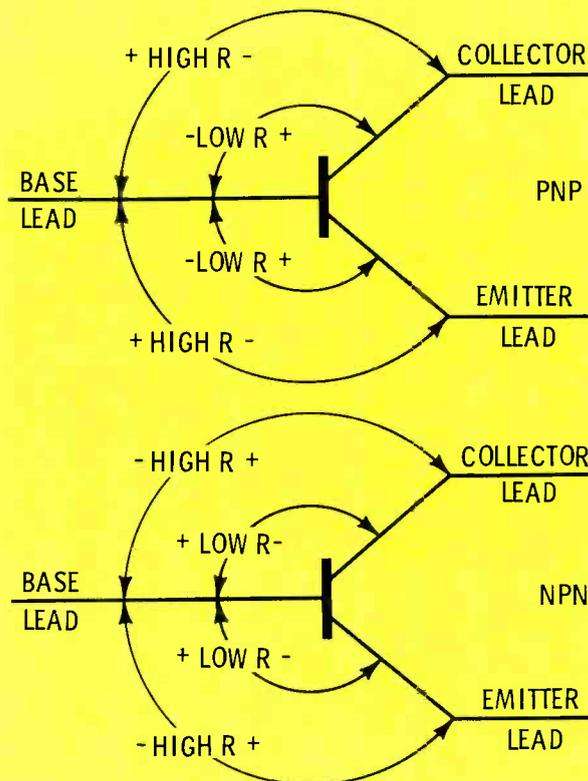
Fig. 1 Comparative ohmmeter readings for low-power PNP and NPN transistors.
