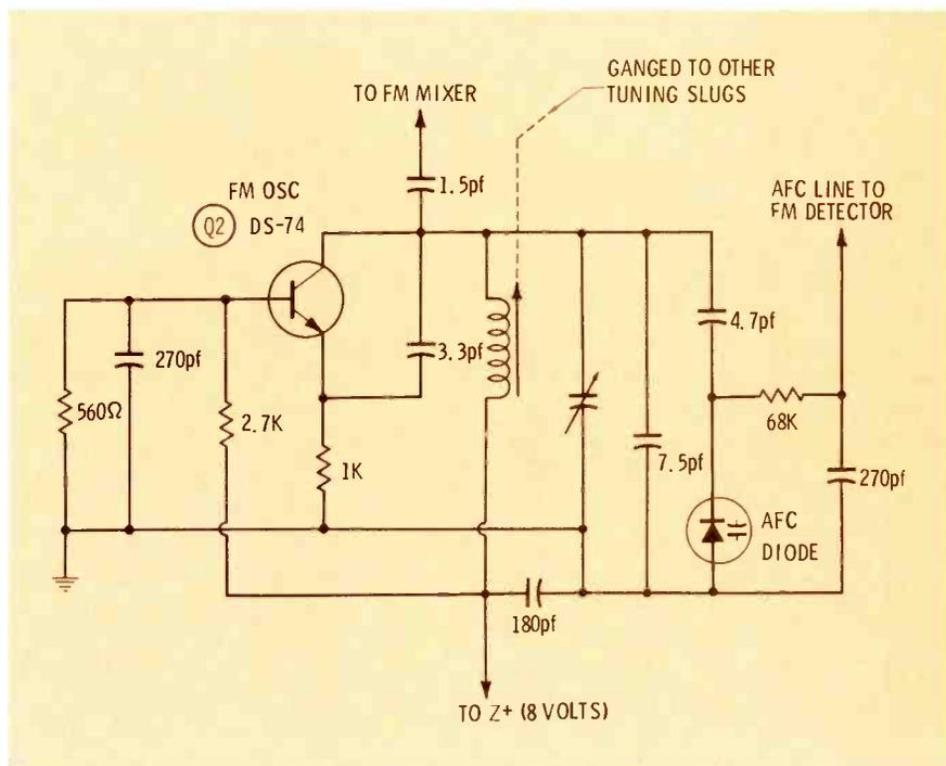
**Fig. 3** Capacitance of FM oscillator transistor is part of the total capacitance of the oscillator tank circuit. Substituting it with the incorrect type will shift the natural frequency of the oscillator enough to prevent reception. Circuit here is employed in Delco Model 7303153 AM/FM auto radio.
