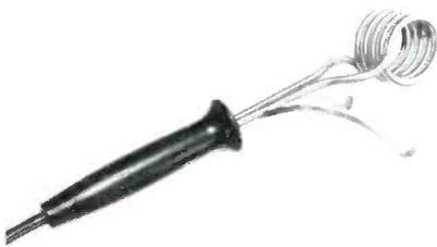
The Heat Tunnel is portable, weighs less than 1 lb., and reportedly shrinks tubing and insulation to 50 % of its original diameter in 5 to 7 seconds.
