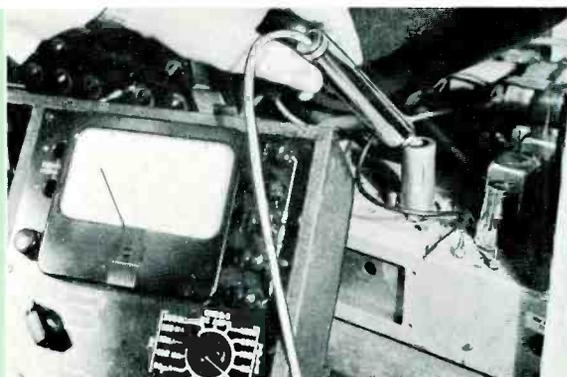
**Fig. 11** Checking local-oscillator operation.
