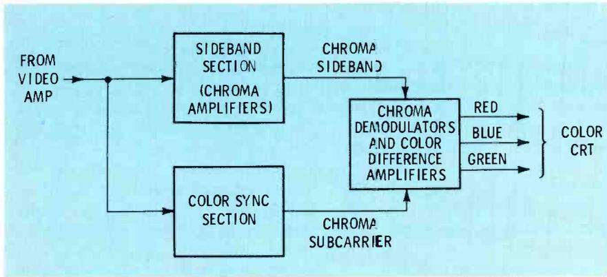
Fig. 3 Color circuitry of color receiver is comprised of three subsections, as shown here.
