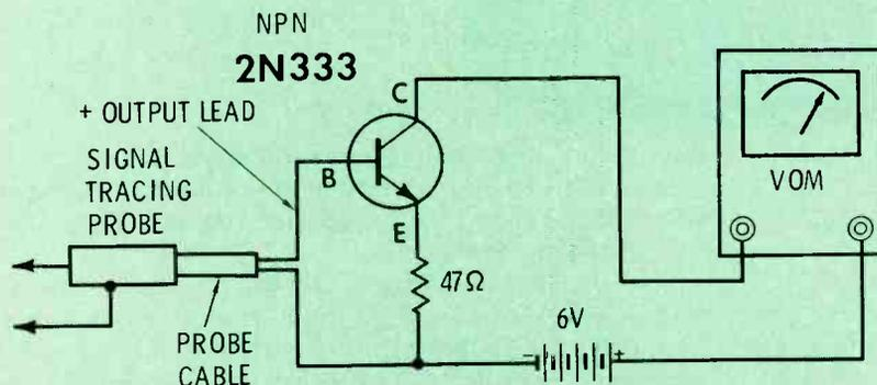
**Fig. 12** Transistor probe amplifier. Use a low DC current scale on the meter.
