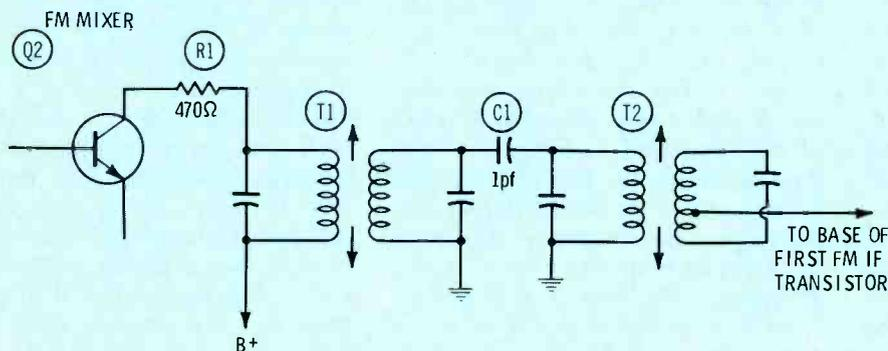
Fig. 2 Open C1 in the quadruple-tuned, two-transformer IF circuit shown here will cause a wide shift in the tuning of the receiver. Circuit shown here is used in Bendix Model 9FBM.
