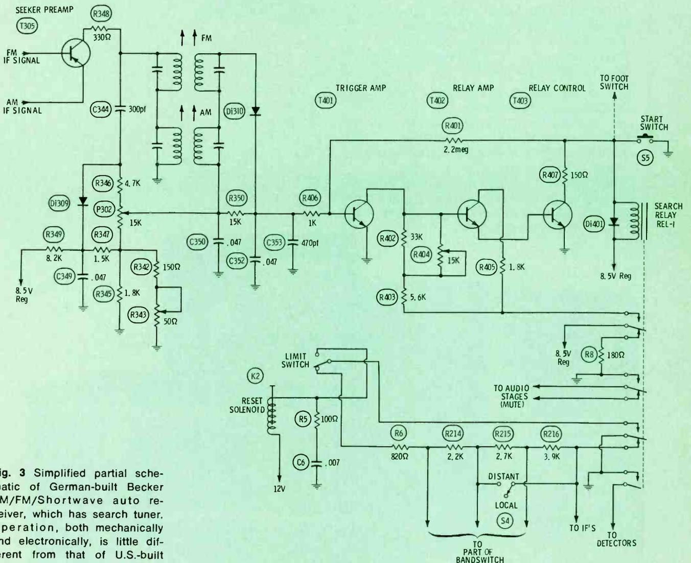
**Fig. 3** Simplified partial schematic of German-built Becker AM/FM/Shortwave auto receiver, which has search tuner. Operation, both mechanically and electronically, is little different from that of U.S.-built signal seeker units.
