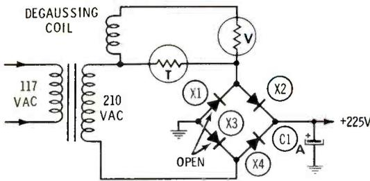
**Symptom**—poor purity that can be cured by external degaussing
