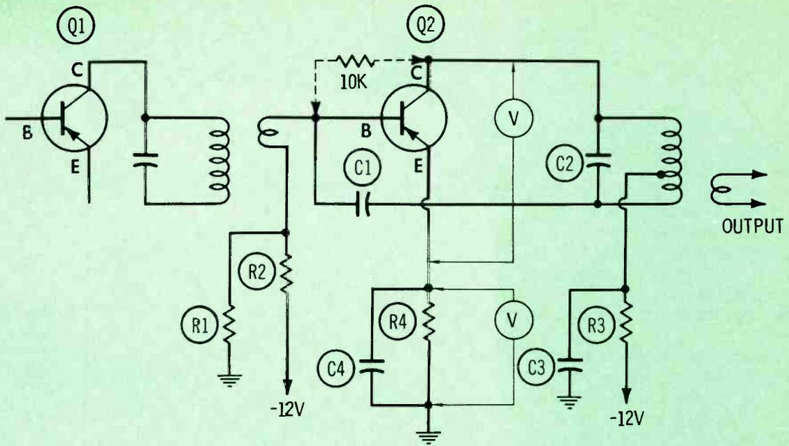
Fig. 4 In-circuit test with a 10K bias resistor. Voltmeter reading should decrease when transistor is turned on.
