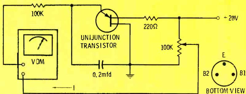
**Fig. 7** Unijunction transistor test circuit.
