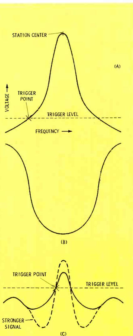
Fig. 2 Graph of rise and fall of DC voltage at base of trigger transistor as tuner scans through station signal. (A) Main signal. (B) Signal for gain control. (C) Resultant trigger voltage.
