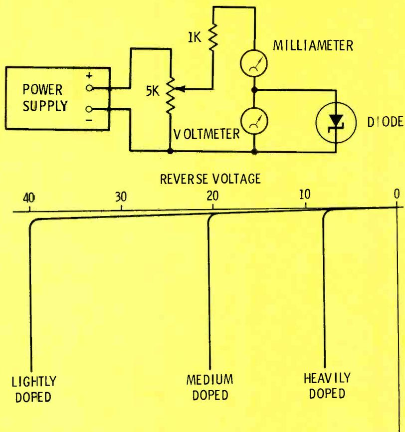
**Fig. 8** Checking a zener diode. Voltage should level off and current increase when 5K potentiometer is increased after zener action has been attained. A) Test setup. B) Zener voltage depends on concentration of doping.
