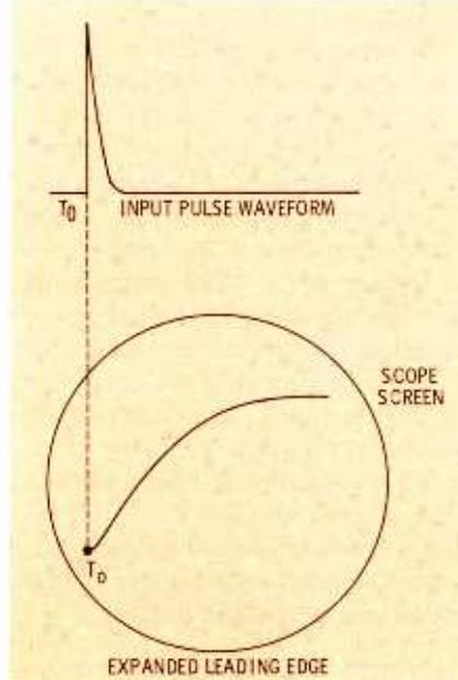
**Fig. 6. Sweep must start at the beginning of the pulse.**
