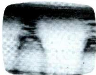
**Fig. 9. Thin horizontal line streaking in transistorized AGC circuits is produced by noisy junction in transistor or AGC diode.**
