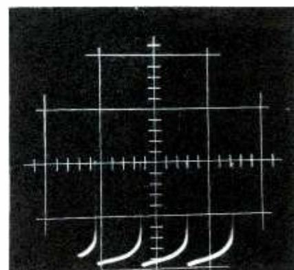
Fig. 5. Normal vertical-output pulses.
