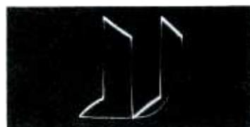
(B) 60Hz square-wave with excessive tilt.
