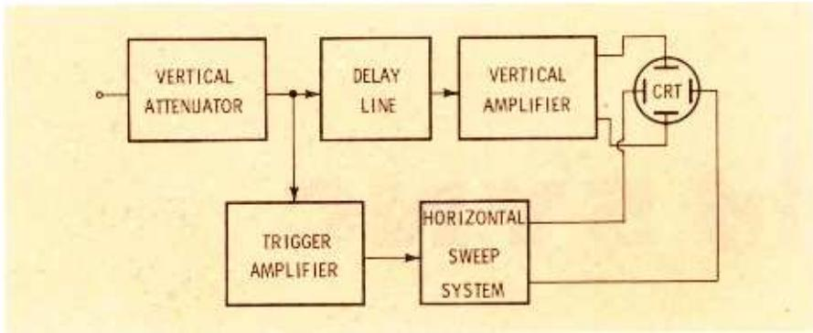
Fig. 7. Delay line permits early triggering of sweep.
