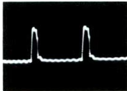
Fig. 10B. The keying pulse in transistor receivers contains noise, ringing, etc.
