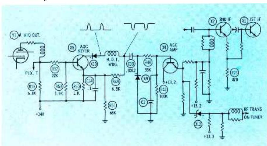
Fig. 7. Philco 16JT26 intermixes tubes and transistors but keyed AGC circuits uses transistors. Shop Talk Editor thinks three circuits are typical of future designs.
