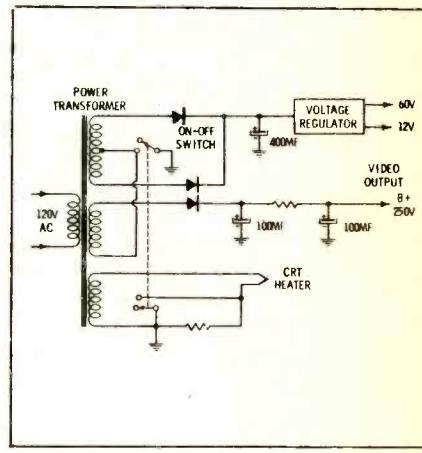
vertical output, horizontal driver, and horizontal output stages; and a regulated 12 volts for the remainder of the circuitry—with the exception of the video output.
