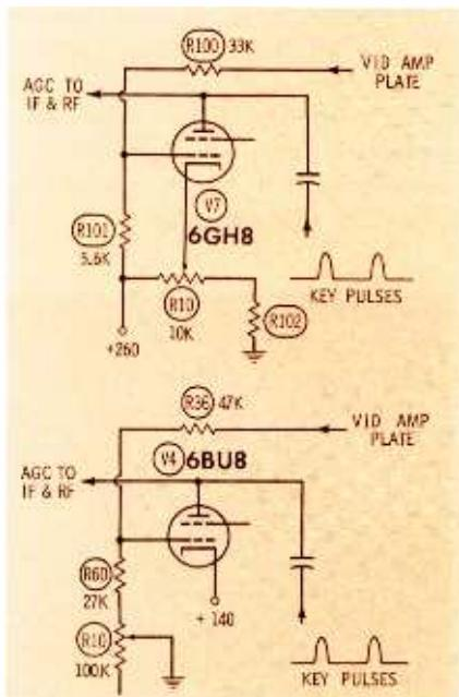
Fig. 1. Sensitivity of keyed AGC stage is controlled by either of these circuits in many designs.
