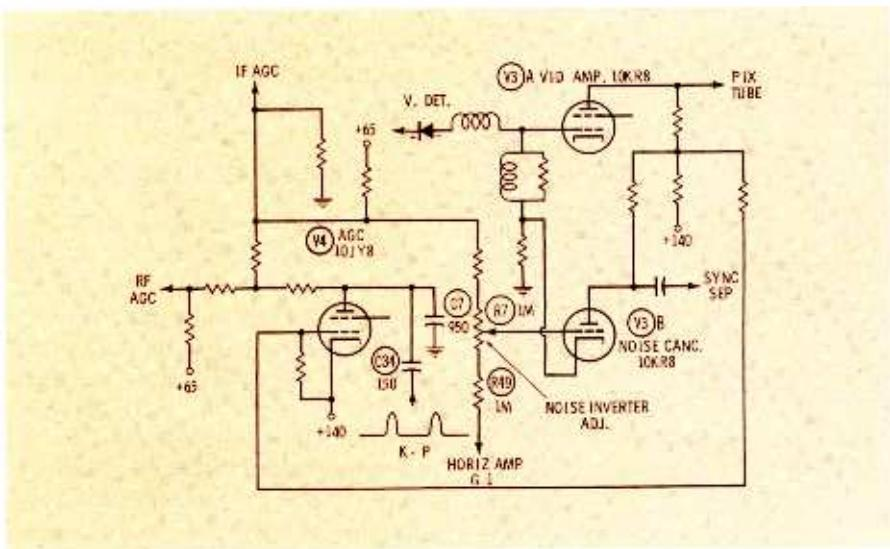
Fig. 3. Decreasing capacity of C-7 to 820 pf cured trouble in Philco.
