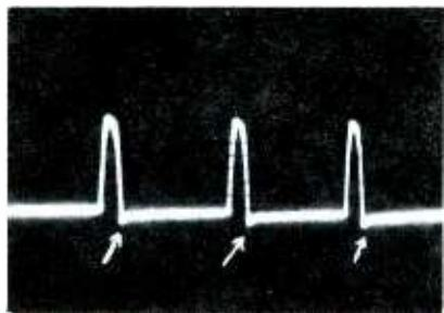
**Fig. 8. Most AGC keying pulses have reverse overshoot following pulses.**
