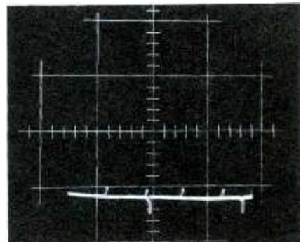
Fig. 4. Vertical oscillator out of sync.
