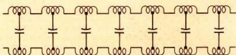
Fig. 8. Basic delay-line circuit.
