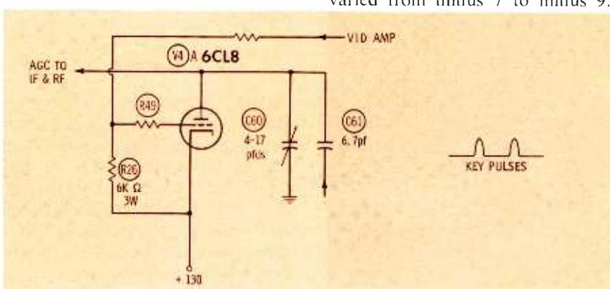
Fig. 2. Westinghouse controls levels of AGC voltage developed by varying amplitude of keying pulses via variable capacitor C-60.
