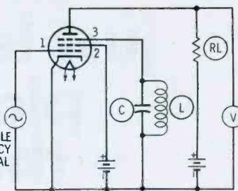
Fig. 2. Gated-beam frequency sensor.
