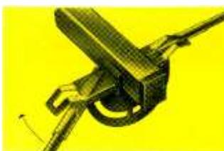
The wedge-snap lock actually tightens and improves with vibration. The spring pressure of the clamp jams the wedge aperture over the squared dipole's end. Since it cannot seat all the way down, a sharp pressure is maintained on the edges of
