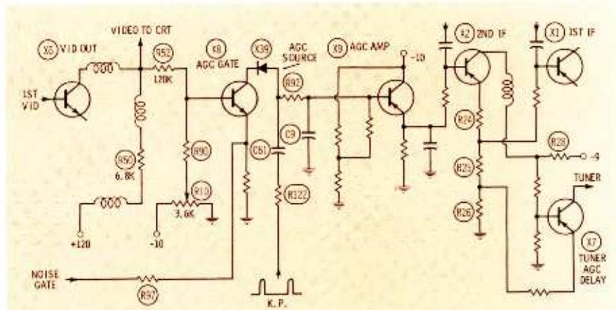
Fig. 5. Late transistorized TV by Zenith uses this keyed AGC circuit with some interesting features.
