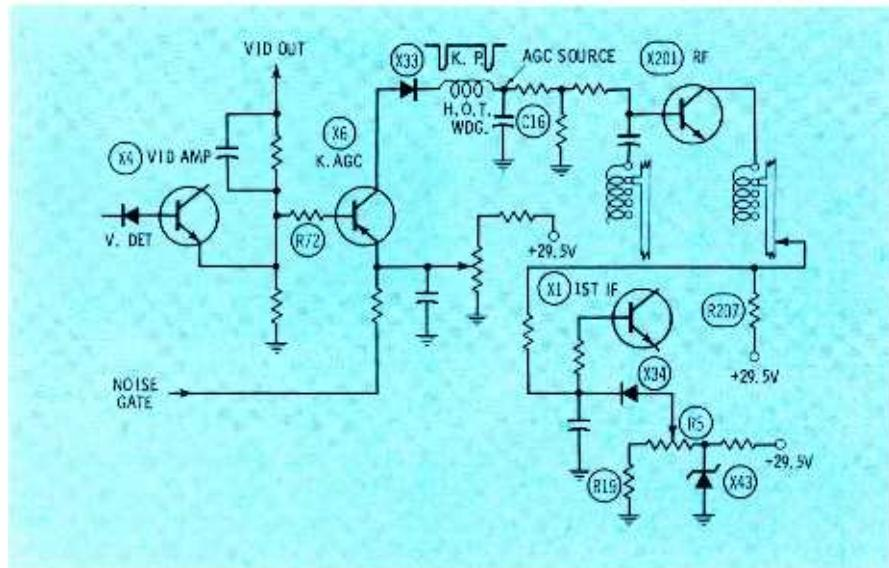
Fig. 6. RCA transistorized TV uses simpler keyed AGC circuit.
