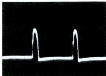
Fig. 10A. Keying pulses in tube circuits are generally clean.
