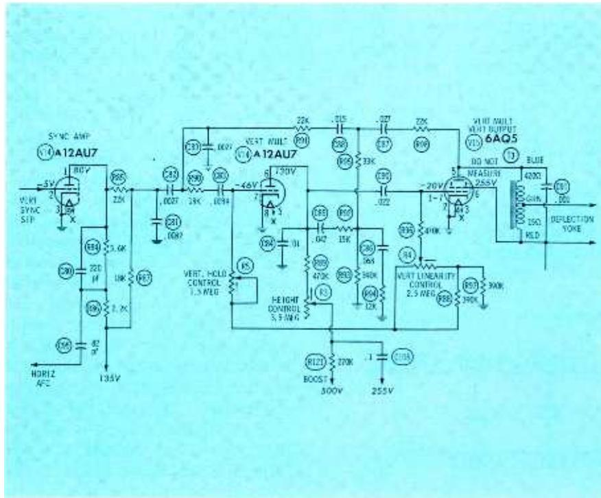
Fig. 1. Vertical section of RCA Chassis KCS84F.
