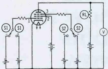
Fig. 1. AND gate using gated-beam tube.
