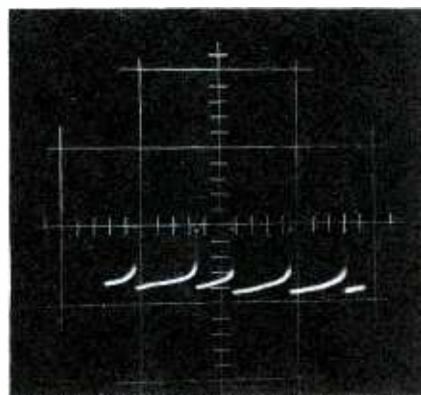
Fig. 3. Abnormal vertical-output pulse.
