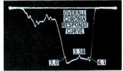
Fig. 2. Generator must be good "sweeper" to align chroma bandpass circuits in color receiver.
