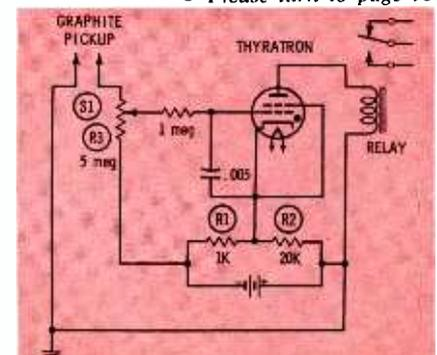
Fig. 5. Graphite-mark sensing circuit used in one type of roll-paper cutting machine.
