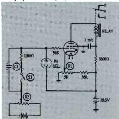
Fig. 3. One of three light-measuring circuits of color printer shown in simplified form.
