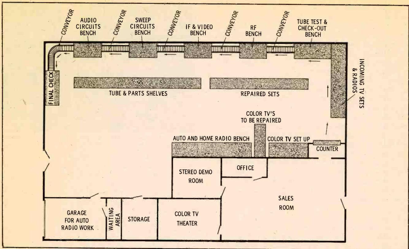
Fig. 11. Floor plan of a TV shop featuring conveyor belts to connect specialist's benches, a separate color TV bench, and a radio bench.
