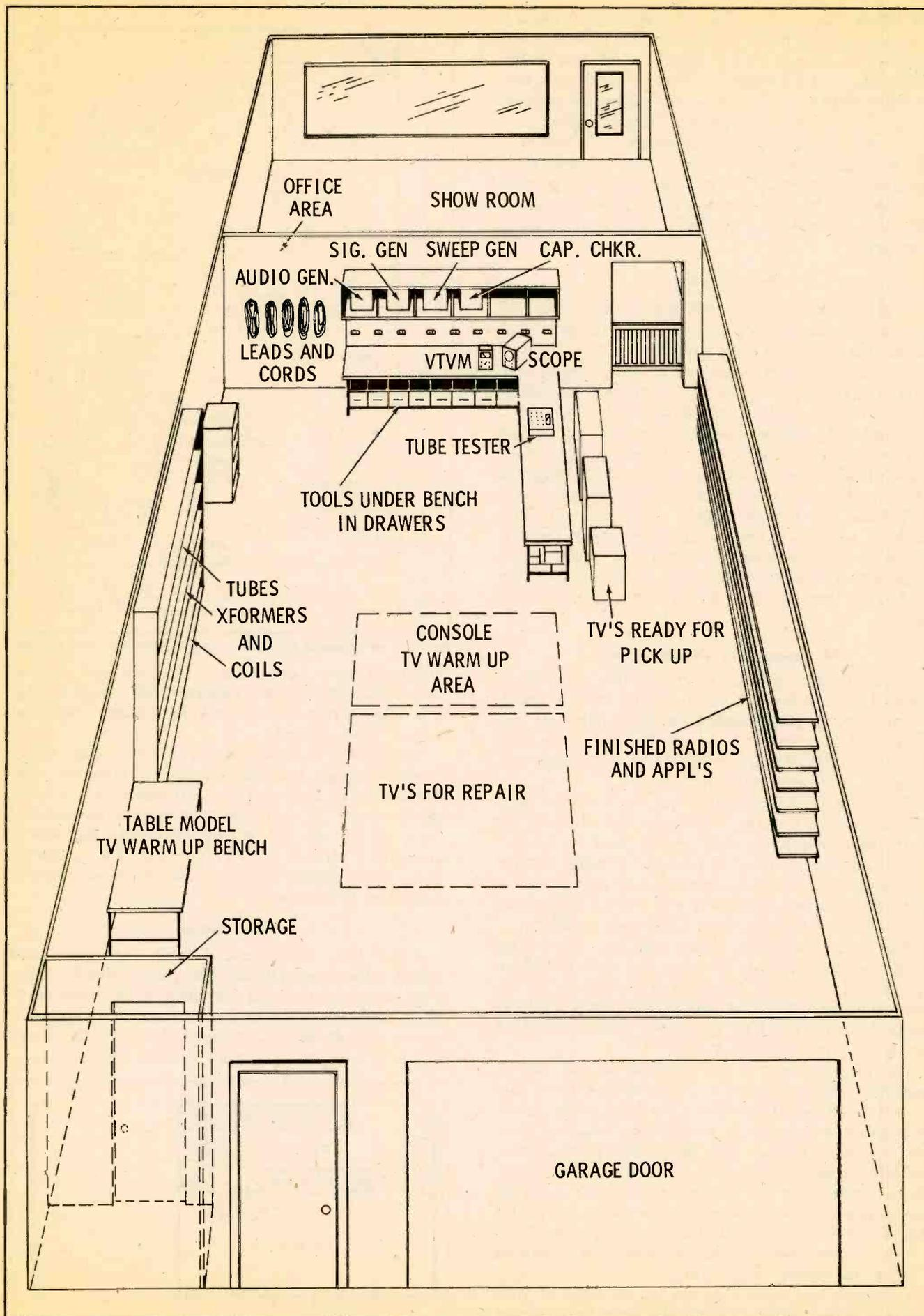
Fig. 5. A compact two-man shop featuring a large, efficient main work bench, an auxiliary bench, and plenty of storage.
