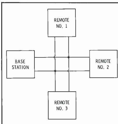
Fig. 4. Intercom connection for several parallel remotes using the same control lines.
