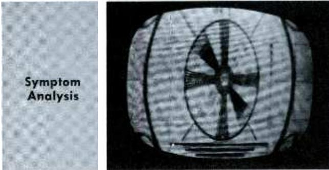
Raster greatly overscans screen at both top and bottom, even with R2 fully counterclockwise. Top can be squeezed down by turning R3 to minimum setting. Picture locks into sync, but tends to roll for several frames whenever signal fades or is interrupted.
