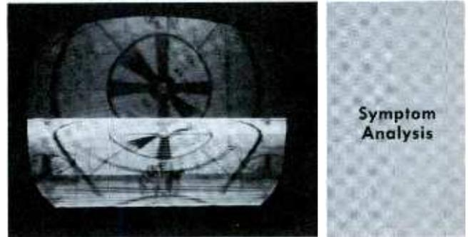
"Reflecting pool" effect, caused by inverted image overlapping bottom half of picture, occurs erratically. When R1 is turned, symptom disappears, but picture tends to stretch at top and fold over at bottom. With no sync signal present, raster is only 2" high.
