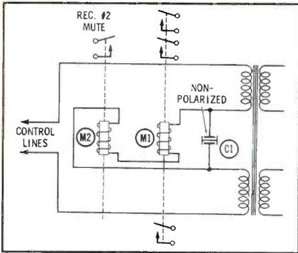
Fig. 5. Series relays allow use of a single wire-pair for multiple control functions. remote is outfitted with a separate console which contains a multifrequency audio oscillator. When a particular tone is generated, the corresponding receiver is the only one in the system that hears the transmission.
