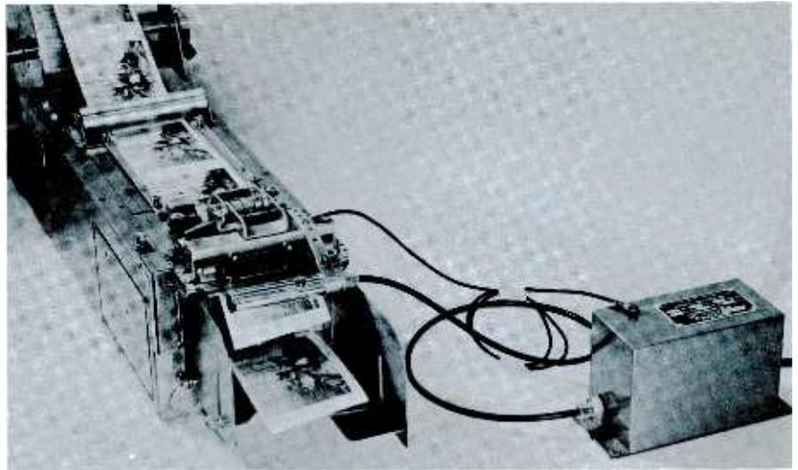
Fig. 4. An automatic roll-paper cutting machine and its associated power supply.
