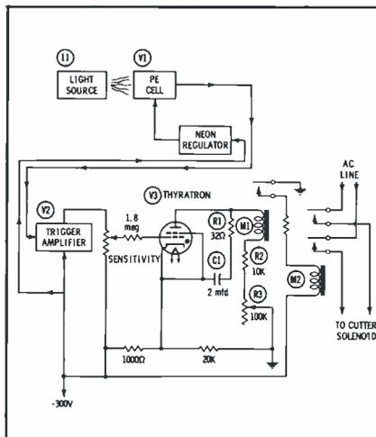
Fig. 6. This light-sensitive mark-detecting scheme uses a photoelectric sensing cell.
