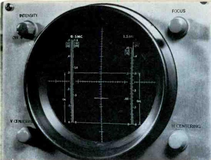
Some scope graticules are marked for direct reading, with a numbered voltage scale; a few have several scales that correspond with settings of the vertical range switch. The graticule shown here has four scales; with the range switch set to the .5-volt setting and the band-switch at 1.5 mc, voltages must be read from the extreme right-hand .5-volt scale.
