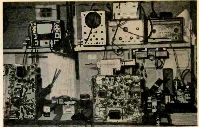
Fig. 9. Test equipment shelves are positioned for ease of equipment operation and the convenience of the TV technician.
