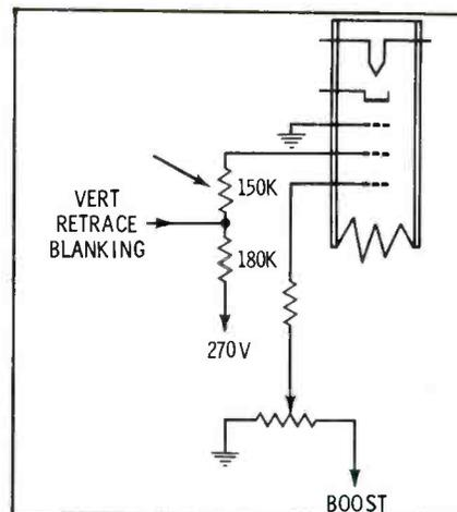
Fig. 4. Loss of accelerating voltage on CRT, due to open resistor, blanks out raster.
