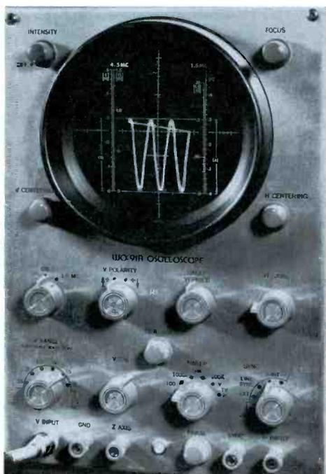
Anyone with the skill to use an ordinary VTVM can easily use his scope as a voltage-measuring instrument. In fact, certain scope functions can be likened to those of a VTVM. For instance, the voltage-range switch of a VTVM can be considered equivalent to the vertical multiplier switch of a scope, since they both determine the "full-scale" range of the voltage indicator. Also, the vertical gain control of a scope is somewhat like the "zero" control of a VTVM.
