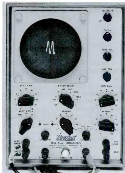
Another type of scope has a 1-volt peak to peak calibration terminal on the front panel. The vertical test lead, or a jumper, will apply the signal from this terminal to the vertical input, and you can adjust the vertical gain to obtain a trace of some arbitrary height—say one inch. Then with the same control settings, any signal corresponding to this same height is equal to 1 volt. The multiplier switch permits measuring larger voltages—as you'll see.
