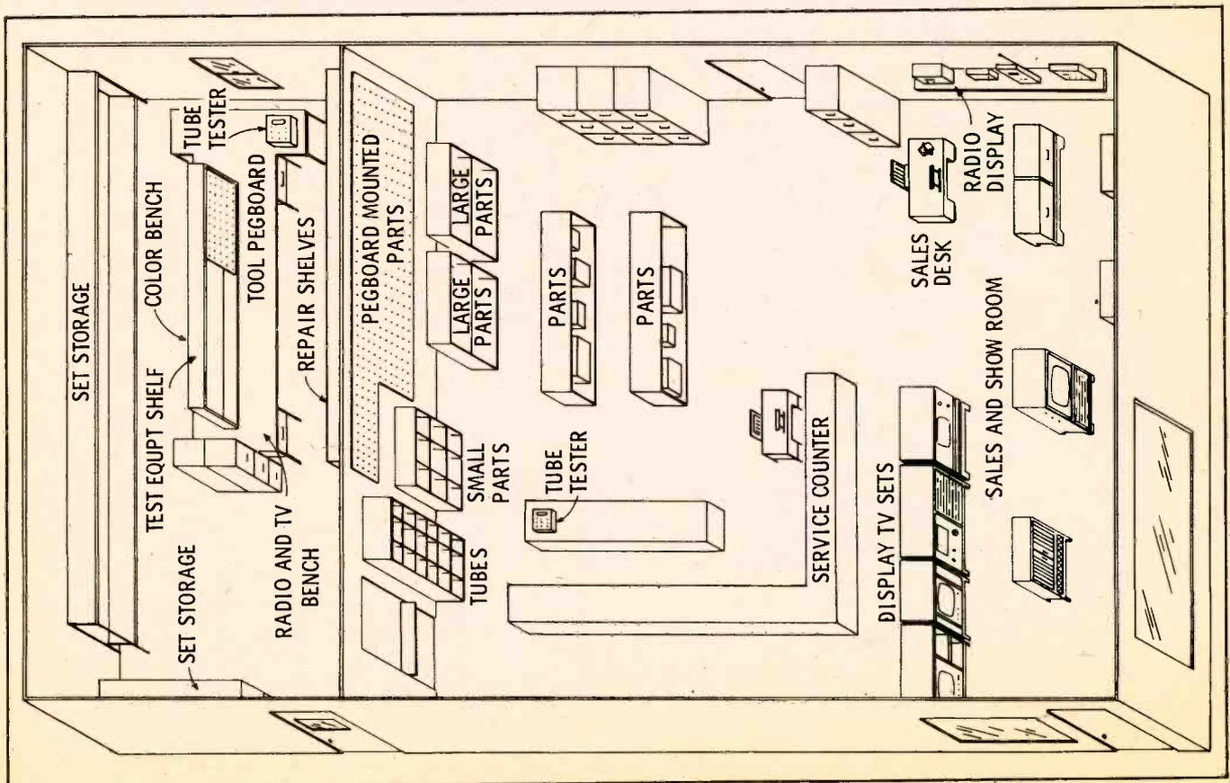
Fig. 6. This floor plan shows a shop with an isolated service area. The sales and business areas are completely separate.
