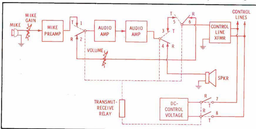
Fig. 2. Relay contacts control operation of remote console and radio equipment.
