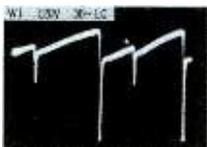
Amplitude of W1 and W5 decreases by amount proportional to loss of height in raster. When R1 is turned to make sync pulses visible in W1, they are seen to have several times normal amplitude; this explains why raster splits in two, and gives hint of trouble in screen circuit. W6 includes full-strength sync signal, but pulses fed back from V1 are much weaker than normal.
