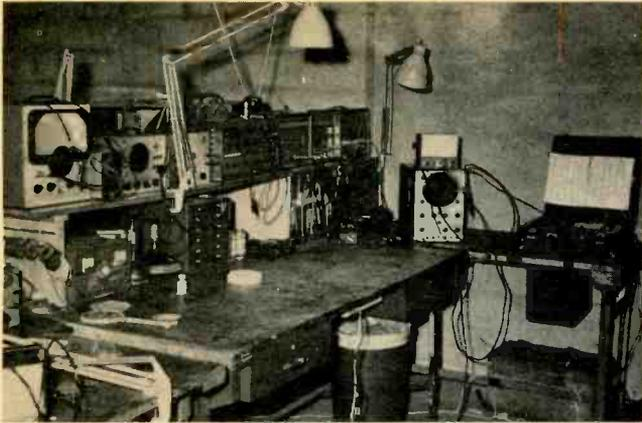
Fig. 7. Compartments keep test equipment up off the bench, thus providing a larger, cleaner working area for the technician.
