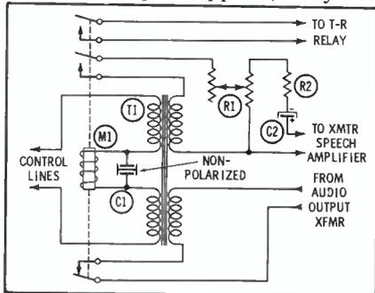
Fig. 3. The system control lines are terminated in a coupling and isolating transformer.
