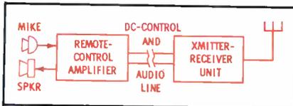
Fig. 1. The two-way radio is remotely controlled by the use of a special amplifier.
