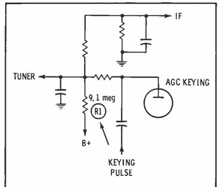
Fig. 3. AGC delay resistor frequently causes intermittent trouble by changing value.
