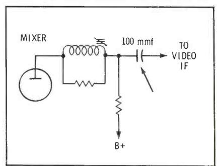
Fig. 1. Leakage in grid capacitor reduces bias on first IF and causes overloading.
