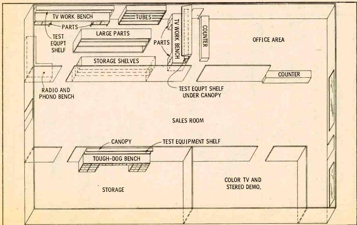
Fig. 8. This shop has two main TV benches, a radio-phono bench, and a separate "tough-dog" bench located in another room.
