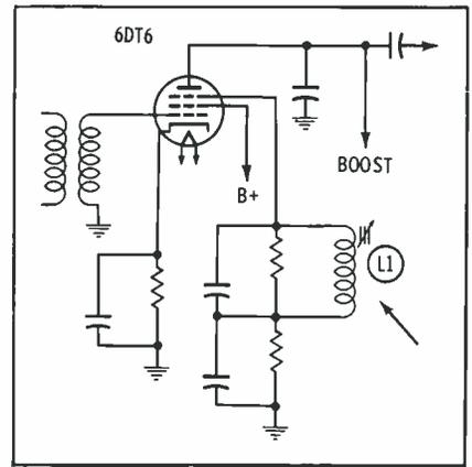
Fig. 2. Major suspect in many cases of intermittent sound trouble is the quadrature coil.
