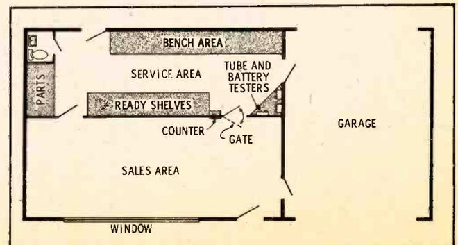
Fig. 4. A one or two man shop complete with drive-in facilities.
