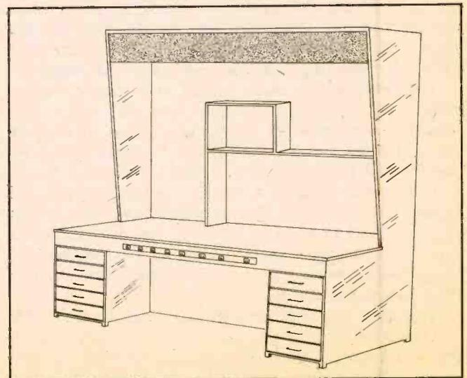
Fig. 10. Construction details of canopy type test bench showing location of test equipment shelves, drawers, and AC outlets.
